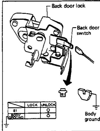
Back door unlock switch & key cylinder tamper switch (Fig 8)
