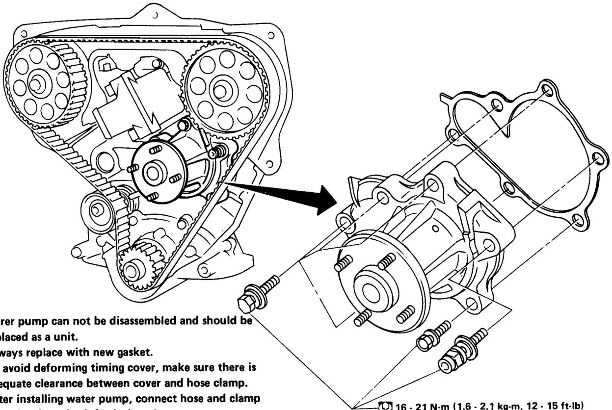
Water pump can not be disassembled and should be replaced as a unit.
