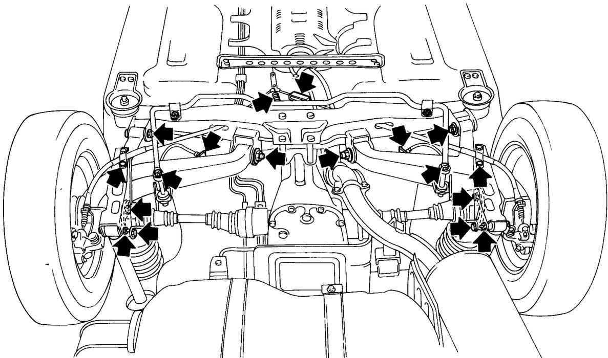
← : Removing and installing points
