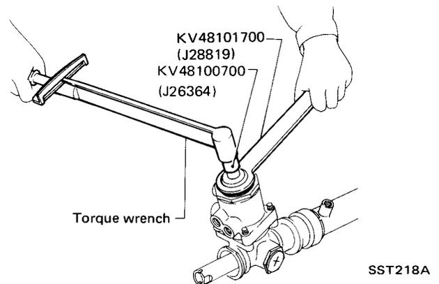
Pinion starting torque  $T_1$  :
