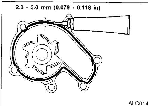
2. Apply a continuous bead of liquid gasket to mating surface of water pump and water pump cover (cylinder block side).
