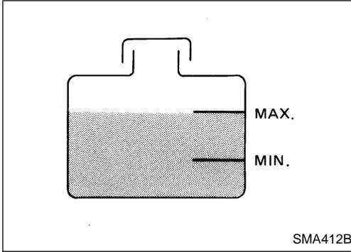
12. Refill reservoir tank to MAX level line.
