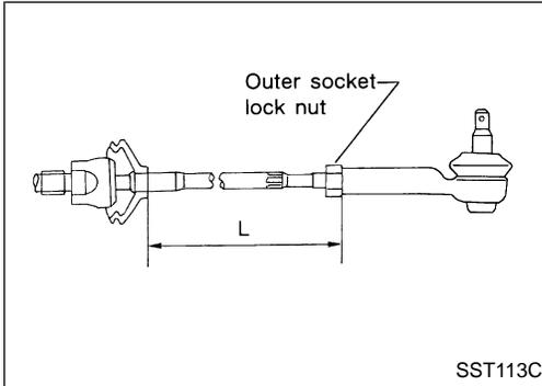
2. Tighten outer socket lock nut to specified torque.
