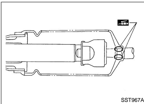
4. Before installing boot, coat the contact surfaces between boot and tie-rod with grease.
