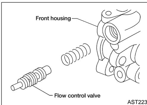
3. Remove connector and flow control valve with spring.
