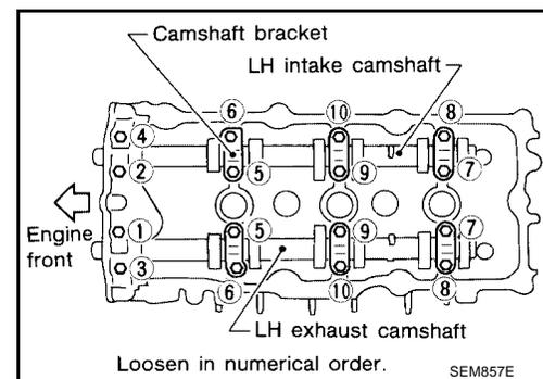
11. Remove the RH and LH cylinder head bolts, with power tool.
