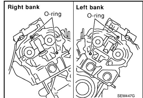
2. Apply Genuine Silicone RTV Sealant or equivalent, to the rear timing chain case. Refer to [EM-159, "POSITION FOR APPLYING LIQUID GASKET"](#).
