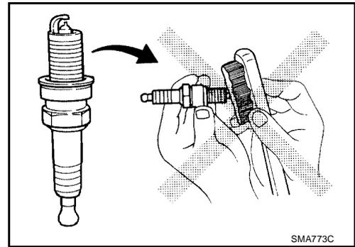
If plug is covered with carbon, a spark plug cleaner may be used.
