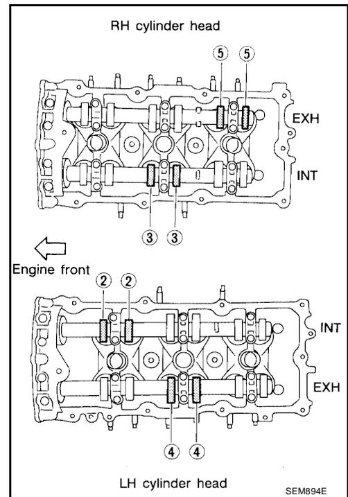
10. Turn the crankshaft 240° and align as above.
