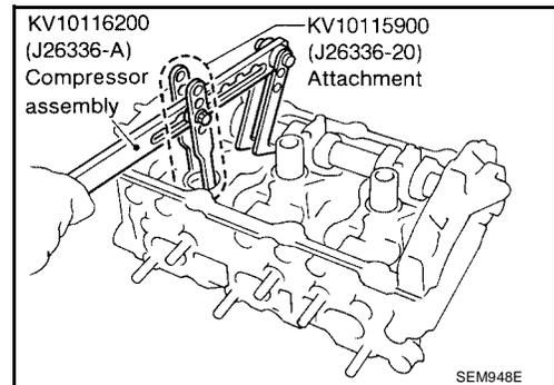
5. Remove valve oil seal with Tool.
