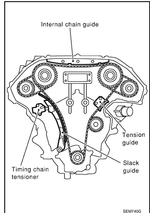
39. Remove the timing chain tensioner and slack side chain guide.
