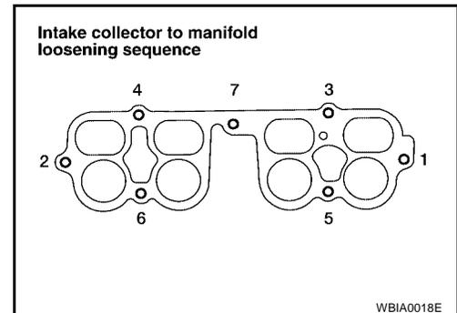
13. Loosen the bolts in the order shown to remove the intake manifold assembly, using power tools.
