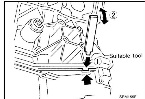
19. Remove the O-ring seals from the bottom of the cylinder block and oil pump housing, use new O-rings for installation.
