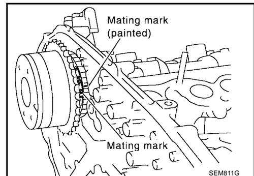
7. After confirming the mating marks are aligned, tighten the camshaft sprocket mounting bolts.
