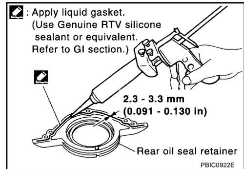
3. Install rear oil seal retainer to cylinder block.
