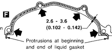
\*1: Apply liquid gasket to the chamfered surface between camshaft bracket and cylinder head.
