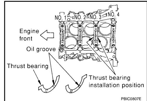
5. Set the upper main bearings in their proper positions on the cylinder block.
