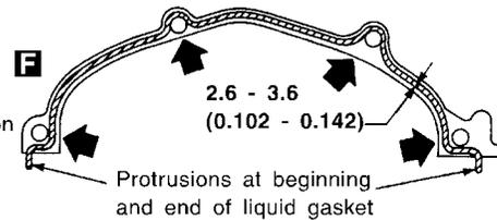
\*1: Apply liquid gasket to the chamfered surface between camshaft bracket and cylinder head.
