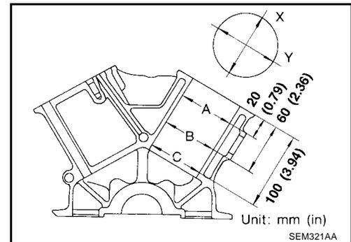
5. Determine piston oversize according to amount of cylinder wear.
