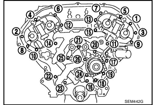
6. Remove rear timing chain case using Tool.
