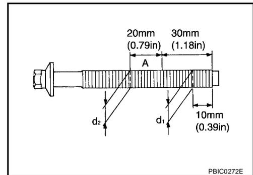
**OUTER DIAMETER OF CONNECTING ROD BOLT**
