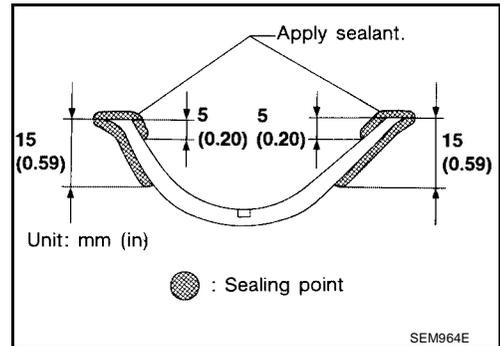
2. Install the front cover gasket and rear oil seal retainer gasket as shown.
