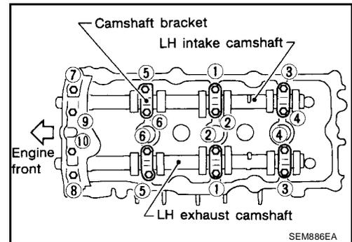
8. Measure difference in levels between front end faces of No. 1 camshaft bracket and cylinder head.
