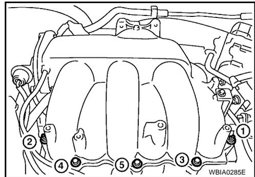
15. Loosen the bolts in the order shown, and remove the intake manifold with power tool.
