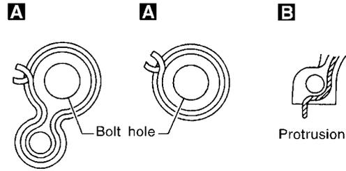
Sealant protrusion away from bolt hole
