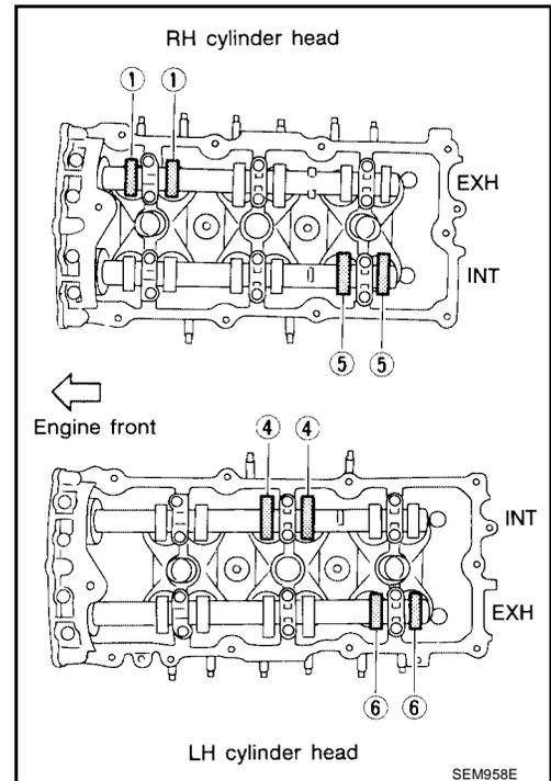
13. If all valve clearances are within specification, install the following components. If the valve clearances are out of specification, adjust the valve clearances.
