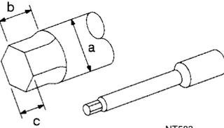
Loosening and tightening cylinder head bolt<br><b>a: 13 (0.51) dia.</b><br><b>b: 12 (0.47)</b><br><b>c: 10 (0.39)</b><br>Unit: mm (in)<br>NT583 |
