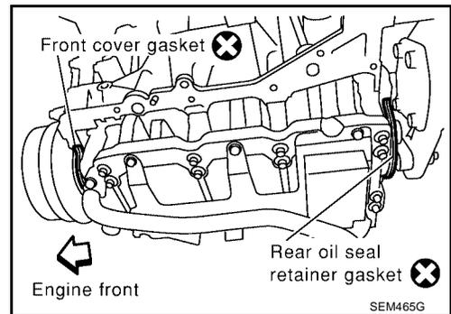
3. Apply a bead of sealant to the cylinder block mating surface of the upper oil pan to a limited portion as shown.
