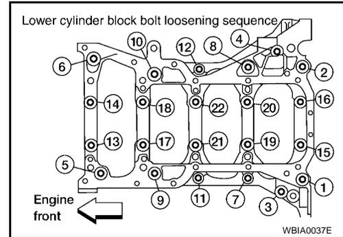
14. Remove the lower cylinder block.
