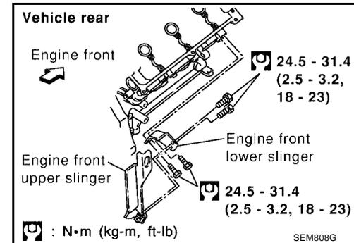
20. For additional safety, secure the engine in position with a hoist.
