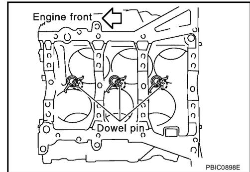
4. Install the main bearings and the thrust bearings.
