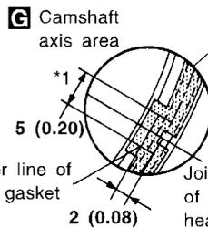
Center line of rear timing chain case sealant groove ← : Run along bolt hole outer side.
