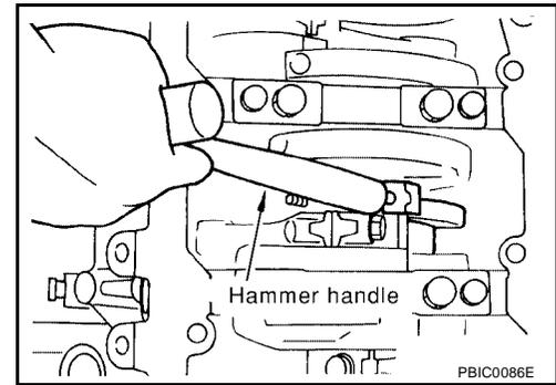
12. Remove the connecting rod bearings.
