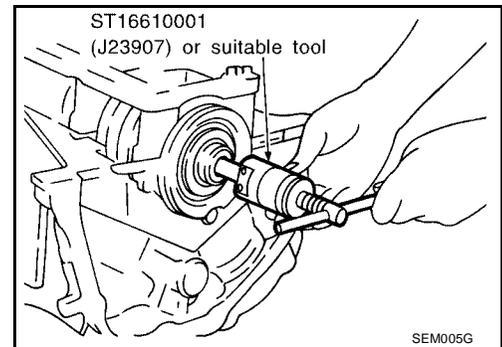
10. Use a seal cutter to cut away liquid gasket and remove rear oil seal retainer. Refer to [EM-111, "REMOVAL OF LIQUID GASKET SEALING"](#) .
