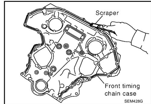
48. Remove all old Silicone RTV Sealant from all the bolt holes and bolts.
