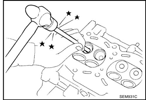
3. Ream cylinder head valve guide hole.
