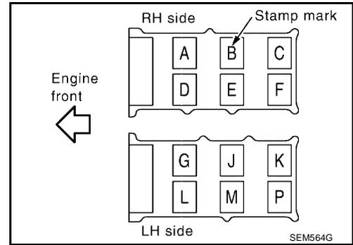
10. Tighten the camshaft brackets in the following five steps in the numerical order shown.
