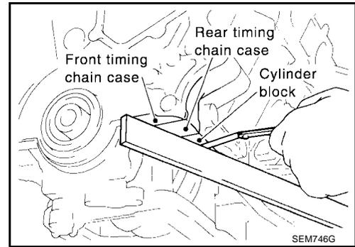
**Front timing chain case to rear timing chain case**
