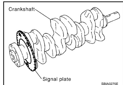
15. Remove the crankshaft.
