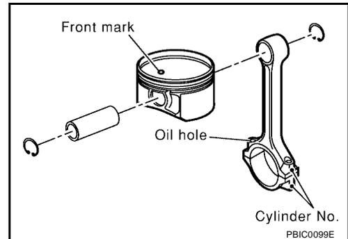
b. Install the piston to the connecting rod.
