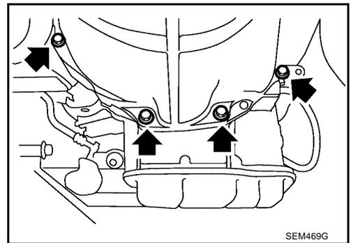
7. Apply a continuous bead of sealant to the lower oil pan.
