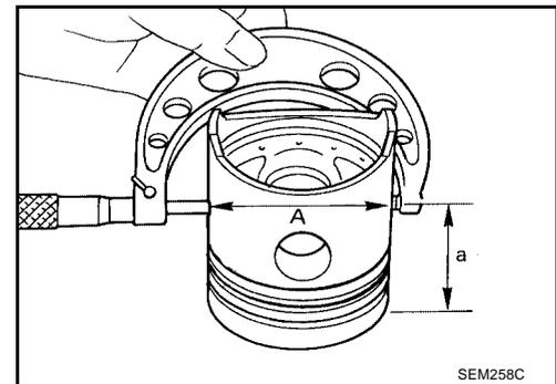
4. Check that piston-to-bore clearance is within specification.
