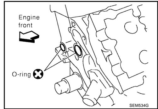
13. Install the new O-rings on the cylinder head.
