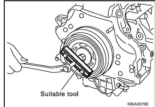
15. Remove the front cover with the following procedure:
