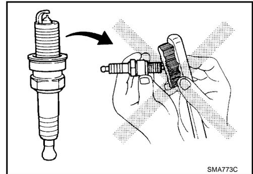
If plug tip is covered with carbon, a spark plug cleaner may be used.
