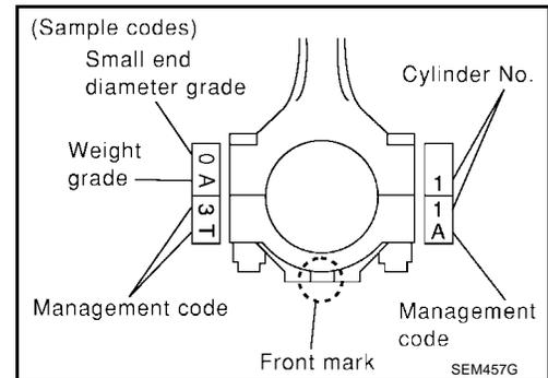
15. Check the connecting rod cap bolts before reusing, then install in their original position in the connecting rod. The bolts should screw in smoothly by hand.
