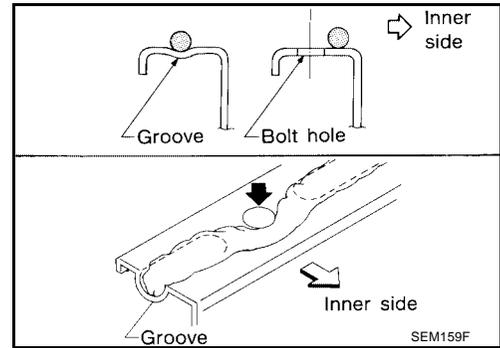
4. Install new O-rings on the cylinder block and oil pump body.
