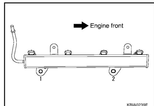
Fuel tube bolt tightening 1st step : 9.3 - 10.8 N·m (0.95 - 1.1 kg-m, 83 - 95 in-lb)
