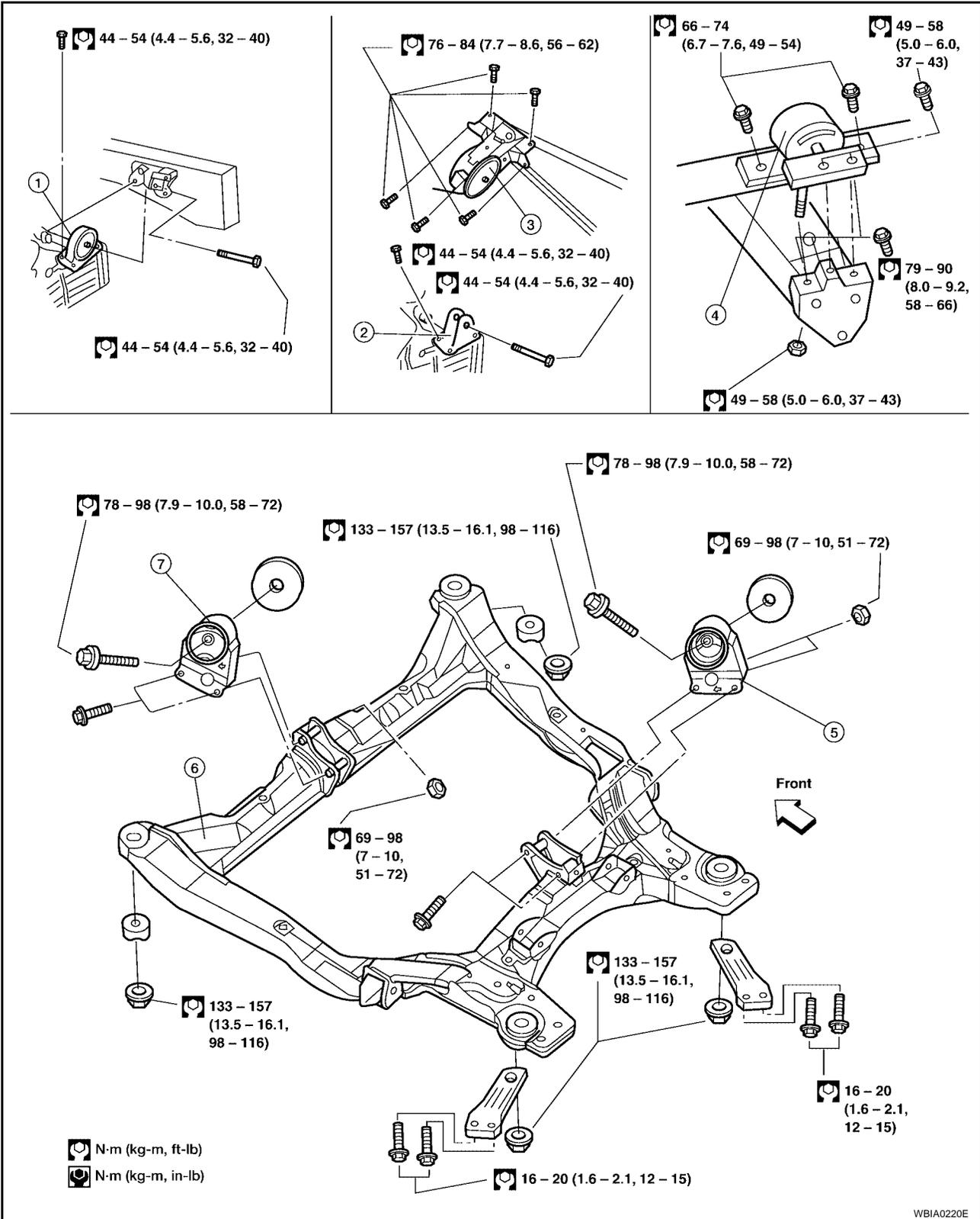
1. LH transaxle mounting insulator (A/T) 2. LH transaxle mounting bracket (M/T) 3. LH transaxle mounting bracket (M/T)
