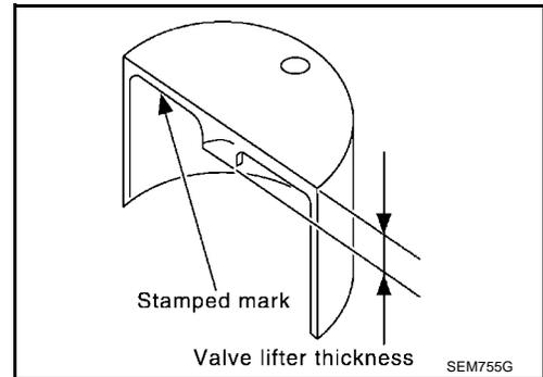
5. Install the selected replacement valve lifter.
