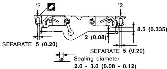
\*2: Remove the protruding sealant from front face. (Remove the hardened sealant from surface only.)
