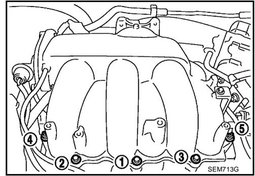
4. Tighten the mounting bolts of the intake manifold collector pipe and electric throttle control actuator assembly diagonally to specification.
