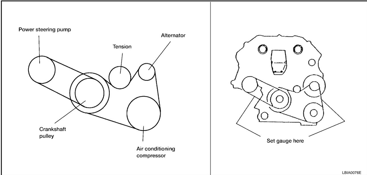
1. Inspect belt for cracks, fraying, wear or oil adhesion. If necessary, replace with a new one.
