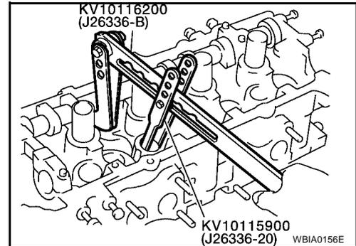
5. Remove valve oil seal with Tool.
