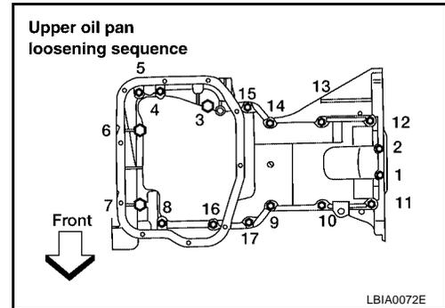
13. Insert the Tool between the upper oil pan and the cylinder block to separate them. Tap gently on the side to move the Tool around the pan; do not damage the mating surface.
