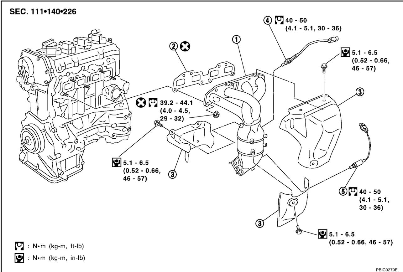
1. Exhaust manifold and three way catalyst assembly
