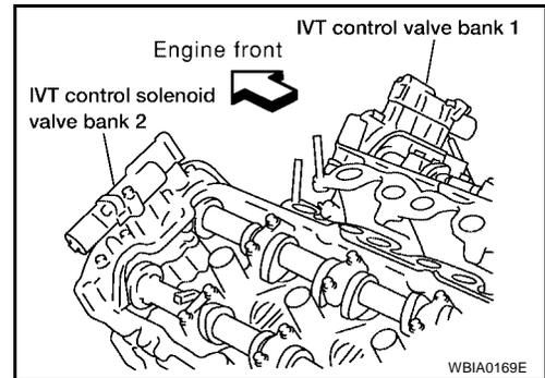
10. Remove the intake and exhaust camshafts and the camshaft brackets.
