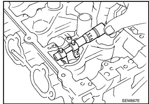
**Calculation of Valve Lifter Clearance**
