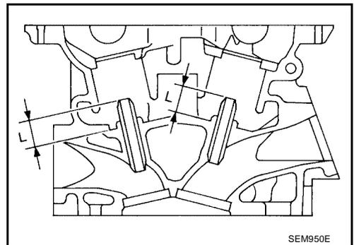
5. Using a valve guide reamer, apply a reamer finish to the valve guide.
