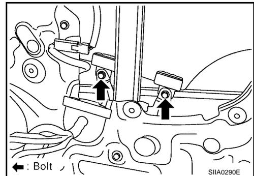
5. Remove the mounting bolts, and remove the regulator and guide channel from the panel.
