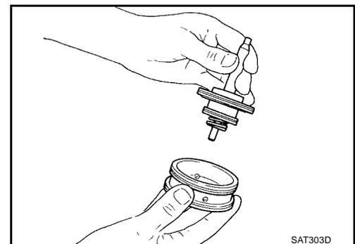
6. Install D-ring to O/D servo piston.
