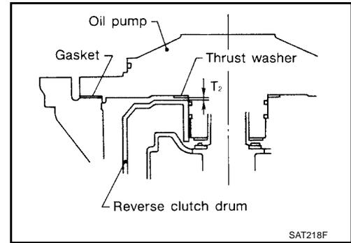
a. Place Tool on machined surface of transmission case (with gasket). Then allow gauging cylinder to rest on reverse clutch drum. Lock cylinder in place with set screw.
