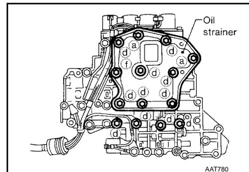
2. Remove solenoid valve assembly and line pressure solenoid valve from control valve assembly.
