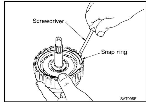
5. Set Tool on spring retainer and remove snap ring from high clutch drum while compressing return springs.
