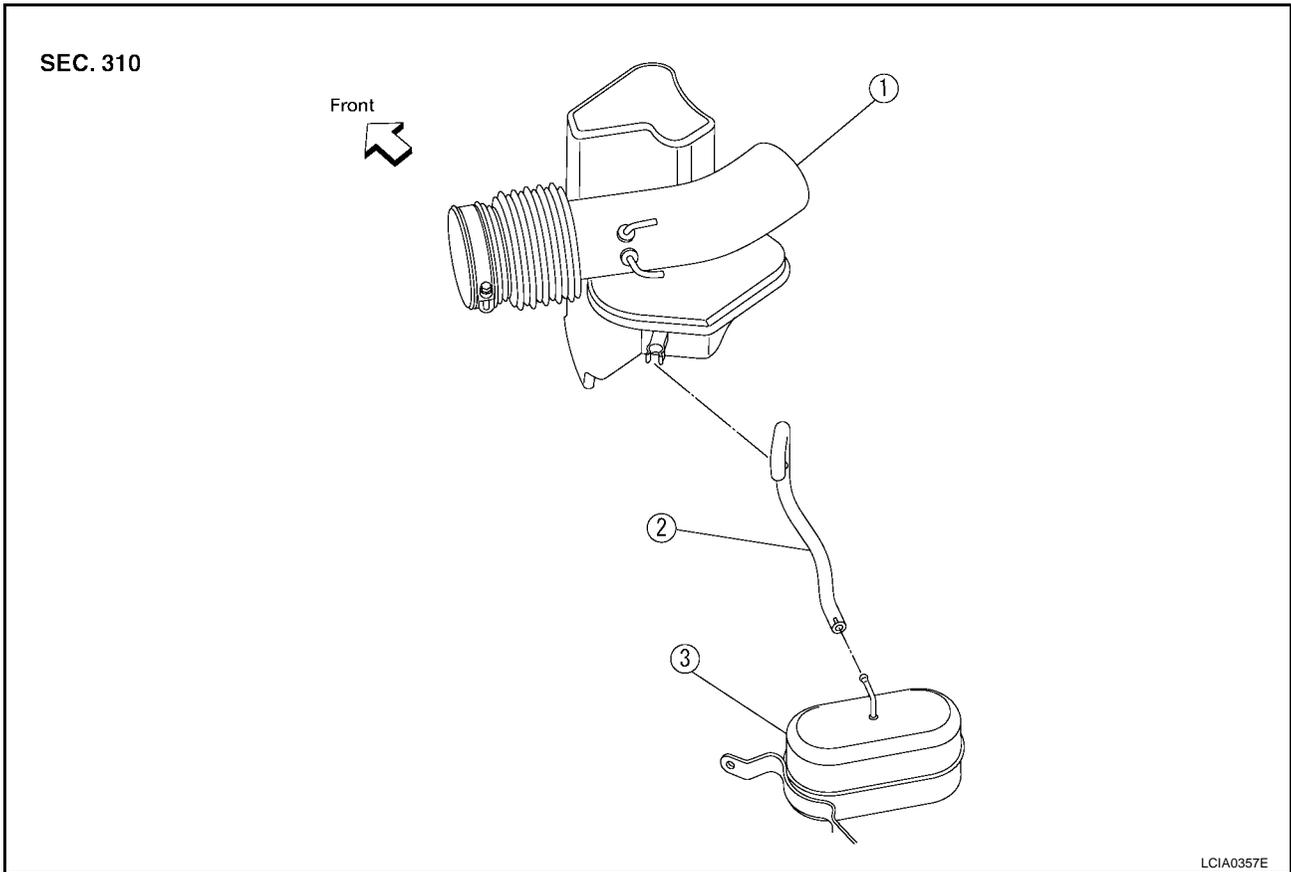
1. Air cleaner to electronic throttle control actuator tube
