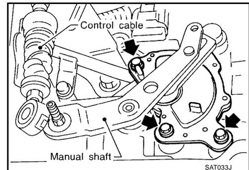
4. Insert pin into adjustment holes in both park/neutral position (PNP) switch and manual shaft as near vertical as possible.
