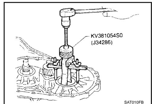
23. Remove differential side bearing adjusting shim from transmission case.
