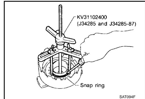
4. Set Tool on spring retainer and install snap ring while compressing return springs.
