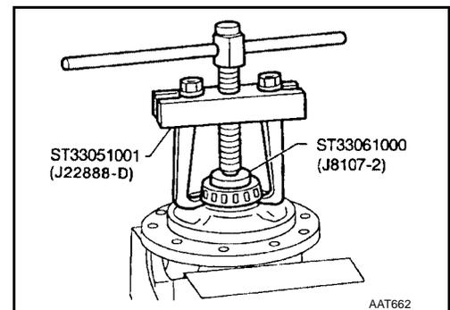
3. Remove differential side bearing outer race and side bearing adjusting shim from transmission case.
