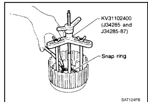
8. Remove forward clutch piston with overrun clutch piston from forward clutch drum by turning it.
