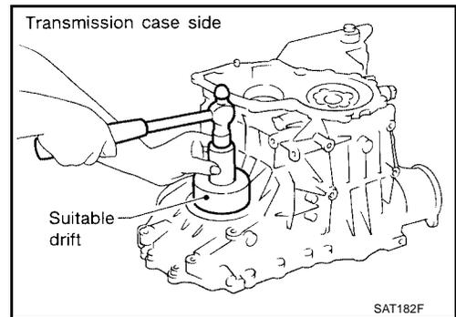
2. Install parking actuator support to transmission case. Tighten parking actuator support bolts to the specified torque. Refer to [AT-273, "OVERHAUL"](#).
