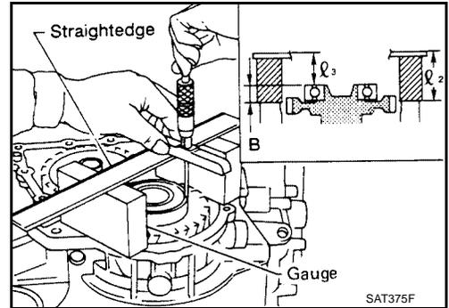
6. Select proper thickness of adjusting shim so that output shaft end play (clearance between side cover and output shaft bearing) is within specifications.
