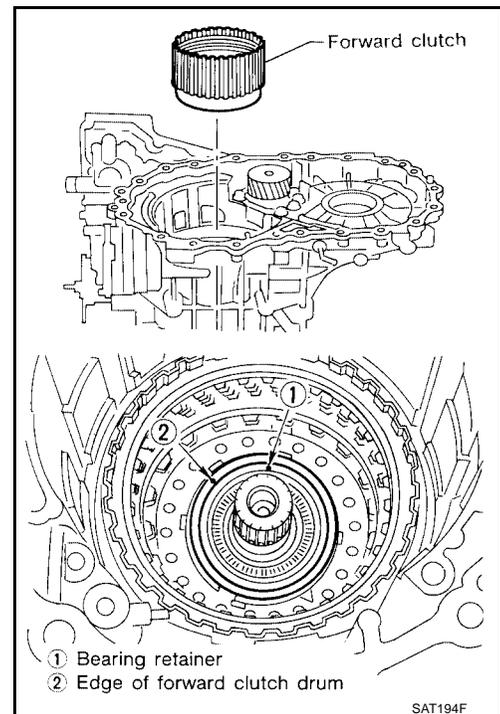
7. Install thrust needle bearing on bearing retainer.
