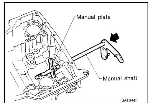
3. Align groove of manual shaft and hole of transmission case.
