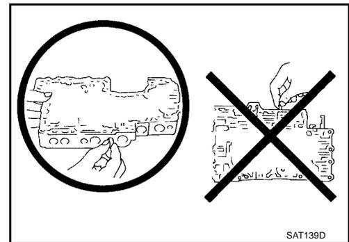
1. Lubricate the control valve body and all valves with ATF. Install control valves by sliding them carefully into their bores.
