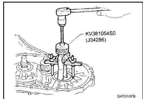
14. Insert Tool and measure turning torque of final drive assembly.
