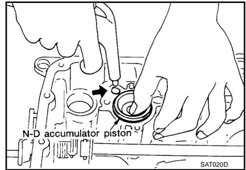
15. Remove O-rings from N-D accumulator piston.
