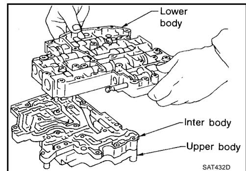
6. Turn over lower body, and remove accumulator support plate.
