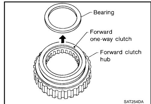
6. Remove forward one-way clutch from forward clutch hub.
