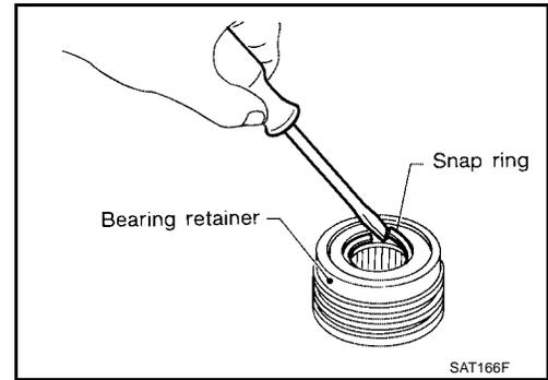
4. Remove needle bearing from bearing retainer.
