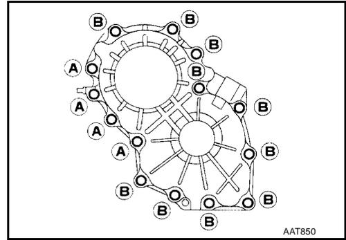
b. Remove side cover by lightly tapping it with a soft hammer.
