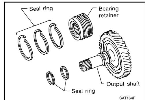
2. Remove output shaft bearing with screwdrivers.
