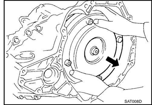
3. Check torque converter one-way clutch using check tool as shown at left.
