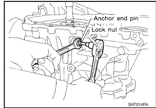
9. Apply compressed air to oil holes of transmission case and check operation of brake band.
