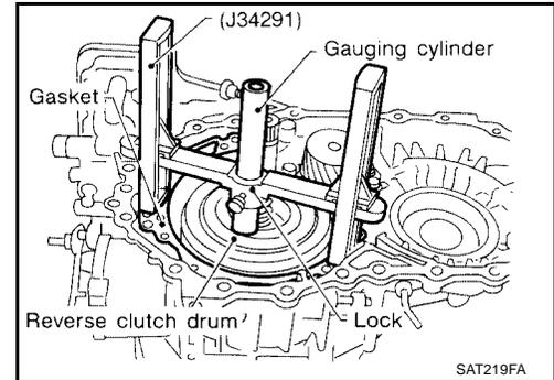
b. Install gauging plunger into cylinder.
