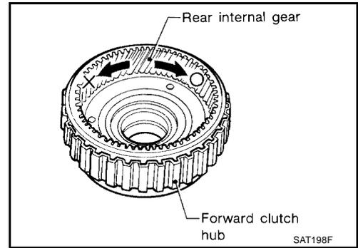
10. Install forward clutch hub and rear internal gear assembly.
