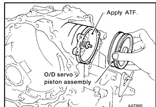
11. Install O/D servo piston retainer to transmission case.
