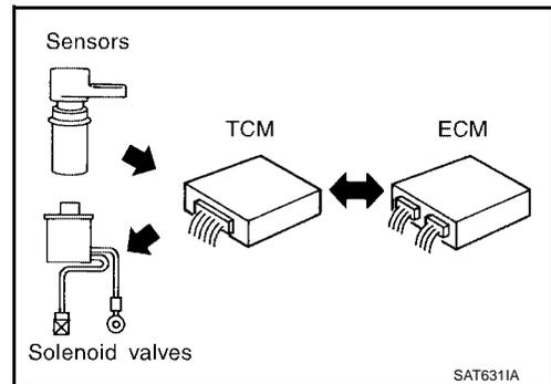
It is much more difficult to diagnose a problem that occurs intermittently rather than continuously. Most intermittent problems are caused by poor electric connections or improper wiring. In this case, careful checking of suspected circuits may help prevent the replacement of good parts.
