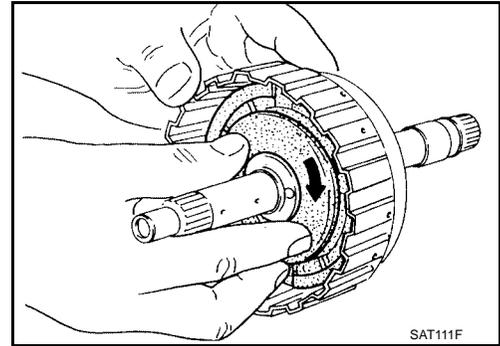
3. Install return springs and spring retainer on piston.
