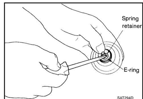
8. Remove O/D servo return spring, band servo thrust washer and band servo piston stem from band servo piston.
