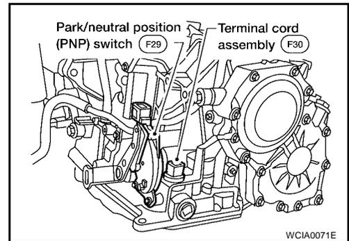
4. Remove stopper ring from terminal cord assembly harness terminal body.
