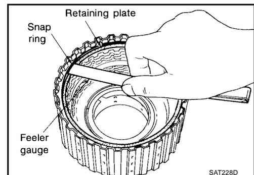
12. Check operation of forward clutch.
