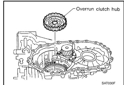
36. Remove needle bearing from overrun clutch hub and check for damage or wear.
