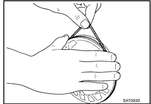
5. Remove oil pump housing oil seal.
