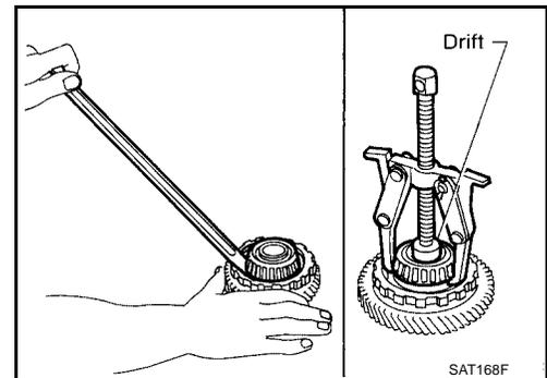
6. Remove idler gear bearing outer race from transmission case.
