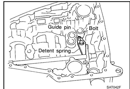
2. Drive out manual plate retaining pin.
