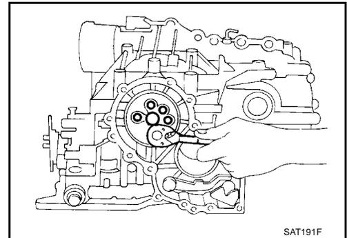
2. Install output shaft thrust needle bearing on bearing retainer.
