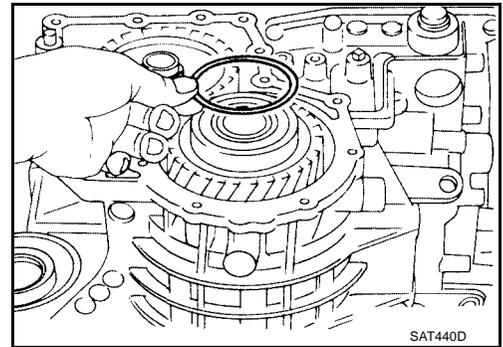
7. Install adjusting shim on output shaft bearing.
