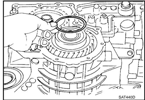
d. Remove output shaft assembly.
