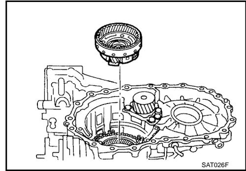
12. Install thrust needle bearing on front planetary carrier, then install them together on transmission case.
