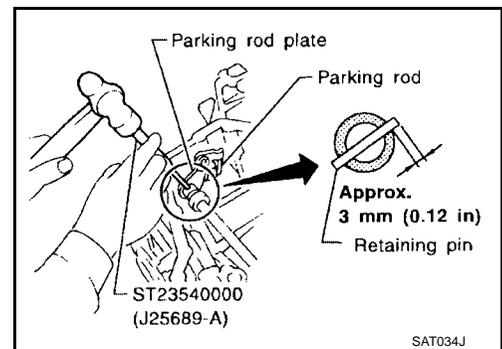
7. Drive manual plate retaining pin.
