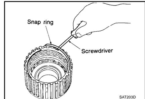
11. Measure clearance between forward clutch retaining plate and snap ring.
