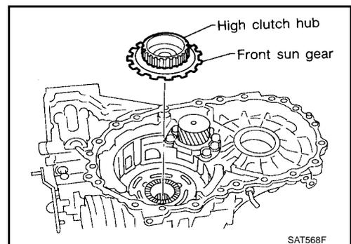
e. Remove front sun gear and needle bearing from high clutch hub and check for damage or wear.
