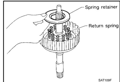
4. Set Tool on spring retainer and install snap ring while compressing return springs.
