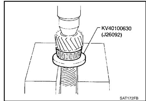
2. Install reduction pinion gear bearing outer race on transmission case.
