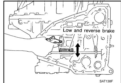
32. Remove low one-way clutch and front planetary carrier assembly according to the following procedures.
