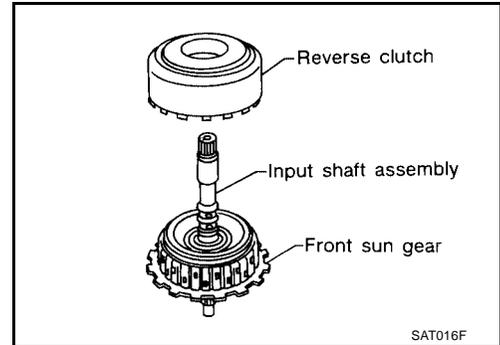
22. Install reverse clutch assembly on transmission case.
