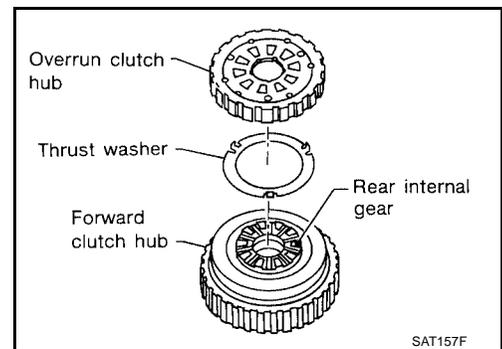
6. Install forward clutch hub on rear internal gear.
