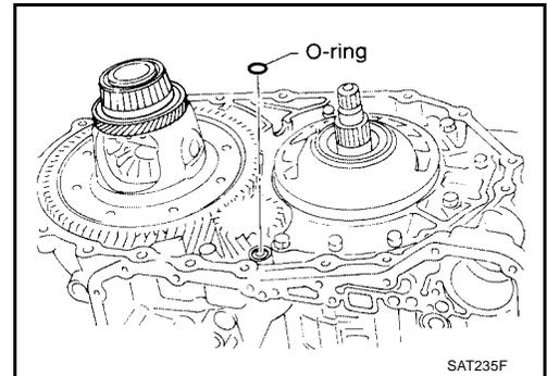
21. Remove final drive assembly from transmission case.
