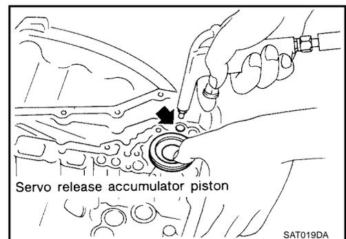
13. Remove O-rings from servo release accumulator piston.
