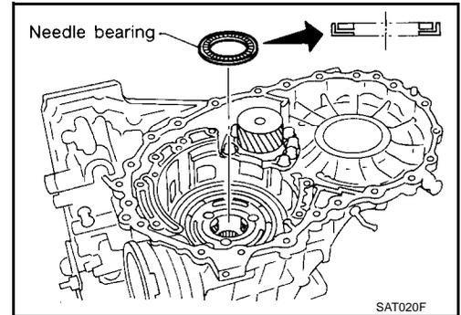
17. Install bearing race, needle bearing and high clutch hub on front sun gear.
