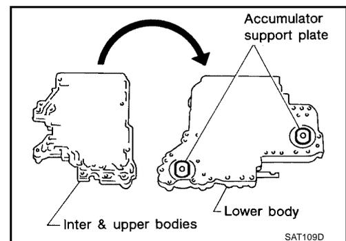
7. Remove bolts **e** , separating plate and separating gasket from lower body.
