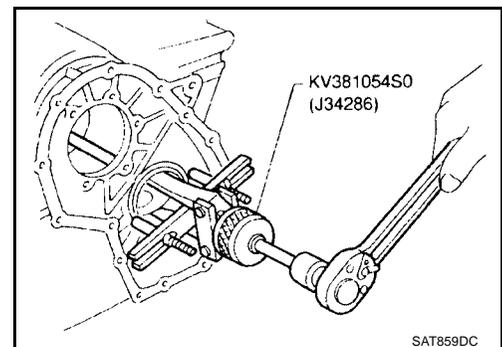
7. Press out reduction pinion gear bearing inner race from reduction pinion gear.
