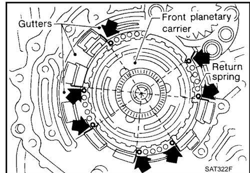
b. Set and align piston with retainer.
