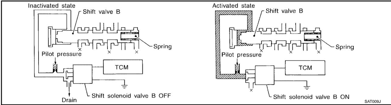
Pilot pressure generated by the operation of shift solenoid valves A and B is applied to the end face of shift valves A and B.
