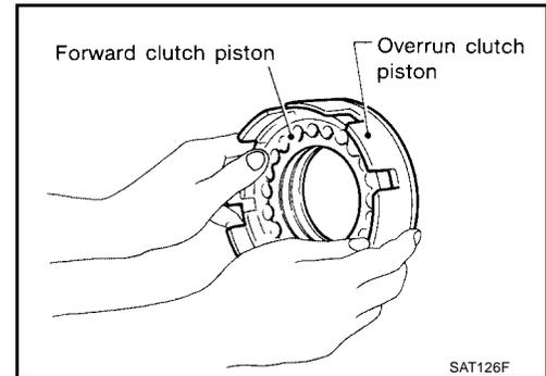
3. Install forward clutch piston assembly on forward clutch drum by turning it slowly.
