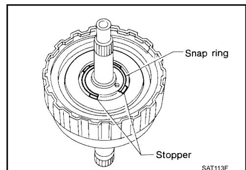
5. Install drive plates, driven plates and retaining plate.
