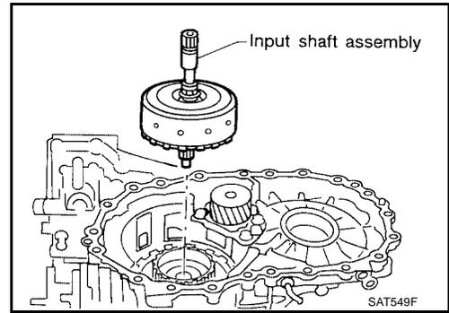
b. Remove input shaft assembly (high clutch) from reverse clutch.
