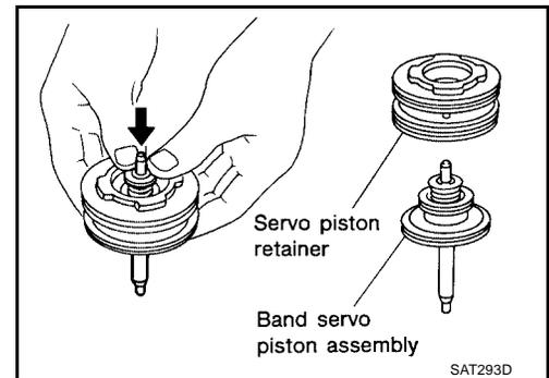
7. Place piston stem end on a wooden block. While pushing servo piston spring retainer down, remove E-ring.
