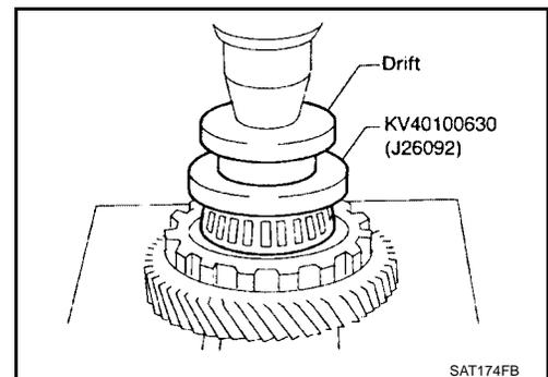
4. Install idler gear bearing outer race on transmission case.
