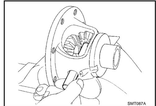
3. Measure clearance between side gear and differential case with washers following the procedure below:
