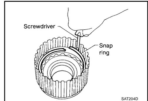
6. Set Tool on spring retainer and remove snap ring from forward clutch drum while compressing return springs.
