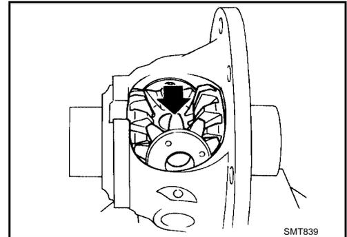
2. Insert pinion mate shaft.
