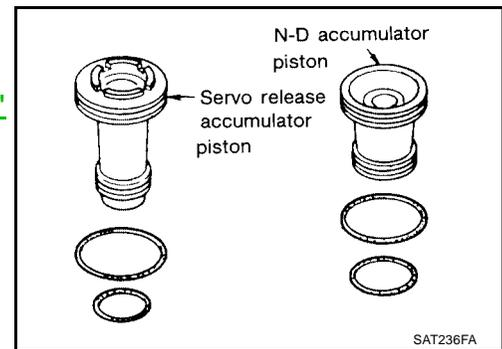
c. Install accumulator pistons and return springs on transmission case.
