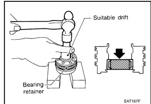
5. Remove idler gear bearing inner race from idler gear.
