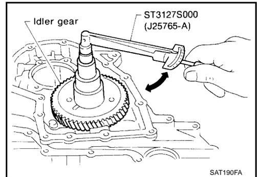
8. After properly adjusting turning torque, clinch idler gear lock nut as shown.
