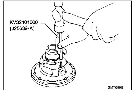
5. Install speedometer drive gear on differential case.
