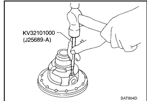
6. Draw out pinion mate shaft lock pin.
