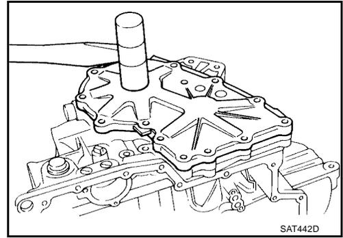
3. Tighten side cover fixing bolts to specified torque. Refer to [AT-273, "OVERHAUL"](#).
