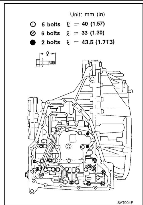
8. Remove servo release and N-D accumulators by applying compressed air if necessary.
