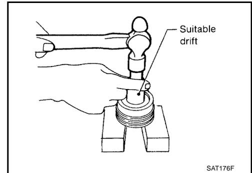
7. Install snap ring to bearing retainer.
