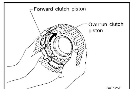
9. Remove overrun clutch piston from forward clutch piston by turning it.
