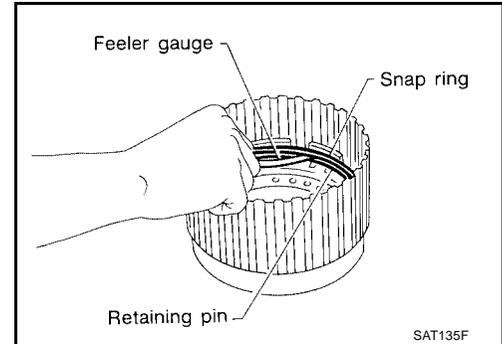
9. Install drive plates, driven plates, retaining plate and dish plate for forward clutch.
