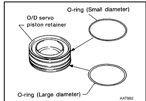
8. Install O/D servo piston to O/D servo piston retainer.
