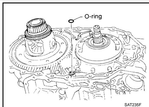
13. Install converter housing on transmission case.
