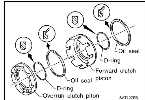
2. Install overrun clutch piston assembly on forward clutch piston by turning it slowly.
