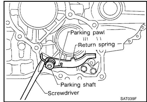
44. Remove parking actuator support from transmission case.
