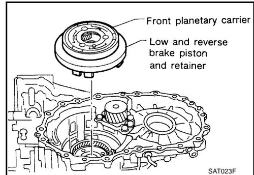
e. Remove low and reverse brake spring retainer.
