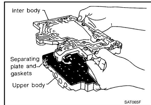
10. Check to see that steel balls are properly positioned in inter body and then remove them.
