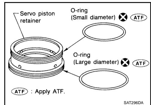
5. Install band servo piston assembly to servo piston retainer by pushing it inward.
