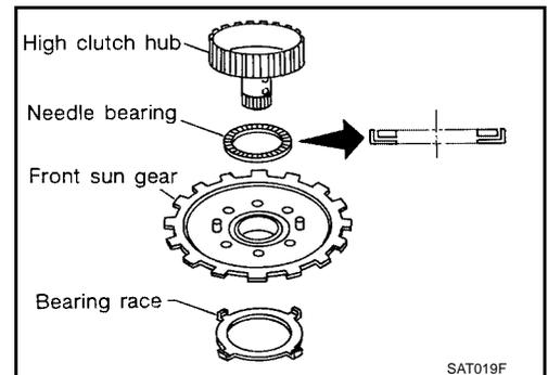
18. Install needle bearing and high clutch drum on high clutch hub.
