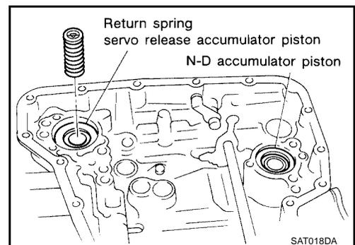
12. Remove servo release accumulator piston with compressed air.
