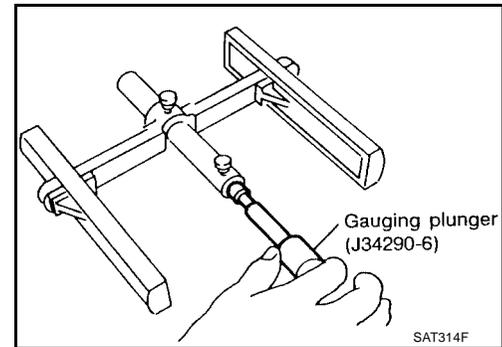
c. With original thrust washer installed on oil pump, place Tool legs onto machined surface of oil pump assembly. Then allow plunger to rest on thrust washer.
