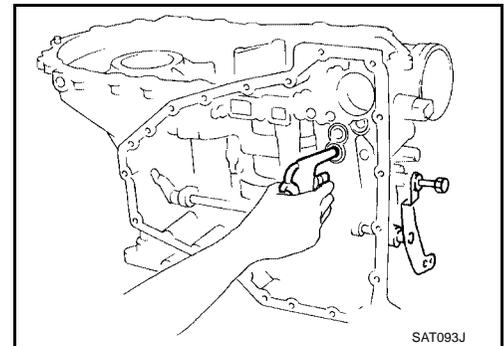
3. Apply compressed air to oil hole in O/D servo piston retainer to remove O/D servo piston from retainer.
