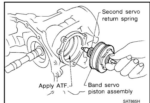
10. Install O/D servo piston assembly to transmission case.
