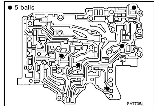
11. Check to see that steel balls are properly positioned in upper body and then remove them.
