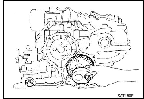
7. Measure turning torque of reduction pinion gear.
