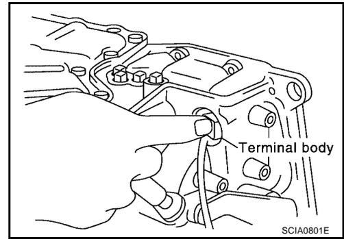
10. Remove manual valve from control valve assembly.
