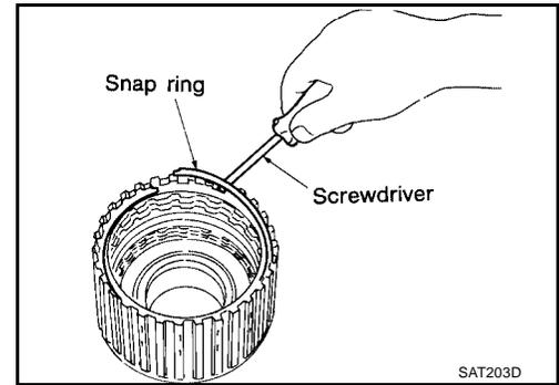
4. Remove snap ring for overrun clutch.
