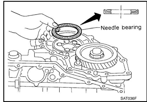
40. Disassemble reduction pinion gear according to the following procedures.
