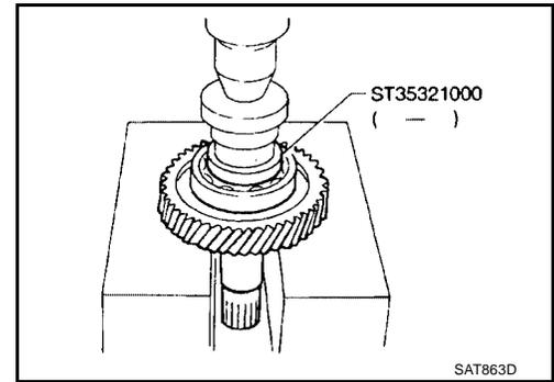
6. Press needle bearing on bearing retainer.
