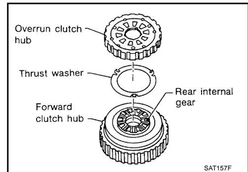
2. Remove forward clutch hub from rear internal gear.
