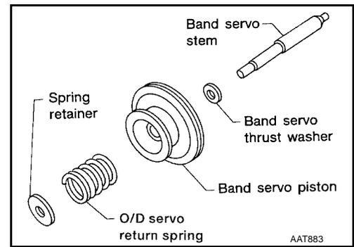
3. Place piston stem end on a wooden block. While pushing servo piston spring retainer down, install E-ring.
