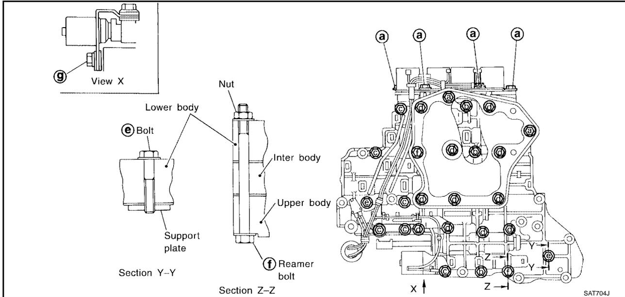
1. Remove bolts **a**, **d** and nut **f** and remove oil strainer from control valve assembly.
