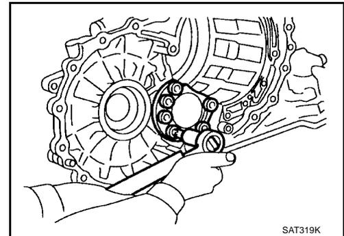
3. Press idler gear bearing inner race on idler gear.
