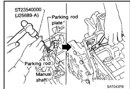
6. Pull out manual shaft retaining pin.
