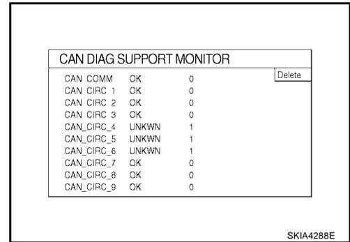
3. Record each item display description (OK/NG/UNKWN) displayed on the following CAN DIAG SUPPORT MONITOR Check Sheet.
