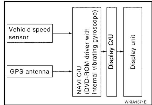
By comparing the vehicle position detection results found by the GPS and by map-matching, more accurate vehicle position data can be used.
