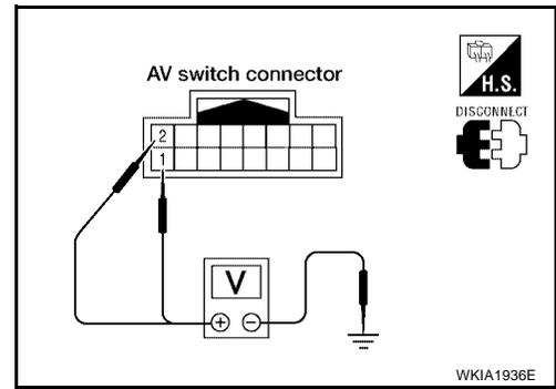
4. Check voltage between BOSE speaker amp. (with BOSE) and ground.
