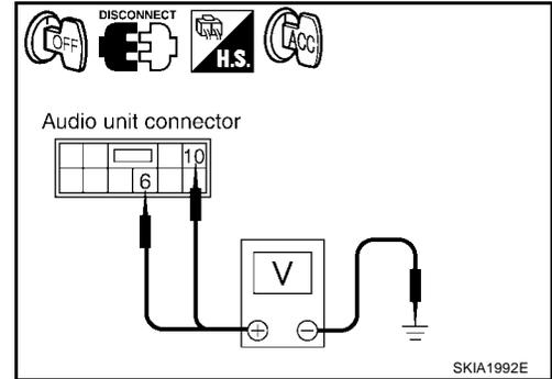
3. Check voltage between AV switch (with NAVI) and ground.
