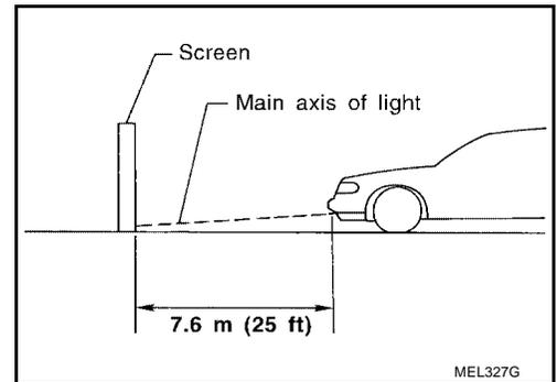
3. Adjust front fog lamps using adjusting screw so that the top edge of the high intensity zone is 100 mm (4 in) below the height of the fog lamp centers as shown.
