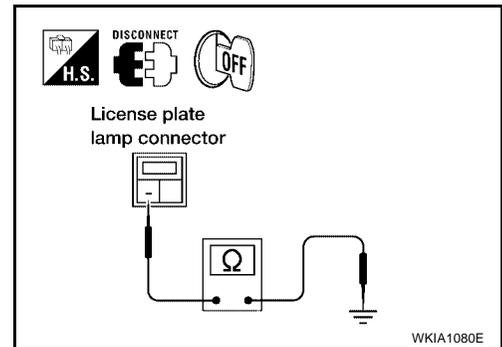
3. Check continuity between rear combination lamp harness connector and ground.
