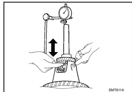
5. If the clearance measured is not within specification, adjust the clearance by changing the thrust washer thickness.
