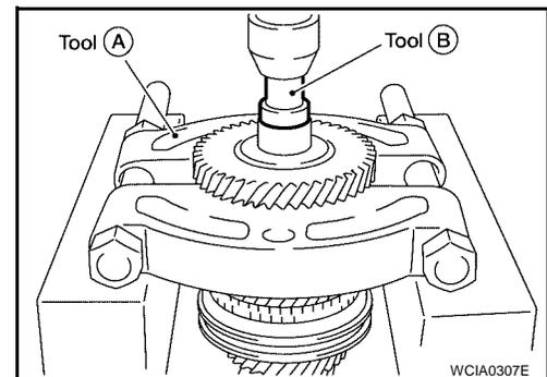
7. Remove the 5th input gear and synchronizer hub assembly simultaneously using Tool as shown.
