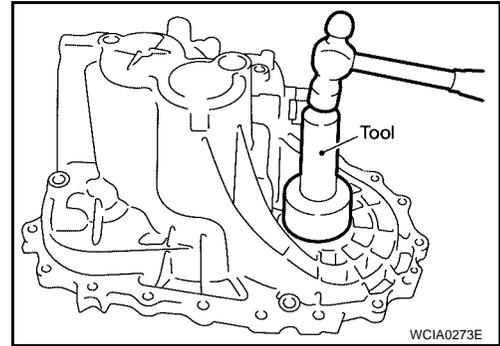
3. Install the oil channel on the mainshaft side as shown.
