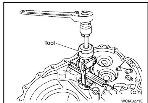
30. Remove the oil channel on the mainshaft side.
