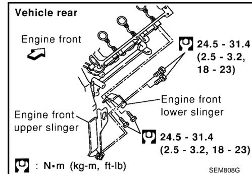
15. Support the engine using an engine support fixture or suitable tool.
