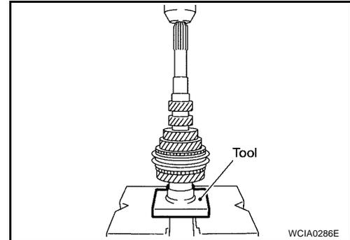
12. Install the synchronizer assembly onto a new 5th-6th synchronizer hub.
