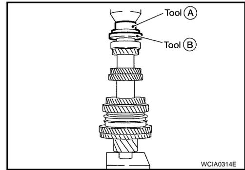
18. Install the C-ring onto the mainshaft, and check that the end play of mainshaft rear bearing meets specifications.
