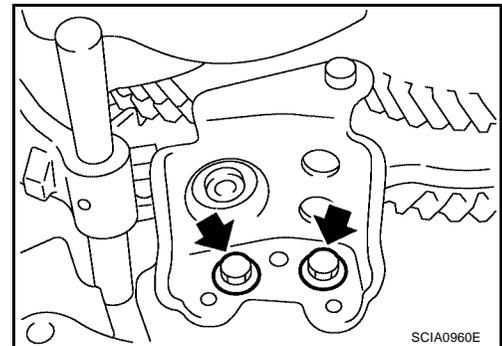
16. Pull out the reverse fork rod then remove the reverse shift fork.
