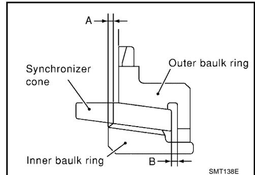
1. Using a dial gauge and Tool, measure clearance "A" at two or more points diagonally opposite, and calculate mean value.
