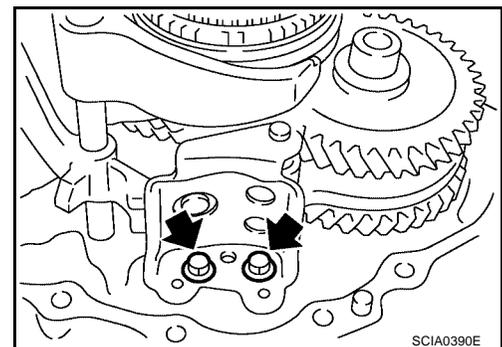
21. Install the magnet onto clutch housing.
