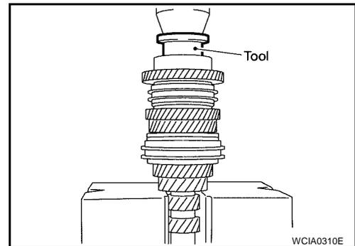
17. Install the input shaft front bearing using Tool as shown.
