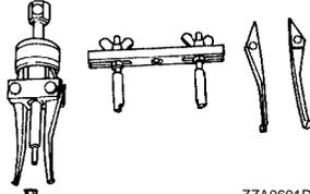
ZZA0601D<br>Removing side bearing outer race<br>Removing mainshaft front bearing                                                                                                                                                                                                                                                                                                                                                                               |
