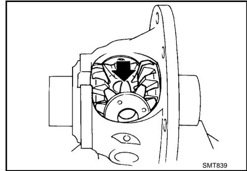
3. While rotating pinion mate thrust washers and pinion mate gears, and aligning them diagonally, install them into differential case.
