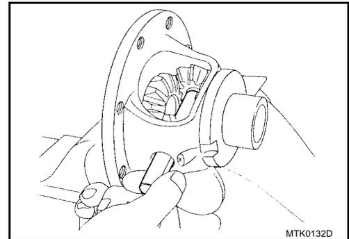
5. Measure end play of side gears using the procedure below, then select a side gear thrust washer.
