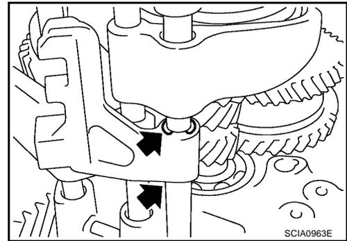
18. Install a new retaining pin onto the 5th-6th shift fork.
