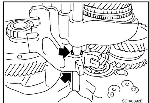
17. Install stopper ring onto 5th-reverse bracket.
