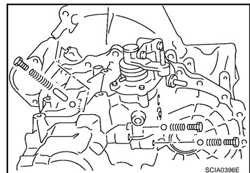
29. Apply Genuine Silicone RTV or equivalent to threads of Park/Neutral position switch and Back-up lamp switch, then install them into transaxle case. Refer to [GI-45, "RECOMMENDED CHEMICAL PRODUCTS AND SEALANTS"](#).
