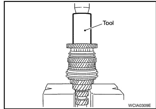
15. Install the snap ring onto the input shaft, and measure to check that end play (gap between snap ring and groove) of the 6th bushing is within specification.
