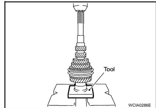
10. Install 5th needle bearing and 5th input gear.
