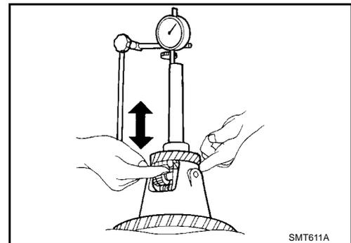
4. If not within specification, adjust the clearance by changing thrust washer thickness.
