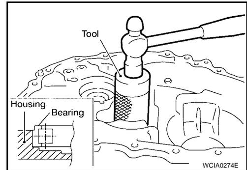
5. Install bearing retainer.
