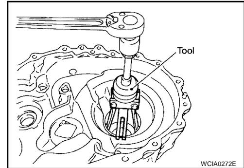
37. Remove the input shaft oil seal using a suitable tool as shown.
