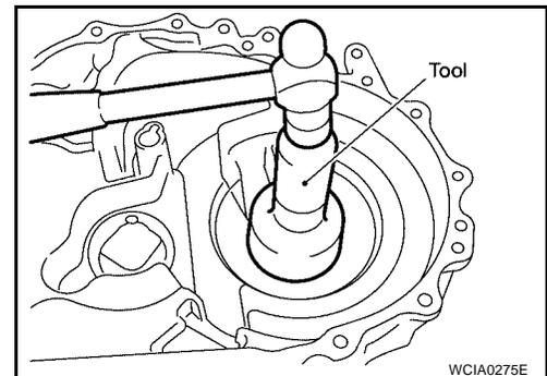
7. Install final drive assembly into clutch housing.
