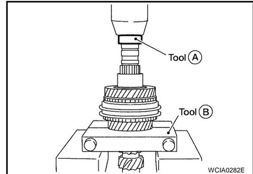
9. Remove 3rd needle bearing.
