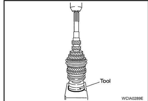
17. Install input shaft front bearing.
