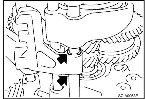
22. Pull out the 5th-6th fork rod and remove the 5th-6th shift fork and the 5th-6th bracket.
