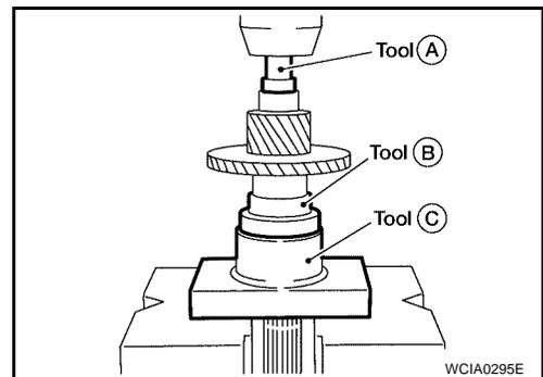
3. Install needle bearing, and then 1st main gear.
