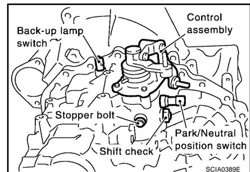
3. After removing shift check and stopper bolt, remove control assembly.
