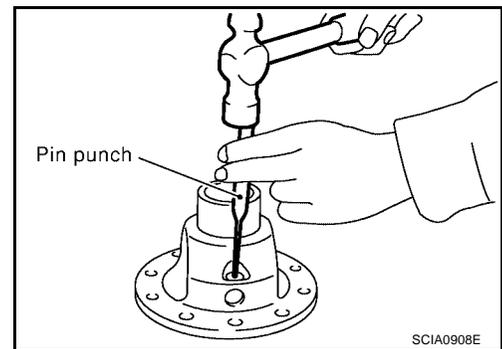
7. Install differential side bearing (transaxle case side) using Tools as shown.
