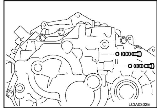
5. Remove the transaxle case fixing bolts as shown.
