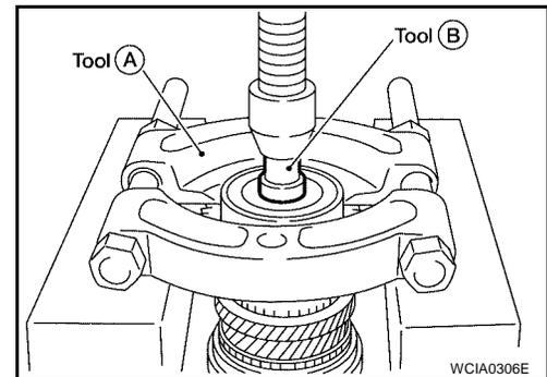
5. Remove the 6th input gear, 6th bushing, and 6th needle bearing using Tool as shown.
