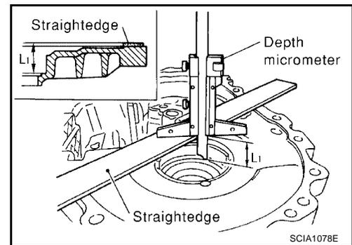
2. Install outer race onto differential side bearing on final gear side. Holding lightly the outer race horizontally by hand, rotate final gear five times or more (for smooth movement of bearing roller).
