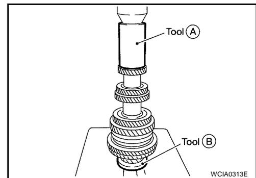
16. Select the 6th main adjusting shim and then install it onto the mainshaft.
