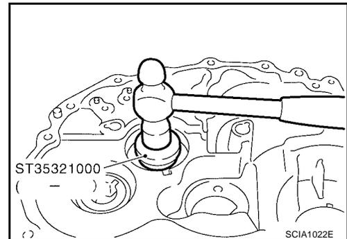
2. Using a drift, install a new differential oil seal.
