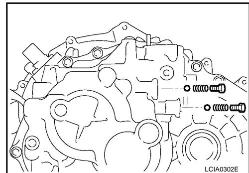
34. Apply sealant to the threads of the park/neutral position switch and back-up lamp switch. Then install them into the transaxle case. Refer to [MT-84, "CASE AND HOUSING COMPONENTS"](#). Use Genuine Silicone RTV or equivalent. Refer to [GI-45, "RECOMMENDED CHEMICAL PRODUCTS AND SEALANTS"](#).
