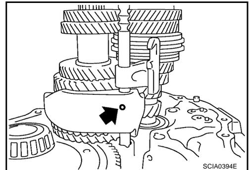
29. Pull out the 1st-2nd fork rod with bracket.
