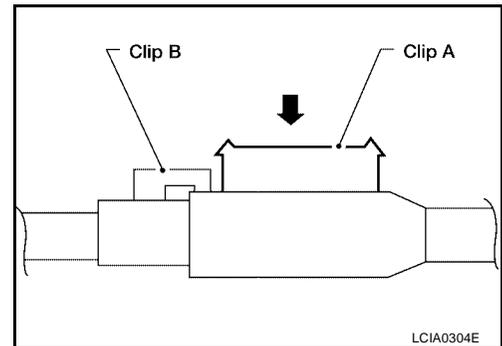
4. Slide clip "B" back over clip "A" until it snaps into place and holds clip "A" in place as shown.
