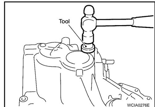
27. Using Tool, install a welch plug as shown.
