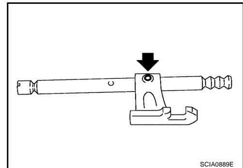
10. Install the 1st-2nd fork rod and the 1st-2nd shift fork, and then install a new retaining pin.
