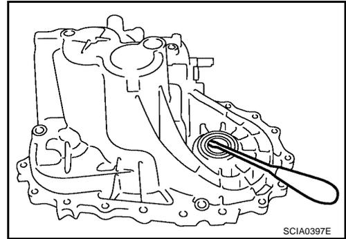
13. Remove magnet from clutch housing.
