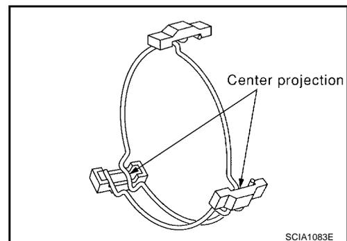
5. Install the 1st gear synchronizer assembly onto the mainshaft, and the synchronizer hub assembly onto the mainshaft using Tool as shown.
