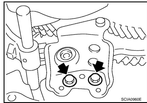
25. Install the check ball, reverse shift check sleeve, reverse check spring, and the reverse check ball plug.
