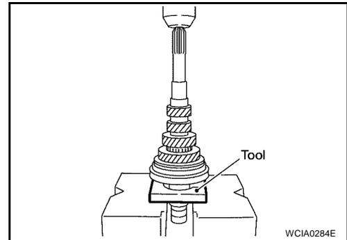
5. Install the 4th bushing using Tool as shown.
