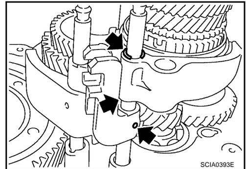
26. Pull out the 3rd-4th fork rod and remove 3rd-4th shift fork and bracket.
