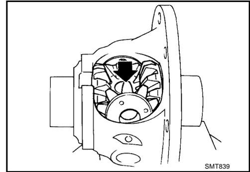
3. While rotating pinion mate thrust washers and pinion mate gears, aligning them diagonally, install them into differential case.
