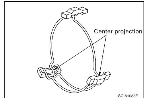
13. Install 5th synchronizer hub assembly.
