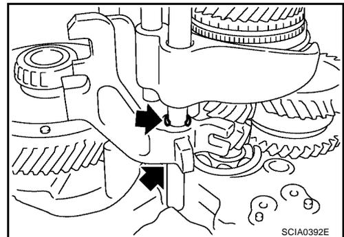
18. Pull out 5th & reverse fork rod and remove 5th shift fork and 5th & reverse bracket.
