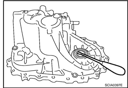
13. Remove the magnet from the clutch housing.
