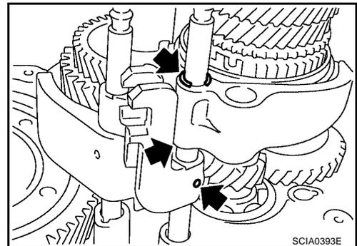
13. Install stopper ring onto 3rd-4th shift fork.
