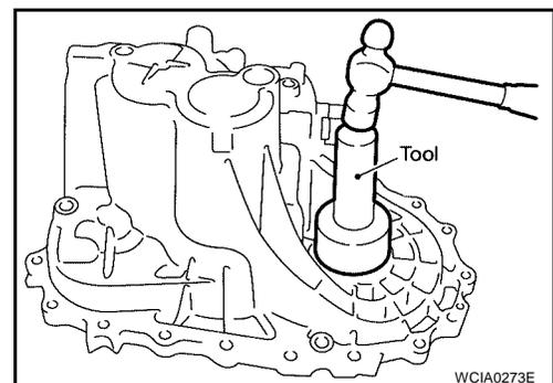
3. Install oil channel on mainshaft side as shown.
