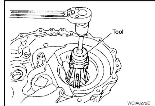
33. Remove input shaft oil seal.
