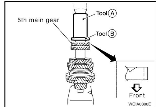
14. Install snap ring onto mainshaft, and check that end play of 5th main gear satisfies standard value.
