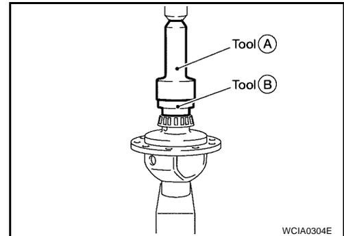
8. Align and install speedometer drive gear onto differential case.
