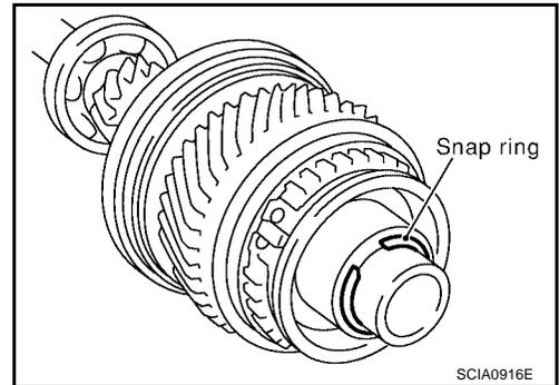
5. Remove input shaft bearing spacer and 5th stopper simultaneously.
