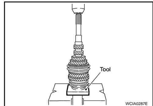
14. Install 5th stopper and then input shaft bearing spacer.
