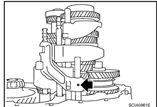
18. Pull out the reverse lever and the reverse bracket fork rod.
