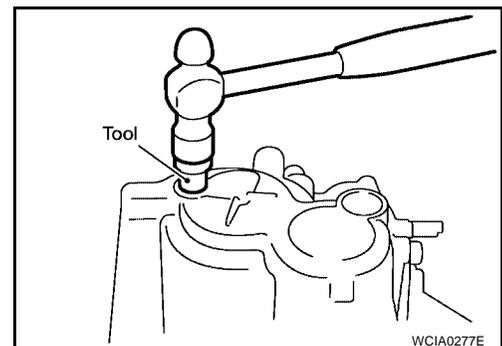
28. Install 1 shift check sleeve, 3 check balls, 3 check springs, and 3 check ball plugs.
