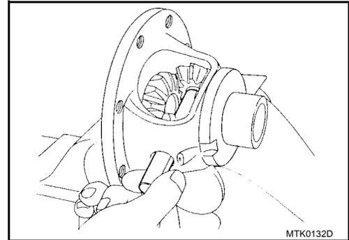
5. Measure end play of side gears, using the procedure below. Then select side gear thrust washer.
