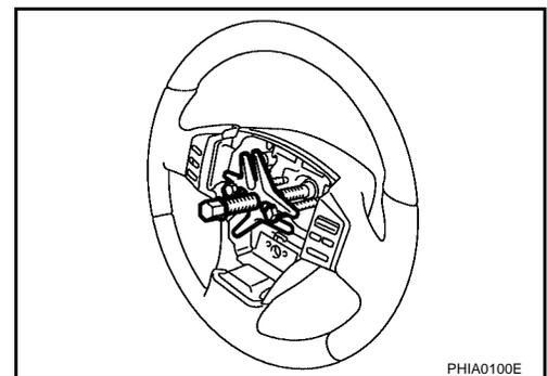
6. Remove the spiral cable screws and remove the spiral cable.
