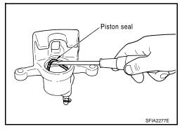
BRAKE CALIPER ASSEMBLY: Assembly
