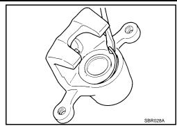
4. Place a wooden block as shown in the figure, and blow air from union bolt mounting hole to remove piston and piston boot. **CAUTION:**
