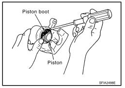
3. Apply brake fluid to piston. Push piston into cylinder body by hand and push piston boot piston side lip into the piston groove. **CAUTION:**
