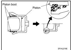
Secure piston boot with retaining ring.
