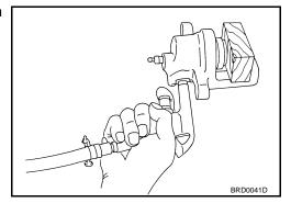
Remove piston seal from cylinder body using a flat-bladed screwdriver.
