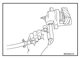
4. Remove piston seal from cylinder body using a flat-bladed screwdriver.
