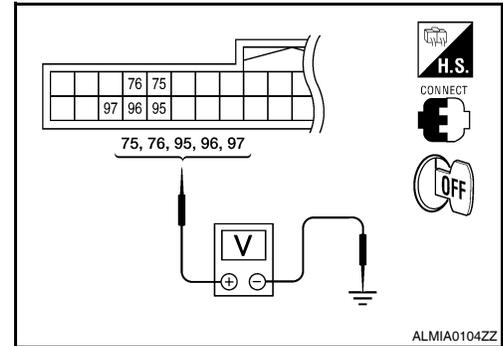
Is the measurement normal when any of the switches are turned ON?
