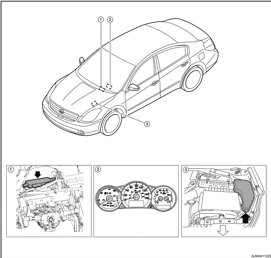
1. BCM M16, M17, M18, M19, M20, M21 (view with instrument panel removed)
