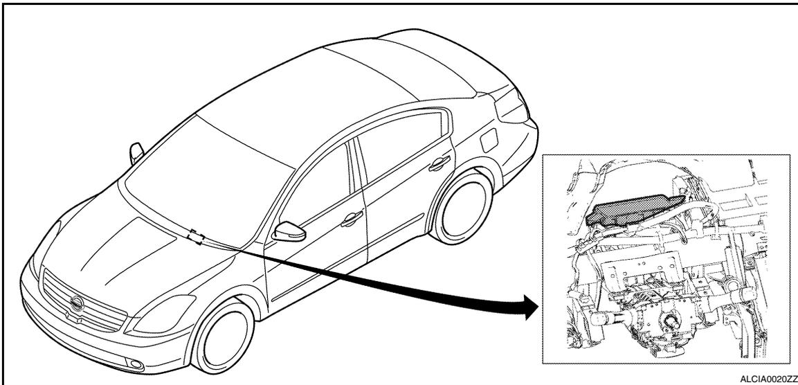
1. BCM M16, M17, M18, M19, M20, M21 (view with instrument panel removed)
