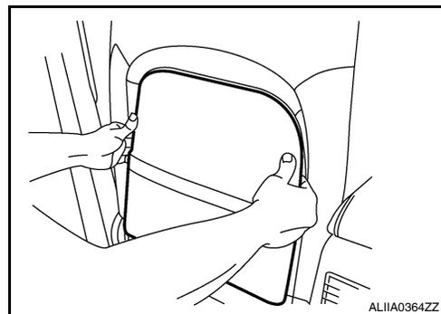
5. Reach in from the bottom of the seatback board to release the top clips. Squeeze the clips at the location shown (A) using suitable tool.
