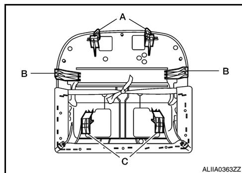
3. Hold the seatback board as shown and push in the side hooks to release them from the seat back frame.
