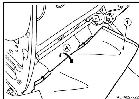
5. Remove the retainer on the seat cushion frame, then remove the harness connector for the seat heater.
