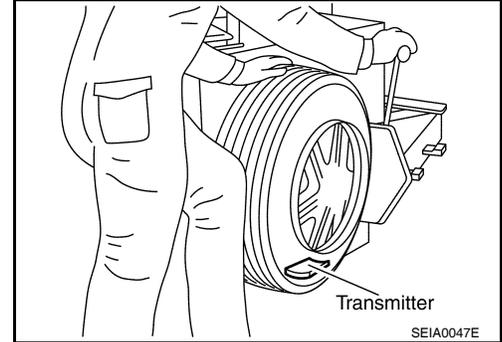
4. Turn tire so that valve hole is at bottom, and gently bounce the tire to ensure transmitter is near valve hole. Carefully lift tire onto turntable and position valve hole (and transmitter) 270 degrees from mounting/dismounting head.
