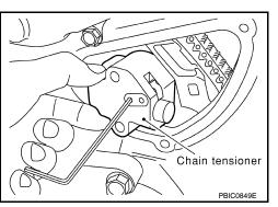
12. Remove the three water pump bolts. Make a gap between water pump gear and timing chain, by turning crankshaft pulley counterclockwise until timing chain loosens on water pump sprocket.
