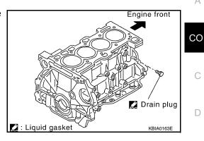
Check the drained coolant for contaminants such as rust, corrosion or discoloration. If the coolant is contaminated, flush the engine cooling system.
