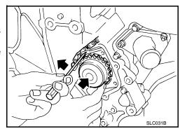
Remove dust and foreign material completely from backside of chain tensioner and from installation area
