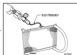
b. Check for leakage.
