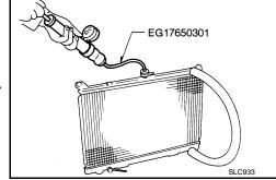
b. Check for leakage.
