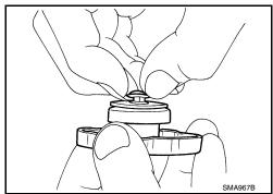
3. Check radiator cap relief pressure using suitable tool and Tool.
