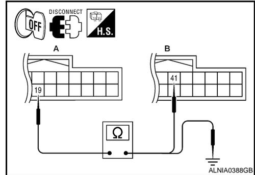
4. Check continuity between display unit harness connector M93 (A) terminal 19 and ground.
