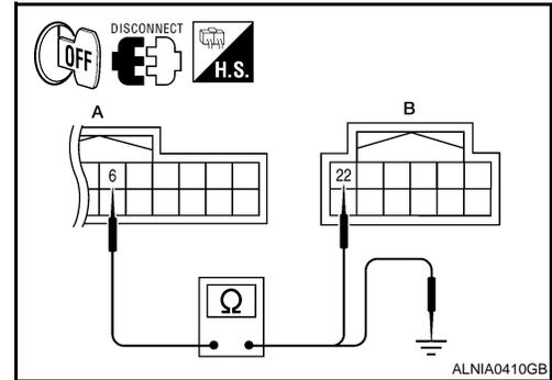
4. Check continuity between display unit harness connector M168 (A) terminal 6 and ground.
