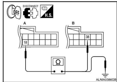
4. Check continuity between display unit harness connector M93 (A) terminal 18 and ground.
