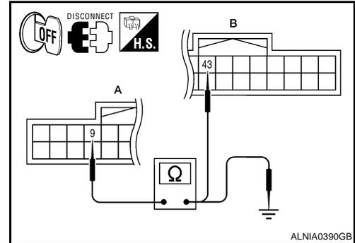
4. Check continuity between display unit harness connector M93 (A) terminal 9 and ground.
