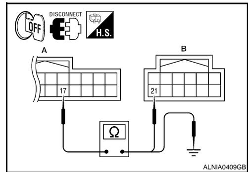
4. Check continuity between display unit harness connector M168 (A) terminal 17 and ground.
