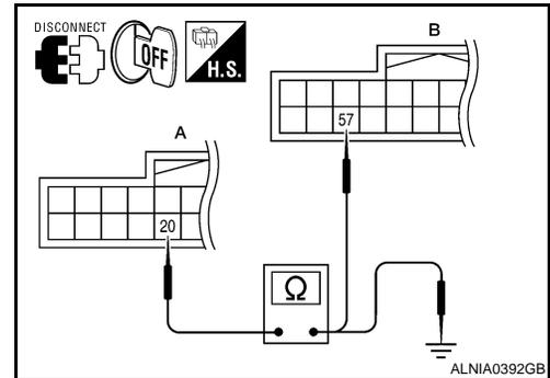
4. Check continuity between display unit harness connector M93 (A) terminal 20 and ground.
