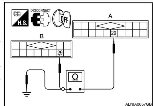
2. Check continuity between satellite radio tuner (factory installed) harness connector M41 (A) terminal 29 and ground.
