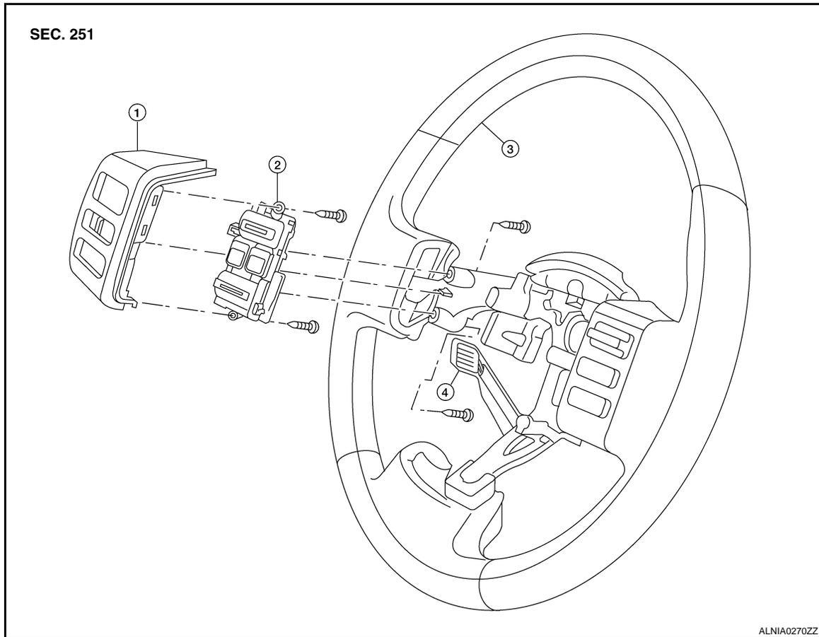
1. Steering wheel audio control switch finisher
