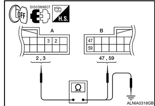
4. Check continuity between the display unit harness connector M93 (A) and ground.
