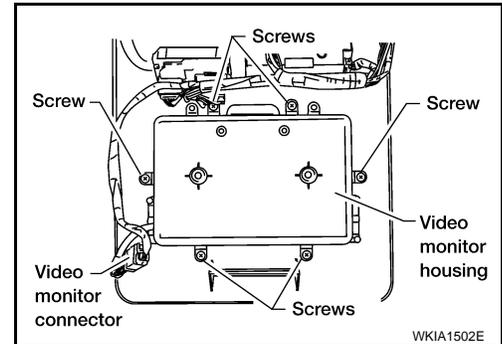
4. Remove video monitor hinge screws.
