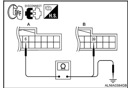
4. Check continuity between display unit harness connector M93 (A) terminal 6 and ground.
