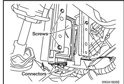
5. Remove the BOSE speaker amp.screws (A). then remove the BOSE speaker amp. (1).
