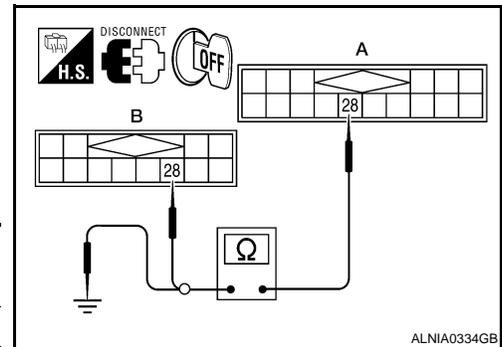
4. Check continuity between satellite radio tuner (factory installed) harness connector M41 (A) terminal 28 and ground.
