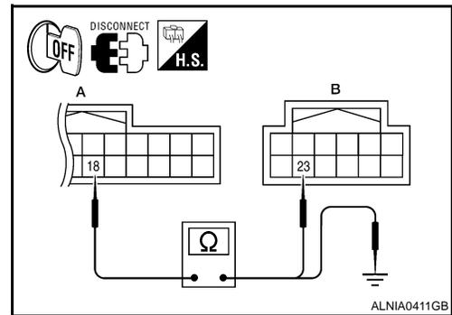
4. Check continuity between display unit harness connector M168 (A) terminal 18 and ground.
