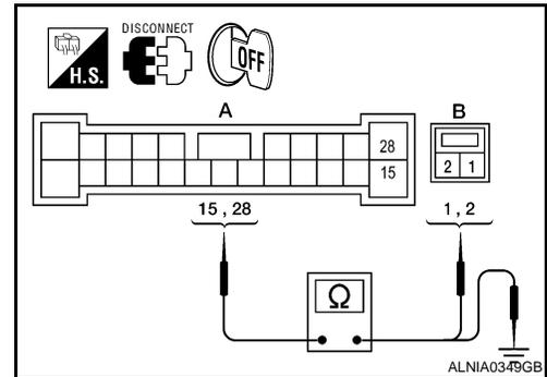
3. Check continuity between BOSE speaker amp. harness connector M113 (A) and ground.
