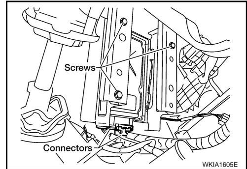
5. Remove the satellite radio tuner screws (A).
