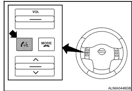
4. While the prompt is playing, press and hold the steering wheel audio control switch
