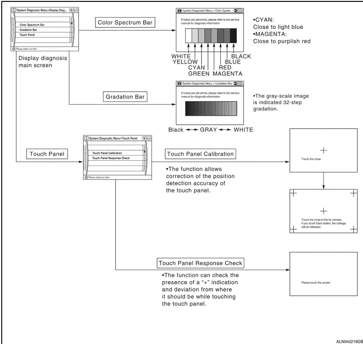
The tint of the color bar indication is as per the following list if RGB signal error is detected.
