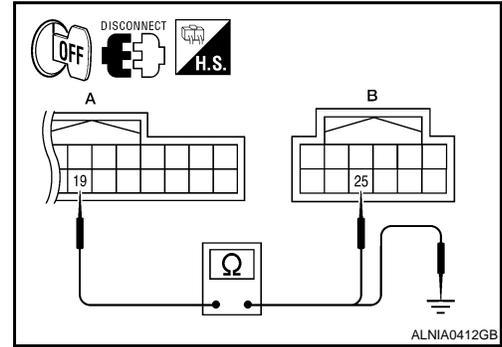
4. Check continuity between display unit harness connector M168 (A) terminal 19 and ground.
