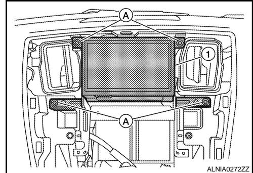
3. Remove the A/C auto amp. screws (A) and the A/C auto amp. (1).
