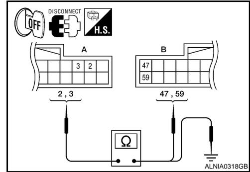
4. Check continuity between the display unit harness connector M93 (A) and ground.
