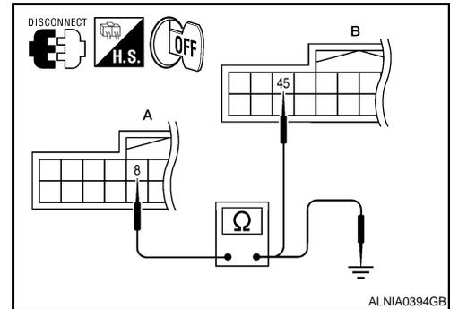
4. Check continuity between display unit harness connector M93 (A) terminal 8 and ground.
