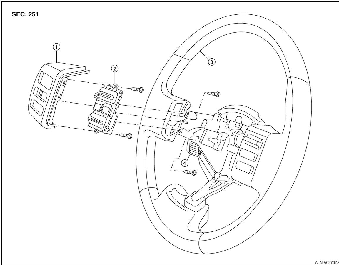
1. Steering wheel audio control switch finisher
