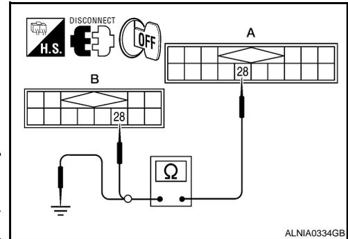
4. Check continuity between satellite radio tuner (factory installed) harness connector M41 (A) terminal 28 and ground.
