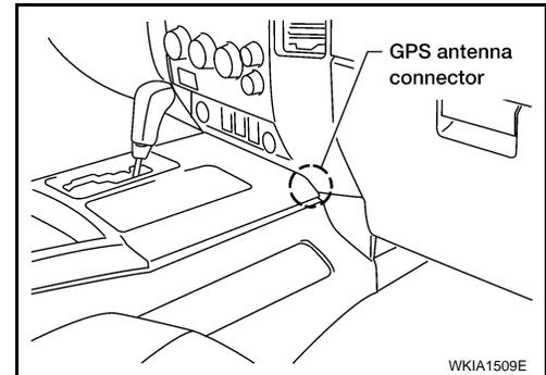
7. Remove the GPS antenna.
