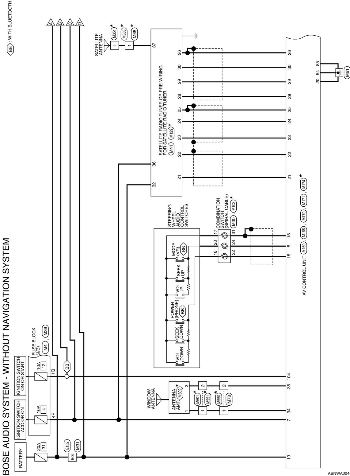
\*: THIS CONNECTOR IS NOT SHOWN IN "HARNESS LAYOUT" OF PG SECTION.
