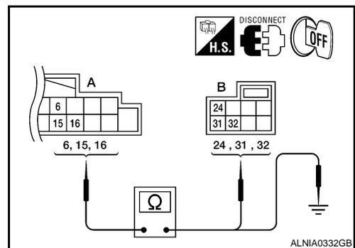
3. Check continuity between AV control unit connector M160 (A) and ground.
