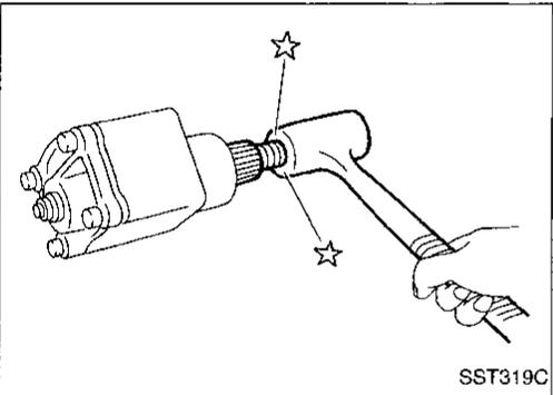
3. Loosen (do not remove) sector shaft cover bolt.
