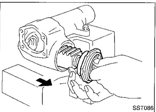
5. Remove worm gear together with worm bearing.
