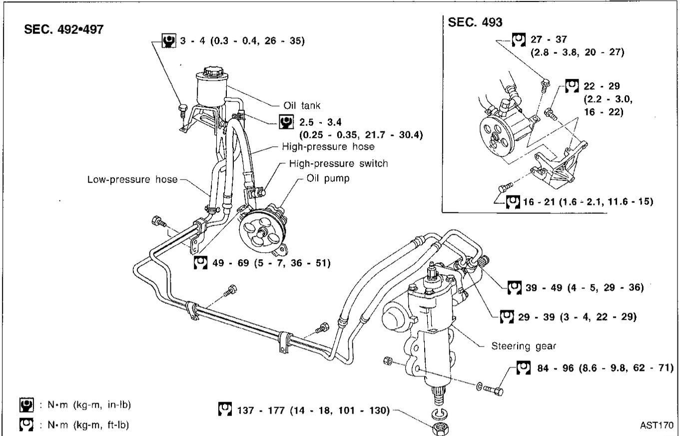
This power steering adopts spool valve control which was developed in a technical tie-up with the ZF Company.
