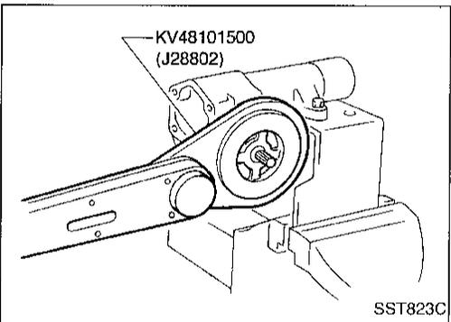
4. Loosen adjusting plug lock nut using Tool.
