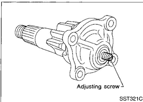
8. Install sector shaft into sector shaft cover. Set adjusting screw to its outermost position.
