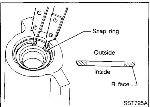
2. Install a new snap ring into gear housing.
