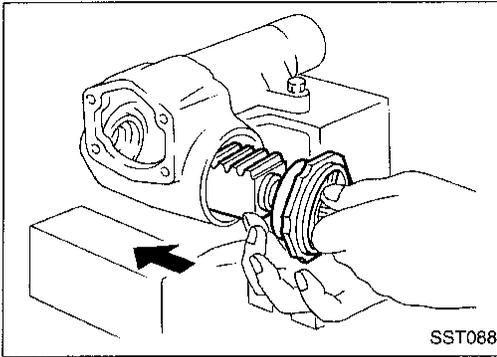
2. Place worm gear assembly together with worm gear bearing into gear housing.
