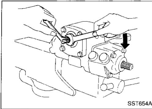
2. Tighten adjusting screw lock nut with tools.
