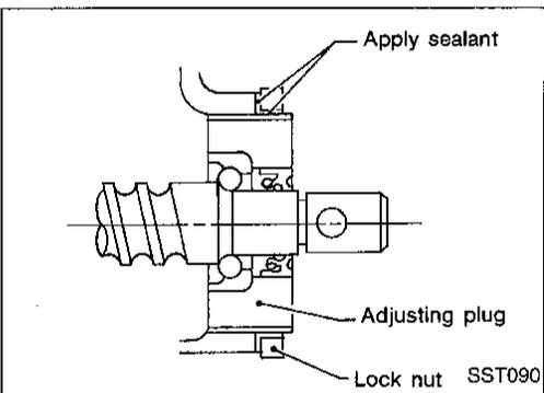
4. Apply suitable sealant to inner surface of lock nut.
