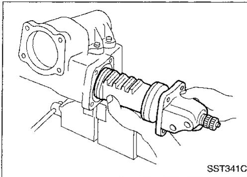
4. Install worm gear assembly with rear housing into the gear housing.
