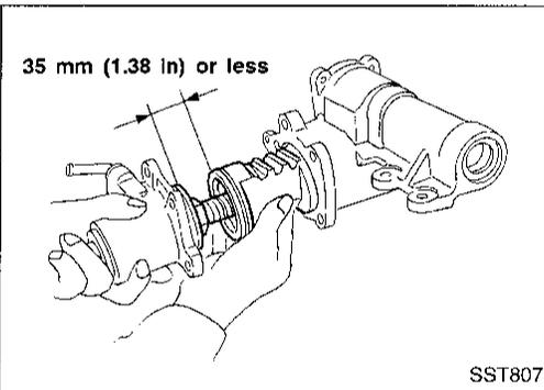
2. Remove rear housing together with worm gear assembly.
