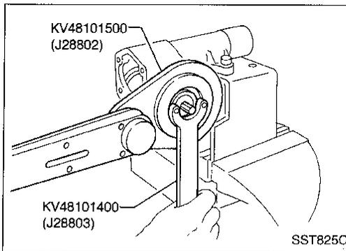
5. Tighten lock nut using Tools.
