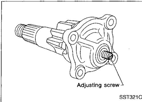
8. Remove lock nut, then loosen adjusting screw using a screwdriver. Separate sector cover and sector shaft.
