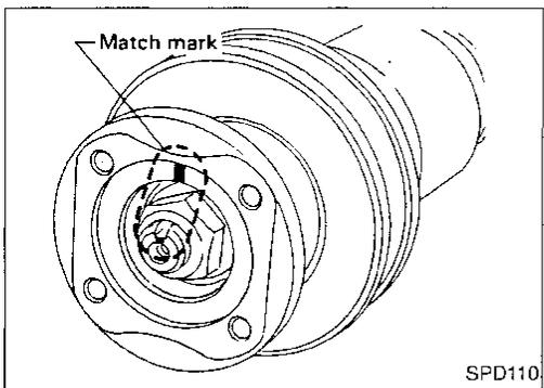
3. Remove locking nut using Tool.
