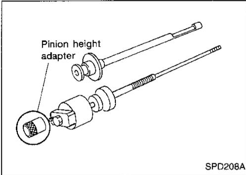
11. Place the J34309-10 pinion height adapter onto the gauge plate and tighten by hand.
