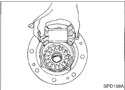
7. Install side gear to pinion mate gears.
