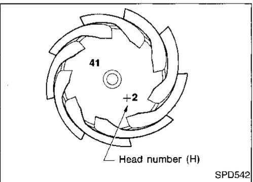
12. Correct the pinion height washer size by referring to the "pinion head number".
