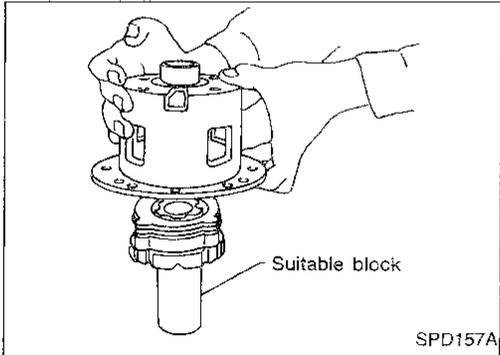
6. Install pinion mate gears, pinion shaft and thrust block to differential case A.
