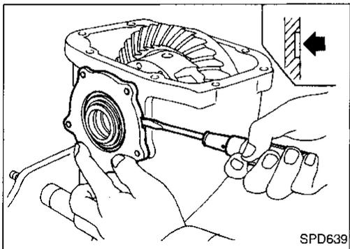
4. Mark side retainers for identification. Remove side retainers. **Be careful not to confuse right and left side retainers and shims.**
