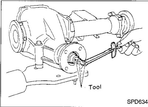
9. Turn drive pinion in both directions several revolutions and measure pinion bearing preload.
