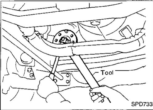
3. Remove companion flange using puller.
