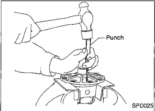
4. Drive out pinion mate shaft lock pin, with Tool from ring gear side.
