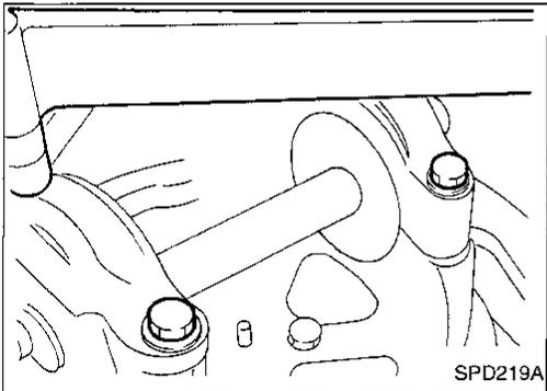
9. Install the side bearing caps and torque the cap bolts.
