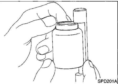
8. Place the solid pinion bearing adjusting spacer squarely into the recessed portion of the J34309-2 gauge anvil.
