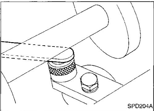
10. Select the correct standard pinion height adjusting washer thickness by using J34309-101 feeler gauge. Measure the gap between the J34309-14 pinion height adapter and the arbor.
