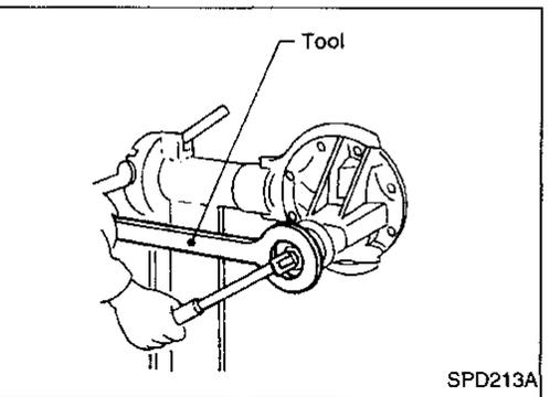
5. Remove drive pinion nut with Tool.
