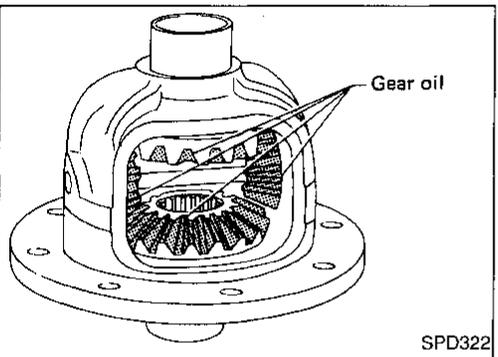
5. Apply gear oil to gear tooth surfaces and thrust surfaces and check to see they turn properly.
