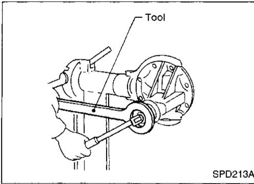
6. Remove drive pinion nut with Tool.
