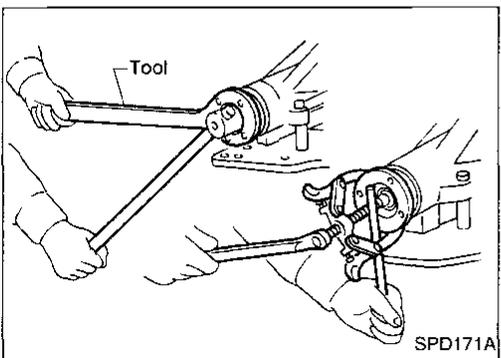
8. Loosen drive pinion nut.
