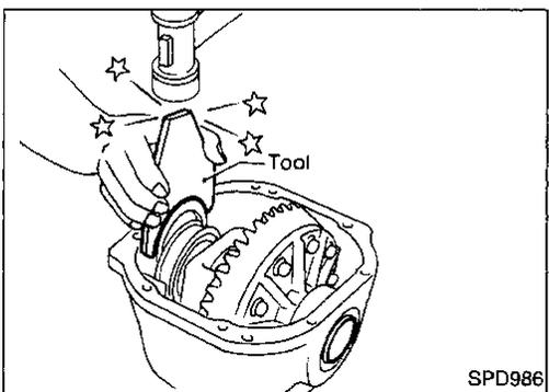
1. Make sure all parts are clean. Make sure, also, the bearings are well lubricated with light oil or type "DEXRON™" automatic transmission fluid.
