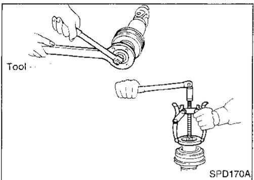
5. Remove center bearing using Tool and press.
