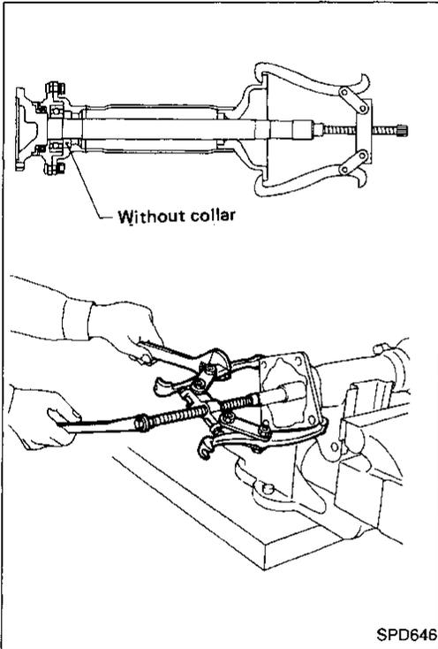
3. Reinstall differential side shaft into extension tube and secure with bolts. Remove rear axle bearing by drawing out differential side shaft from rear axle bearing with puller.
