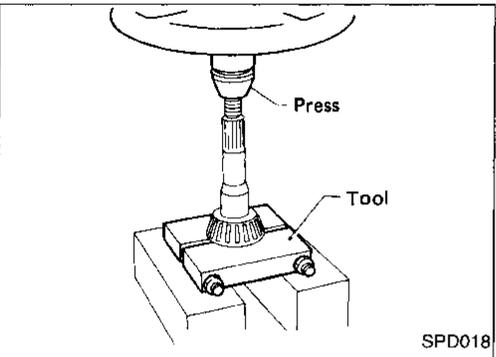
12. Remove pinion rear bearing inner cone and drive pinion adjusting washer.
