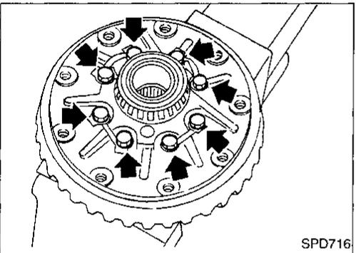
4. Separate differential case LH and RH. Put match marks on both differential case LH and RH sides prior to separating them.
