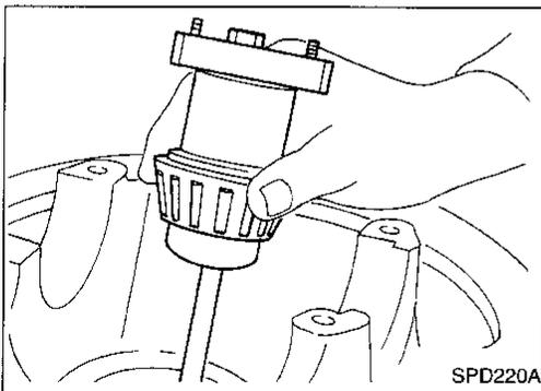
14. Remove the J34309 pinion preload shim selector Tool from the final drive housing and disassemble to retrieve the pinion bearings.
