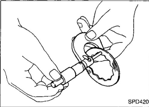
2. Measure thickness of each disc and plate.
