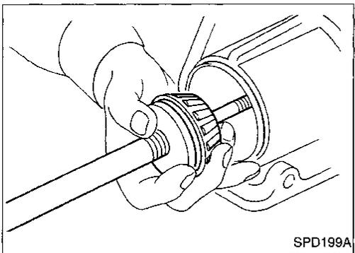
4. Assemble the front pinion bearing inner cone and the J34309-2 gauge anvil. Assemble them together with the J34309-1 gauge screw in the final drive housing. Make sure that the pinion height gauge plate, J34309-16, will turn a full 360 degrees. Tighten the two sections together by hand.
