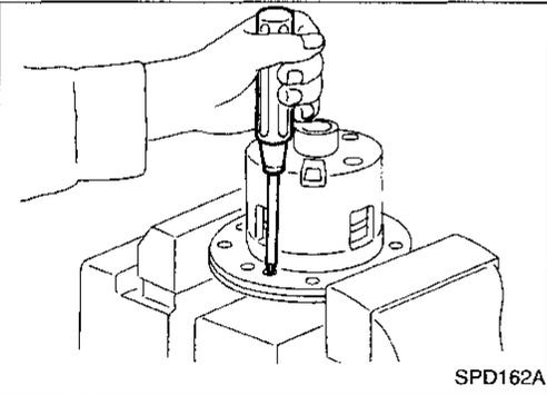
12. Tighten differential case couple screws.
