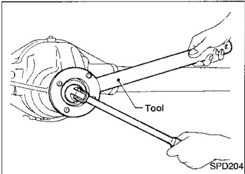
8. Tighten pinion nut to 127 N·m (13 kg·m, 94 ft·lb).
