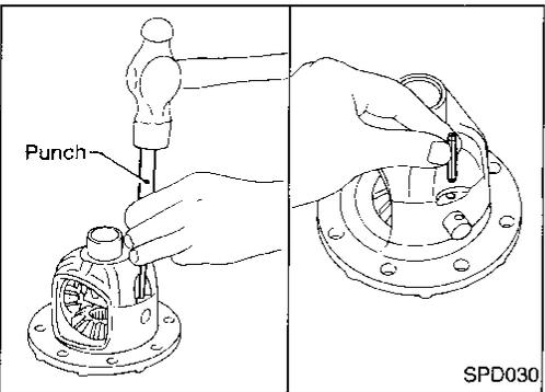
4. Install pinion mate shaft lock pin with a punch.
