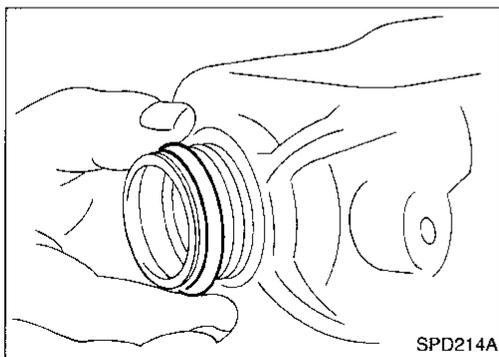
3. Reinstall all of the original side bearing adjusting shims on the carrier side, away from the ring gear.
