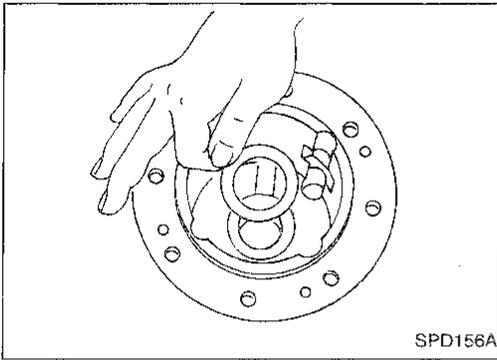
5. Install differential case A over side gear, discs and plates assembly.
