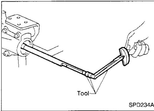
6. Measure the turning torque at the end of the J34309-2 gauge anvil using Tool.
