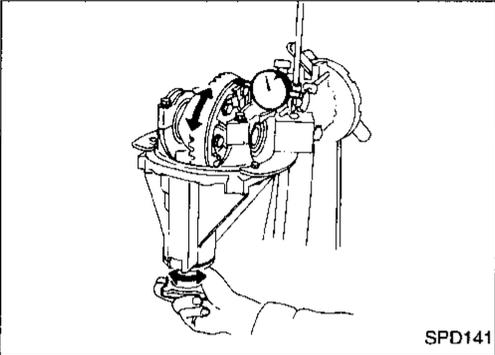
15. Check runout of ring gear with a dial indicator.
