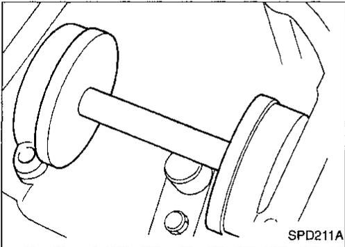
9. Select the correct standard pinion height adjusting washer thickness. Select by using a standard gauge of 3 mm (0.12 in) and J34309-101 feeler gauge. Measure the distance between the J34309-11 pinion height adapter including the standard gauge and the arbor.
