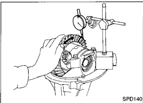
12. Measure ring gear-to-drive pinion backlash with a dial indicator.
