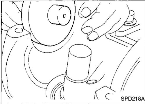
8. Now, position the side bearing discs, J25269-18, and arbor firmly into the side bearing bores.
