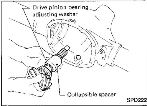
6. Place drive pinion bearing spacer, drive pinion bearing adjusting washer and drive pinion in gear carrier.
