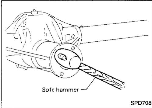
7. Insert companion flange into drive pinion by tapping the companion flange with a soft hammer.
