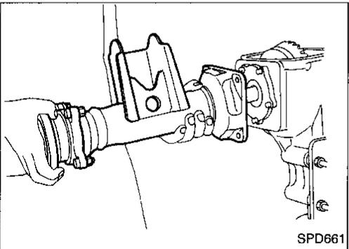
21. Install extension tube and differential side shaft assembly.
