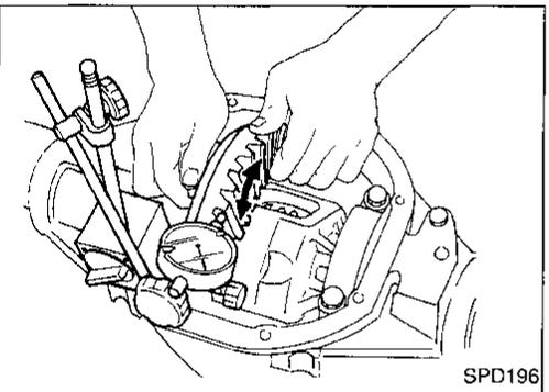
15. Measure ring gear-to-drive pinion backlash with a dial indicator.
