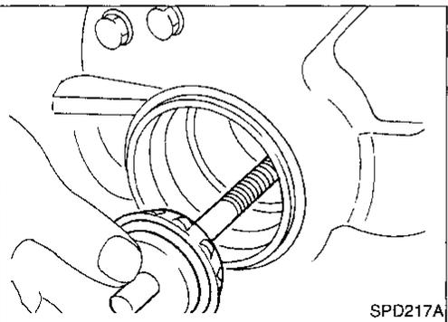
4. Install the J34309-2 gauge anvil with the front pinion bearing into the final drive housing and assemble it to the J34309-1 gauge screw. Make sure that the J34309-16 gauge plate will turn a full 360 degrees, and tighten the two sections by hand to set bearing pre-load.
