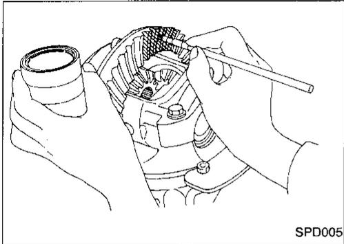
1. Thoroughly clean ring gear and drive pinion teeth.
