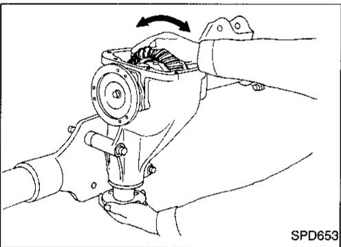
3. Hold companion flange steady and rotate the ring gear in both directions.
