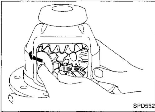
1. Install side gears, pinion mate gears and thrust washers into differential case.
