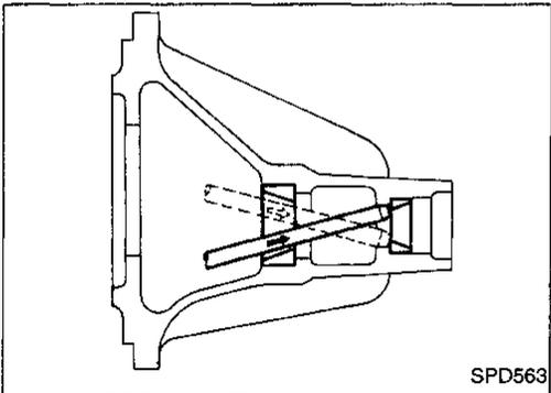
10. Pull out rear bearing inner cone with a press and Tool.
