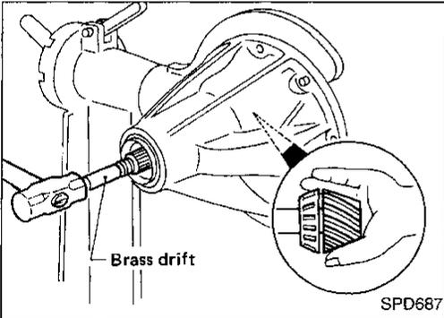
9. Take out drive pinion together with pinion rear bearing inner cone, drive pinion bearing spacer and pinion bearing adjusting shim.
