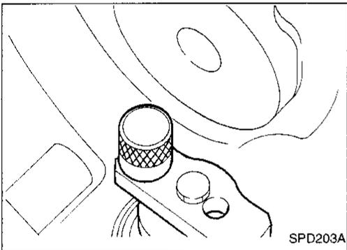
12. Position firmly the side bearing discs, J25269-4, and arbor into the side bearing bores.
