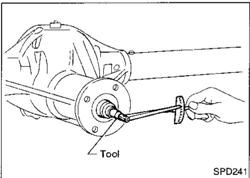
9. Tighten the pinion nut by very small degrees until the specified preload is achieved. When checking the preload, turn the drive pinion in both directions several times to set the bearing rollers.
