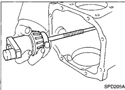
13. Remove the J34309 pinion preload shim selector Tool from the final drive housing. Then disassemble to retrieve the pinion bearings.
