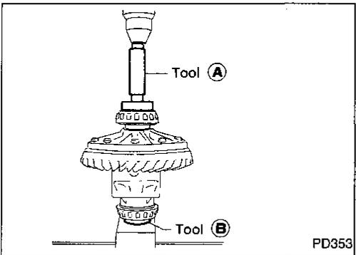
6. Press-fit side bearing inner cones on differential case with Tools.
