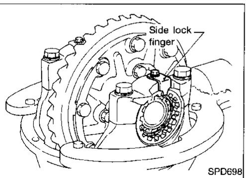
14. Tighten side bearing cap bolts.
