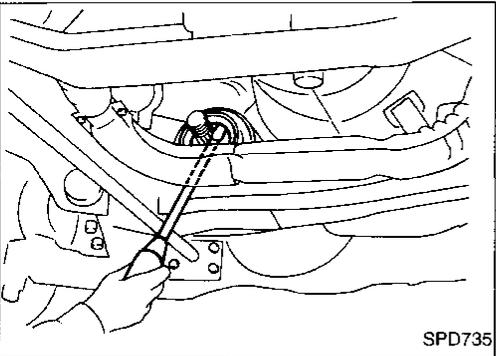
5. Apply multi-purpose grease to cavity at sealing lips of oil seal. Press front oil seal into carrier.
