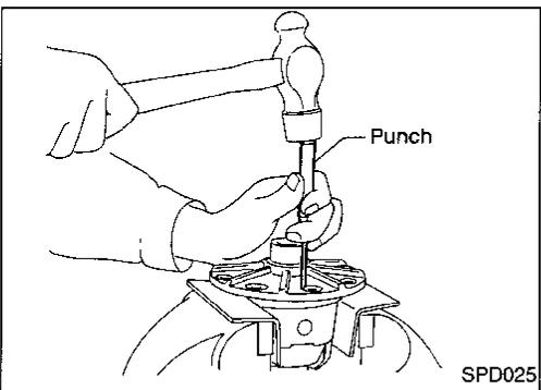
4. Punch off pinion mate shaft lock pin from ring gear side.
