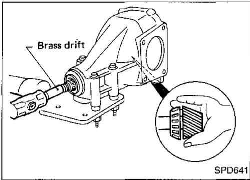
10. Take out drive pinion together with pinion rear bearing inner cone, drive pinion bearing spacer and pinion bearing adjusting washer.
