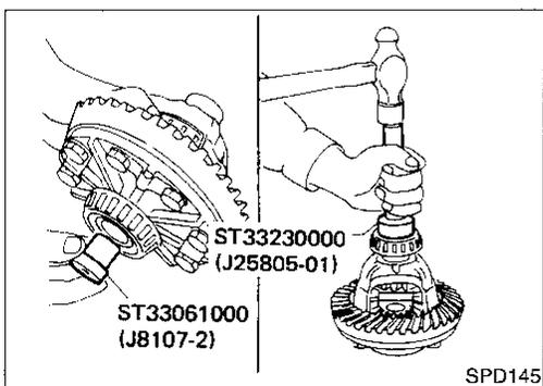
4. Reinstall the carrier side bearing using Tools J25805-01 and J8107-2. Press on the bearings.
