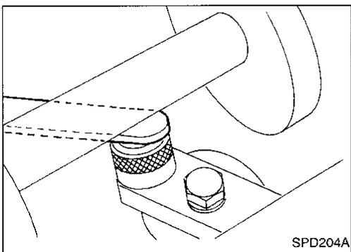
10. Select the correct standard pinion height adjusting washer thickness using a standard gauge of 2.5, 3.0, or 3.5 mm (0.098, 0.118, or 0.138 in) and J34309-101 feeler gauge. Measure the distance between the J34309-12 "H233B" pinion height adapter and the arbor.
