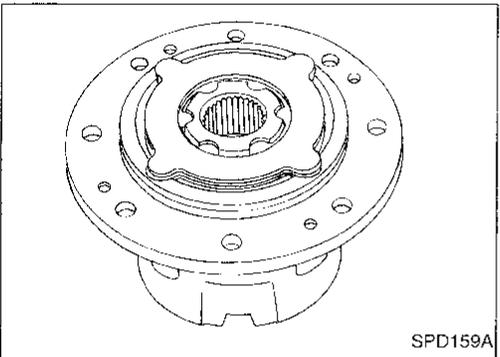
10. Install side gear thrust washer to differential case B.
