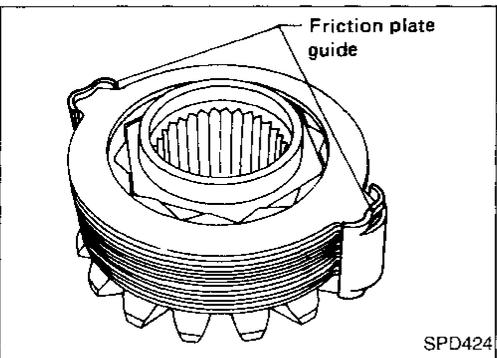
4. Install friction plate guides.
