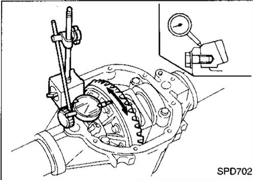
18. Check runout of ring gear with a dial indicator.
