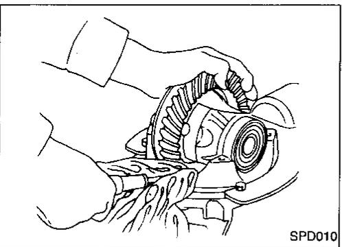
4. Remove differential case assembly with a pry bar.
