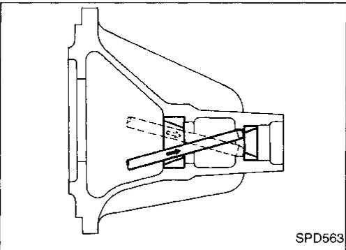
10. Remove front oil seal and pinion front bearing inner cone.
