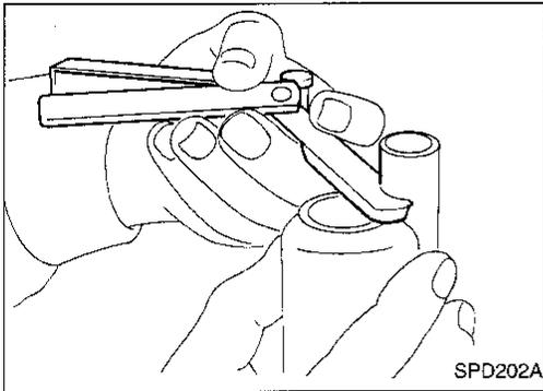
9. Select the correct thickness of pinion bearing preload adjusting washer using a standard gauge of 6 mm (0.24 in) and J34309-101 feeler gauge. The exact total measure you get with the gauges is the thickness of the adjusting washer required. Select the correct washer.
