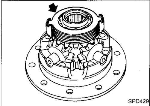
8. Install side gear to pinion mate gears.
