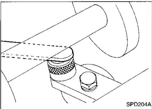
13. Select the correct standard pinion height adjusting washer thickness using a standard gauge of 3 mm (0.12 in) and J34309-101 feeler gauge. Measure the distance between the J34309-10 "R180A" pinion height adapter and the arbor.
