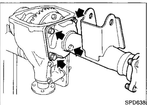
2. Remove extension tube and differential side shaft assembly.
