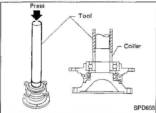
3. Install extension tube retainer, rear axle bearing and rear axle shaft bearing collar on differential side shaft.
