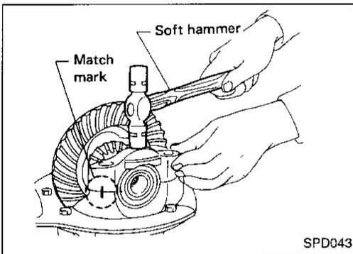
11. Align mark on bearing cap with that on gear carrier and install bearing cap on gear carrier.
