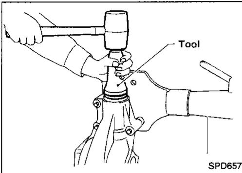
4. Place pinion front bearing inner cone in final drive housing.
