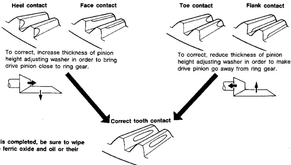
When adjustment is completed, be sure to wipe off completely the ferric oxide and oil or their equivalent.
