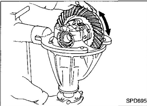
Usually the pattern will be correct if you have calculated the shims correctly and the backlash is correct. However, in rare cases you may have to use trial-and-error processes until you get a good tooth contact pattern. The tooth pattern is the best indication of how well a differential has been set up.
