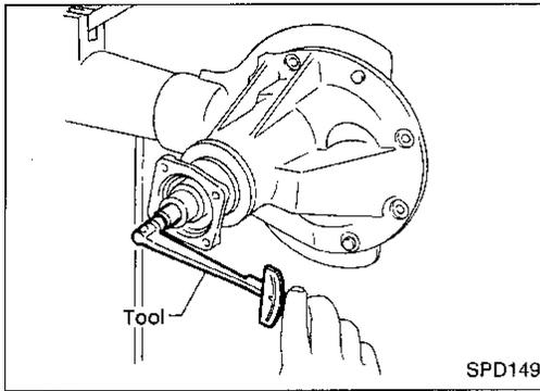
9. Tighten pinion nut by degrees to the specified preload while checking the preload with Tools.
