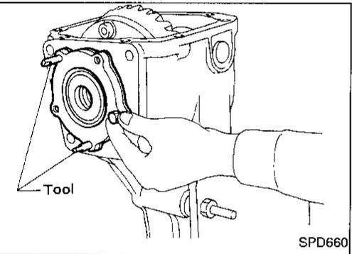
12. Install side oil seal to side retainer.
