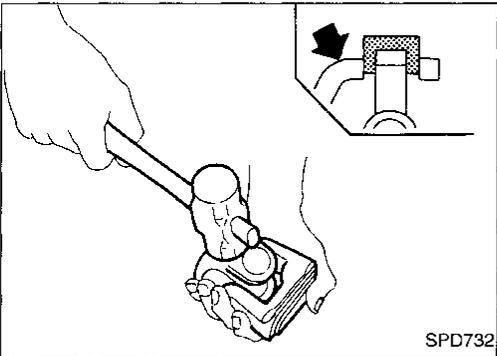
4. Remove bearing at opposite side in above operation. Put marks on disassembled parts so that they can be reinstalled in their original positions.
