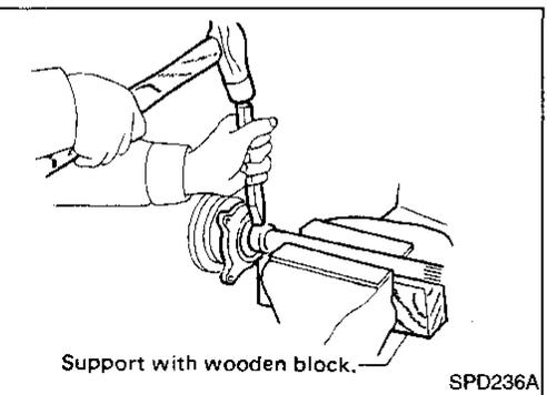
2. Cut rear axle bearing collar with cold chisel. Be careful not to damage differential side shaft.
