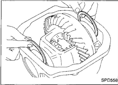
12. Insert left and right side bearing adjusting washers in place between side bearing and carrier.
