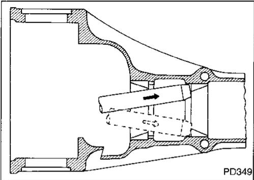
10. Remove pinion rear bearing inner cone and pinion height adjusting washer.
