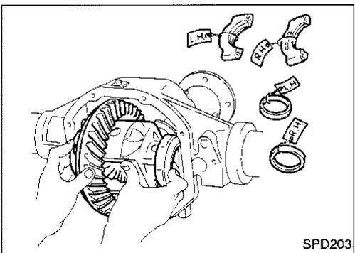
10. Select side bearing adjusting washer. Refer to Adjustment.
