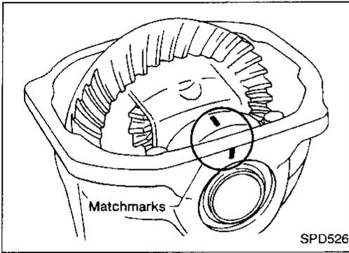
5. Install the side bearing caps in their correct locations and torque the bearing cap retaining bolts.
