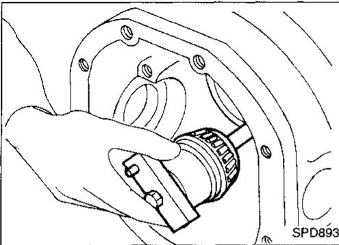
3. Place the pinion preload shim selector tool gauge screw, J34309-1, with the pinion rear bearing inner cone installed, into the final drive housing.
