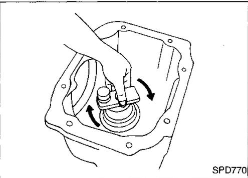
5. Turn the assembly several times to seat the bearings.
