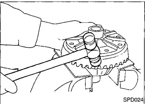
3. Tap ring gear off differential case with a soft hammer. Tap evenly all around to keep ring gear from binding.
