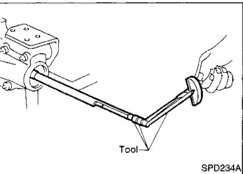
6. Measure the turning torque at the end of the J34309-2 shaft using Tool.
