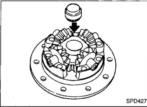
7. Install side gear to pinion mate gears.
