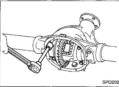
4. Remove differential case assembly with pry bar.
