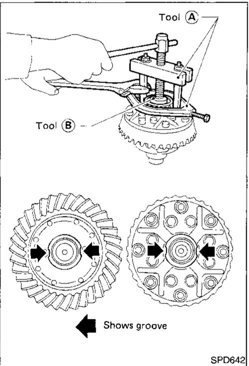
1. Remove side bearing inner cones.
