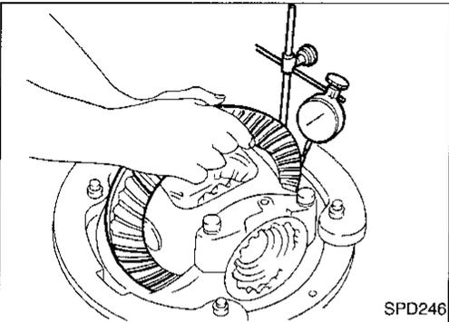
13. Tighten both right and left side bearing adjusters alternately and measure ring gear backlash and total preload at the same time. Adjust right and left side bearing adjusters by tightening them alternately so that proper ring gear backlash and total preload can be obtained.
