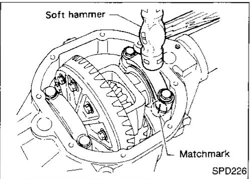
14. Align mark on bearing cap with that on gear carrier and install bearing cap on gear carrier.
