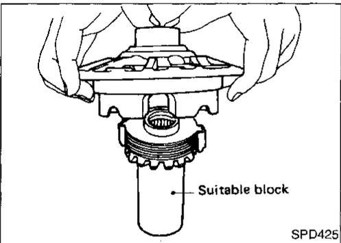
5. Install pinion mate gears and pinion shaft to differential case B.
