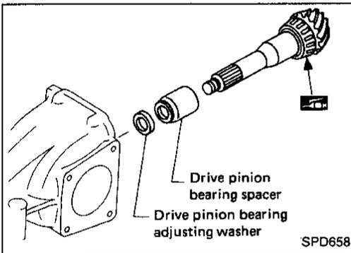
6. Place drive pinion bearing spacer, pinion bearing adjusting washer and drive pinion in final drive housing.
