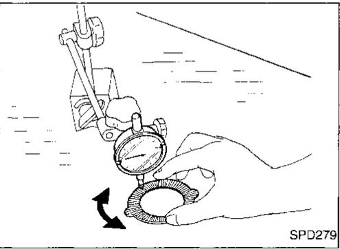
3. Check friction discs or plates for warpage.
