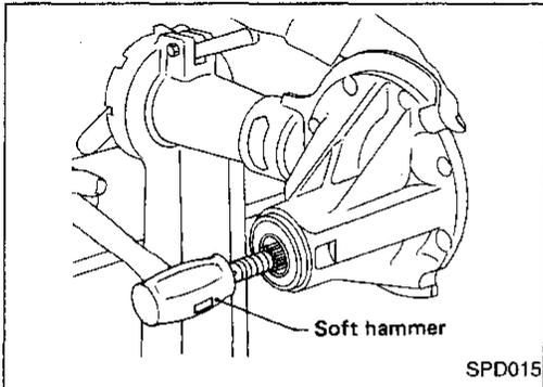
9. Remove pinion bearing outer races with a brass drift.
