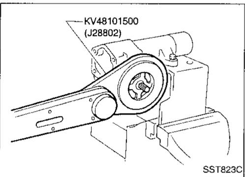
4. Loosen adjusting plug lock nut using Tool.
