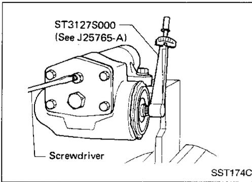
4. Adjust steering gear turning torque in a straight-ahead position using Tool, then lock with lock nut.
