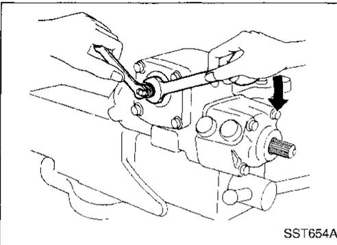
2. Tighten adjusting screw lock nut with tools.
