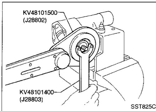
5. Tighten lock nut using Tools.
