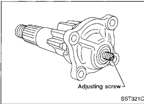
8. Remove lock nut, then loosen adjusting screw using a screwdriver. Separate sector cover and sector shaft.
