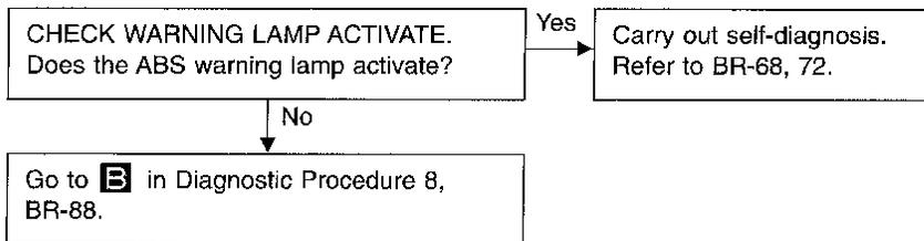
**Note: ABS does not work when vehicle speed is under 10 km/h (6 MPH).**
