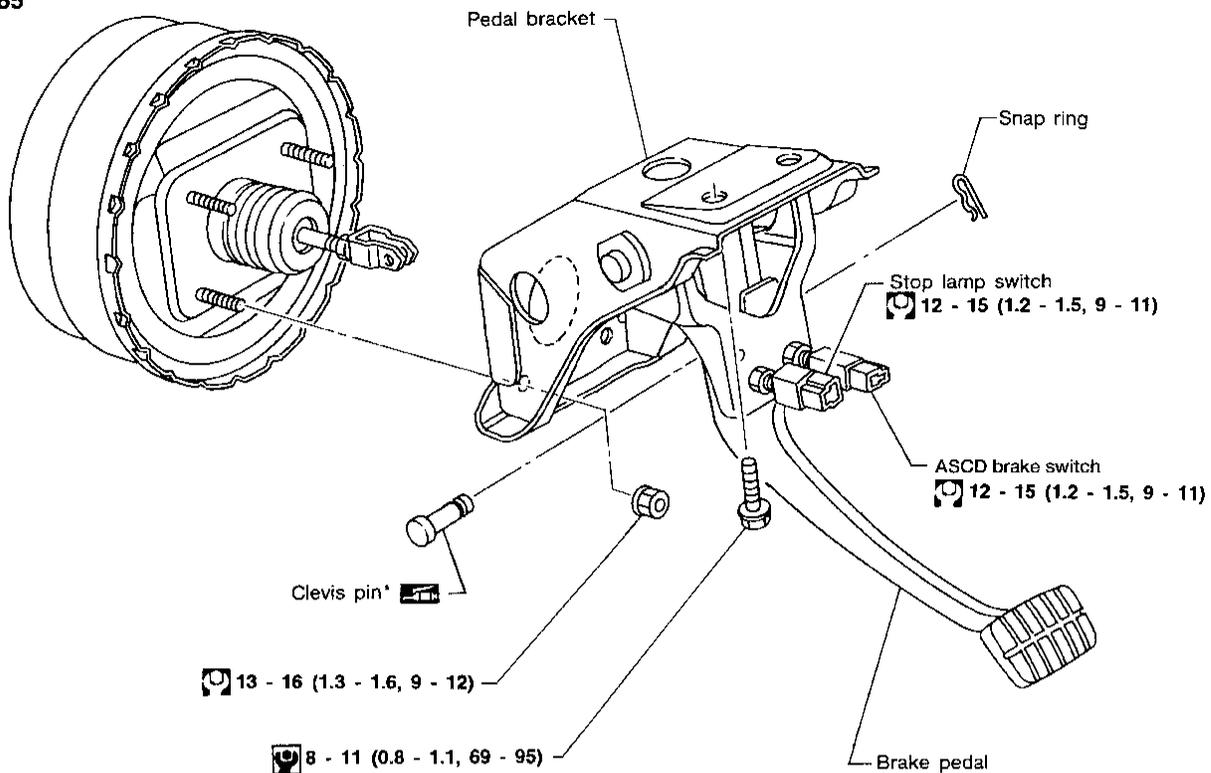
\* Replace plastic stopper located at the end of clevis pin if deformed or damaged.
