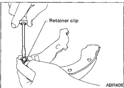
5. Remove retainer clip with a suitable tool. Then separate toggle lever and brake shoe.
