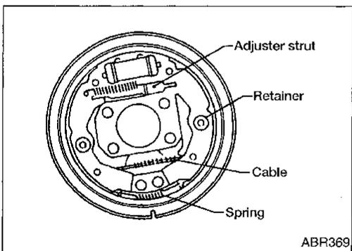
2. After removing retainer, remove spring by rotating shoes.
