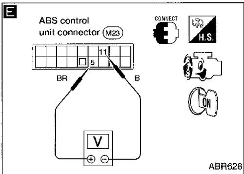
Main Power Supply and Ground Circuit Check
