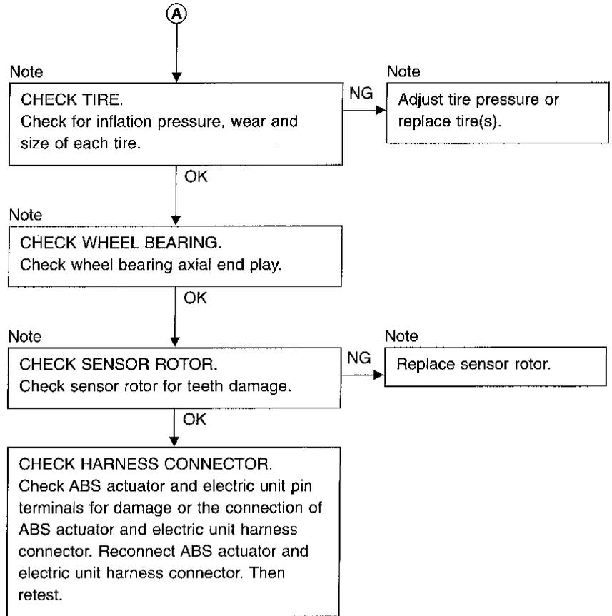
Note: Wheel position should be distinguished by code numbers except code No. 18 (sensor rotor).
