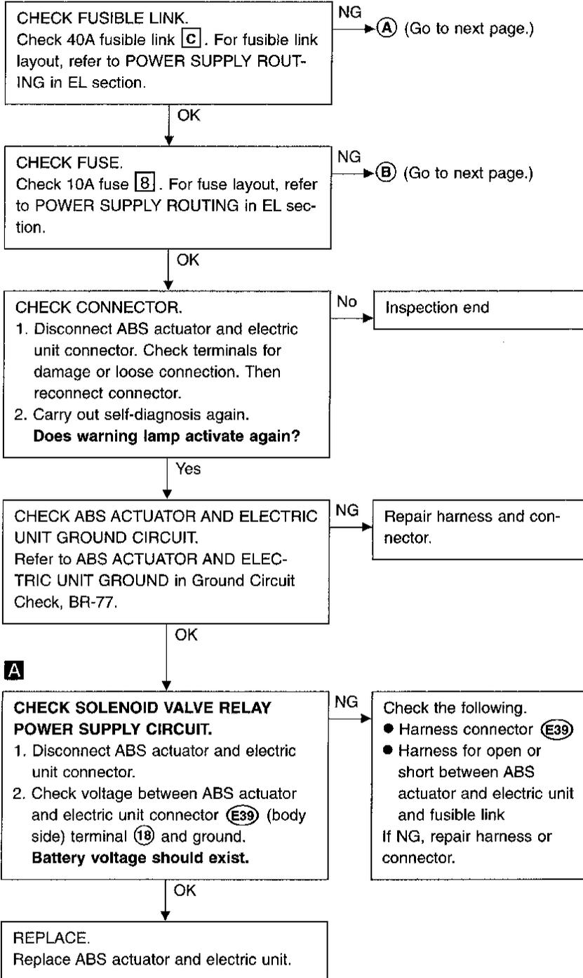
Diagnostic Procedure 2 (ABS actuator solenoid valve and solenoid valve relay) (Cont'd)
