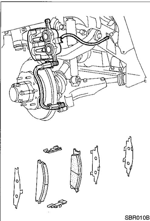
3. Open cylinder body upward. Then remove pad retainers, return spring and inner and outer shims.
