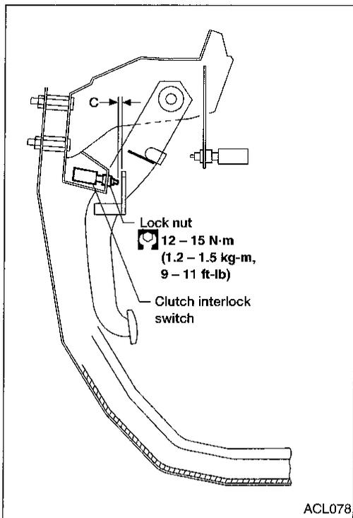
4. Adjust clearance "C" shown in the figure while fully depressing clutch pedal.
