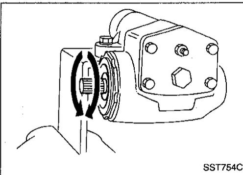
5. Turn worm gear several times by hand to properly break in worm bearing.
