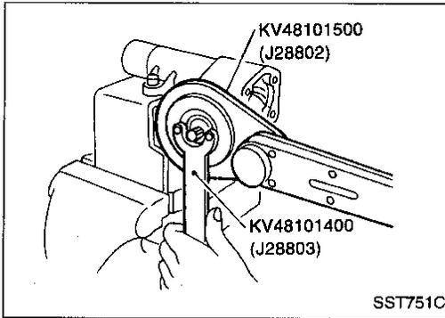
5. Tighten lock nut using Tools.
