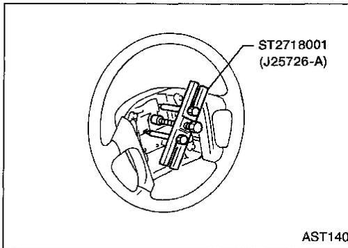
3. Remove steering wheel using Tool.
