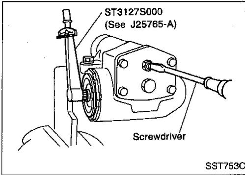
4. Adjust steering gear turning torque in a straight-ahead position using Tool, then lock with lock nut.
