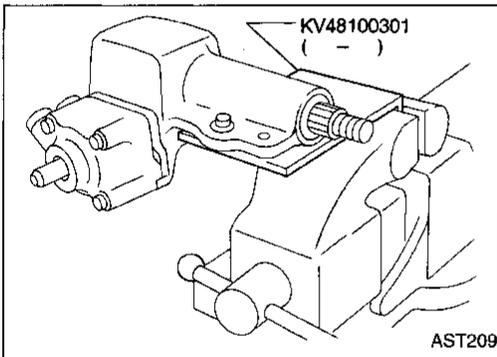
**TURNING TORQUE MEASUREMENT**
