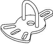
Removing rear axle shaft<br>NT159                      |
