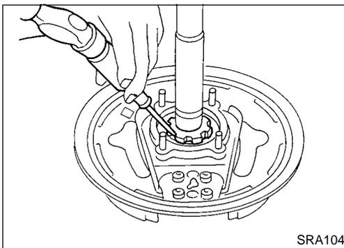
7. Unbend lock washer with a screwdriver.
