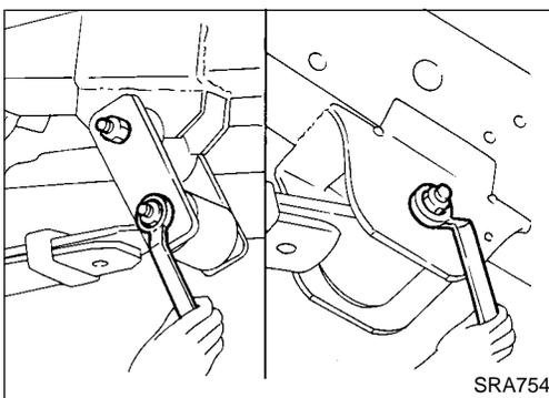
7. Tighten spring shackle nuts, front pin nuts and shock absorber nuts.
