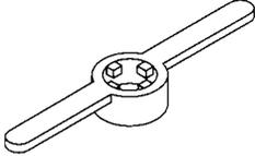
Removing wheel bearing lock nut<br>NT160             |
