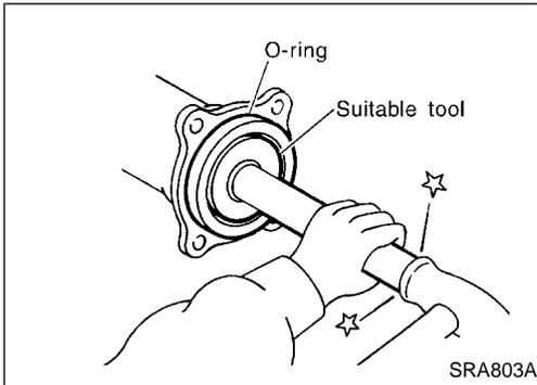
7. Install new oil seal to rear axle housing using a suitable tool.
