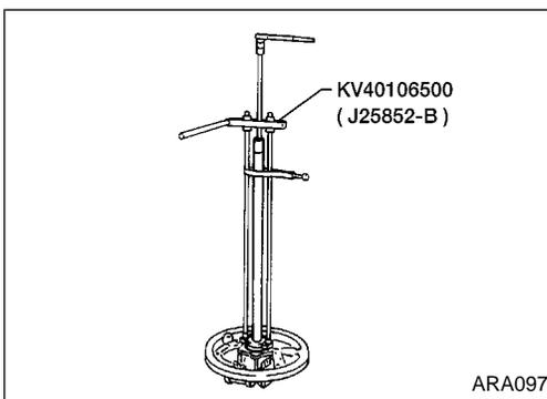
6. Remove ABS sensor rotor.
