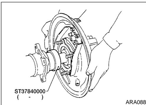
10. Position axle shafts in rear axle housing with Tool as a guide.
