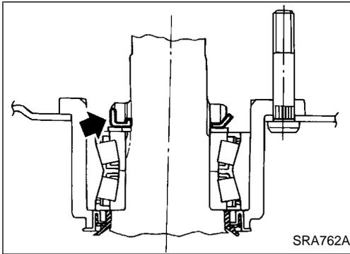
4. Install plain washer and a new wheel bearing lock washer.
