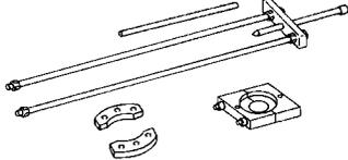
Removing wheel bearing and ABS sensor rotor<br>NT683 |
