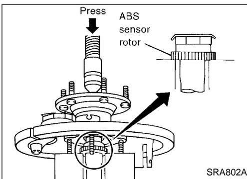
9. Press ABS sensor rotor onto axle shaft until it contacts wheel bearing lock nut.
