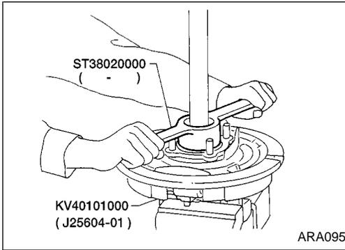
9. Remove wheel bearing together with bearing cage and baffle plate from axle shaft.
