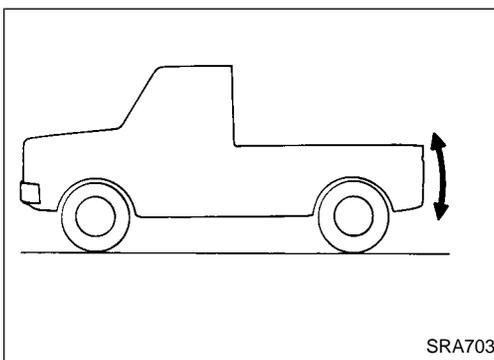
6. Remove stands and bounce the vehicle to stabilize suspension. (Unladen)
