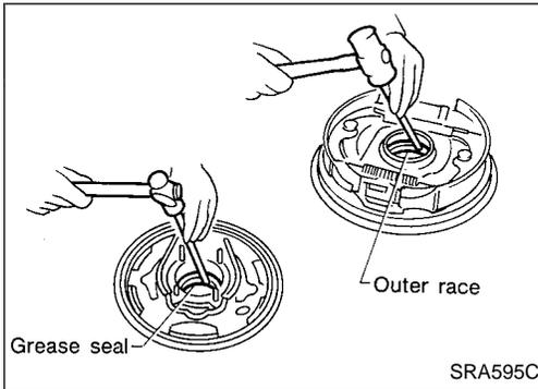
11. Remove wheel bearing assembly.
