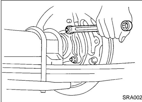
1. Disconnect parking brake cable and brake tube.
