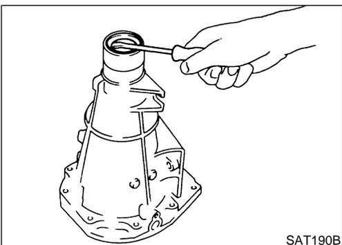
c. Remove oil seal from rear extension case.
