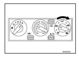
Confirm that discharge air comes out according to the air distribution table at left. Refer to MTC-23, "Discharge Air Flow".
