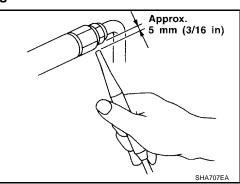
2. When testing, circle each fitting completely with probe.
