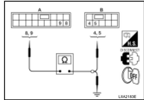
3. Check continuity between main power window and door lock/unlock switch and ground.
