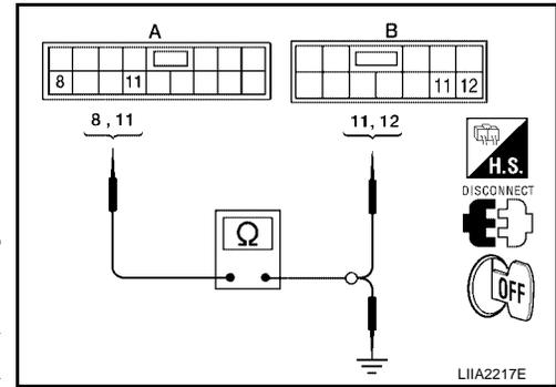
4. Check continuity between main power window and door lock/unlock switch connector and ground.
