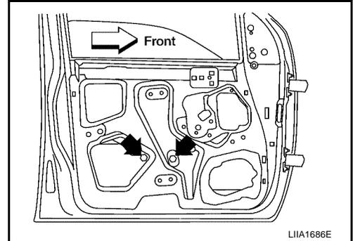
7. While holding the door window, raise it at the rear and pull the glass out of the sash toward the outside of the door.
