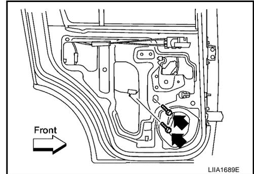
6. Raise the rear door glass and hold it in place with suitable tool.
