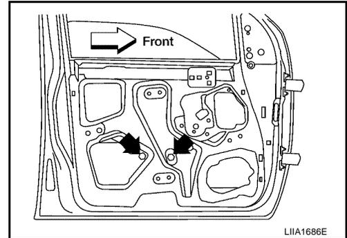
7. Raise the front door glass and hold it in place with suitable tool.
