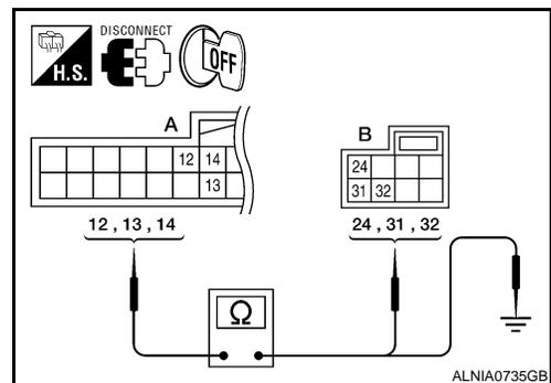
3. Check continuity between Bluetooth control unit connector B141 (A) and ground.
