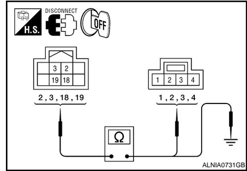
3. Check continuity between audio amp. harness connector B158 (A) and ground.
