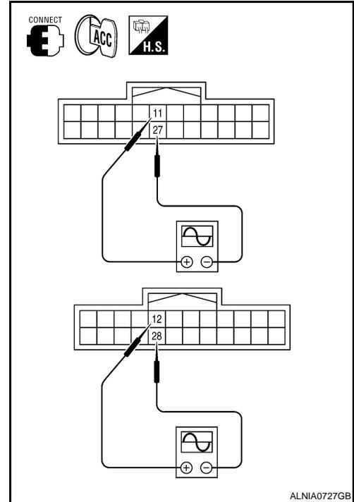
Are audio signal voltage readings as specified?
