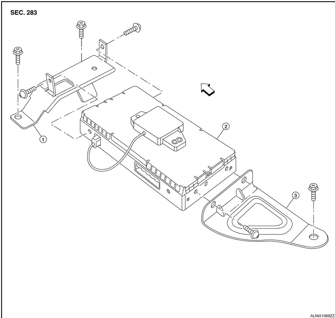
1. Bluetooth control unit front bracket    2. Bluetooth control unit/antenna    3. Bluetooth control unit rear bracket
