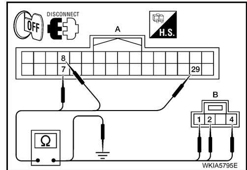
4. Check continuity between Bluetooth control unit harness connector B141 (A) and ground.
