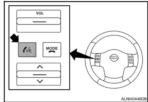
4. While the prompt is playing, press and hold the steering wheel audio control switch
