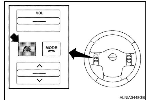
4. While the prompt is playing, press and hold the steering wheel audio control switch
