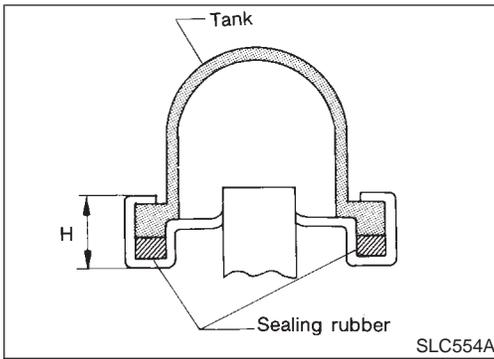
5. Make sure that the rim is completely crimped down.
