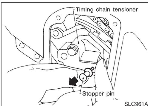
6. Install timing chain tensioner, then remove the stopper pin.
