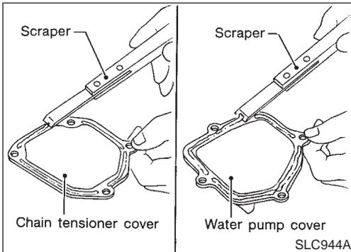
3. Before installing, remove all traces of liquid gasket from mating surface of water pump cover and chain tensioner cover using a scraper. Also remove traces of liquid gasket from mating surface of front cover.
