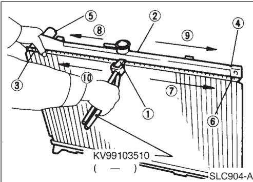
4. Caulk tank in specified sequence with Tool.
