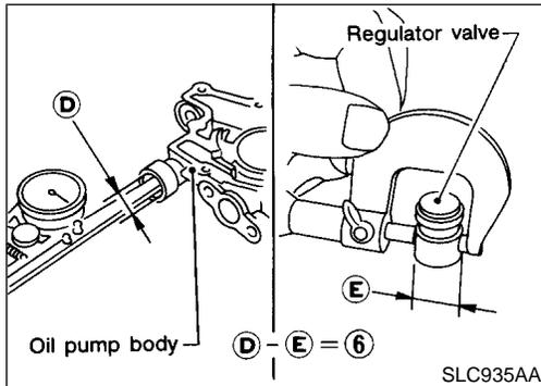
4. Check regulator valve to oil pump body clearance.
