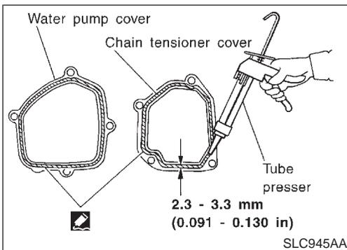
4. Apply a continuous bead of liquid gasket to mating surface of chain tensioner cover and water pump cover.
