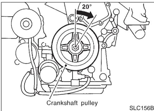
5. Return the crankshaft pulley to its original position by turning it 20° forward.
