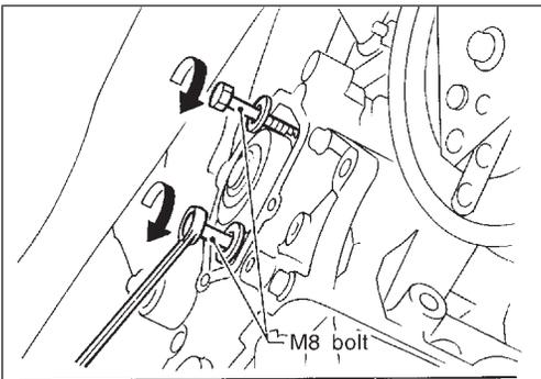
9. Tighten M8 bolts by turning half turn alternately until they reach timing chain rear case.
