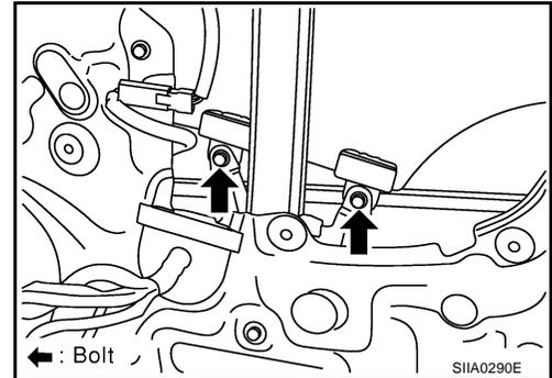
6. Remove the bolts and the regulator and guide channel from the panel.
