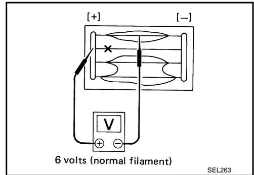
3. If a filament is burned out, circuit tester registers 0 or battery voltage.
