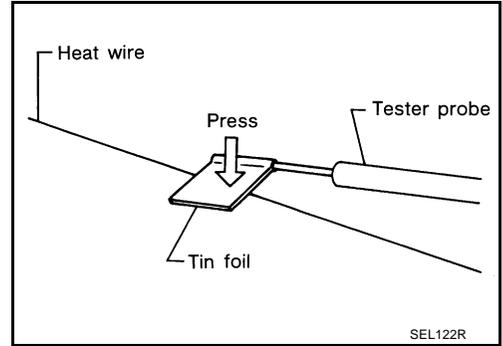
2. Attach probe circuit tester (in Volt range) to middle portion of each filament.
