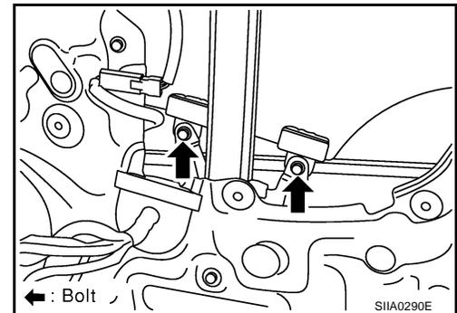
5. Remove the partition sash from the glass run.
