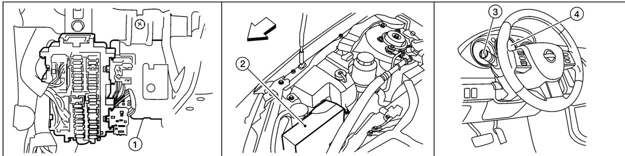
1. BCM M18, and M20 (View with instrument panel removed)
