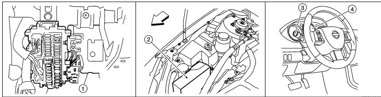
1. BCM M18 and M20 (View with instrument panel removed)
