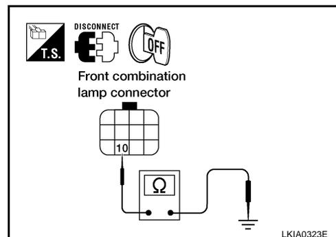
3. Check continuity between license lamp plate harness connector and ground.
