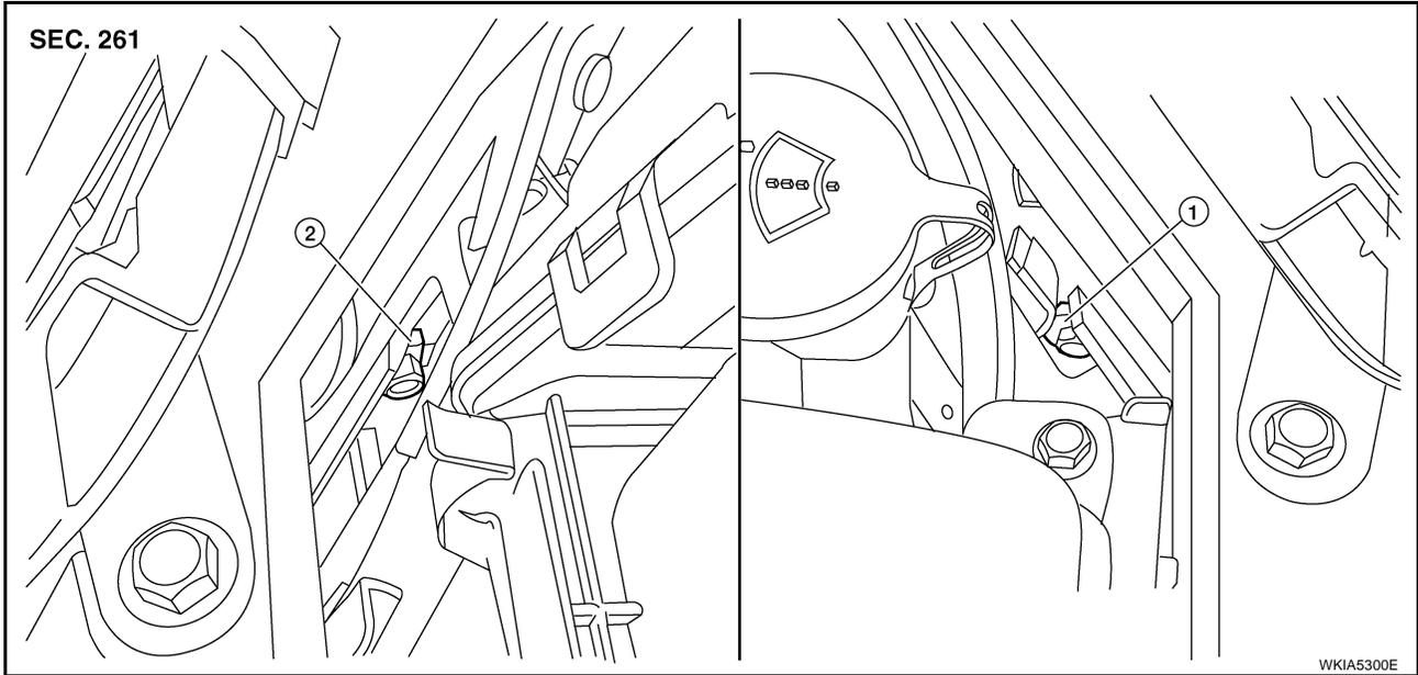
1. Passenger side adjustment screw    2. Driver side adjustment screw
