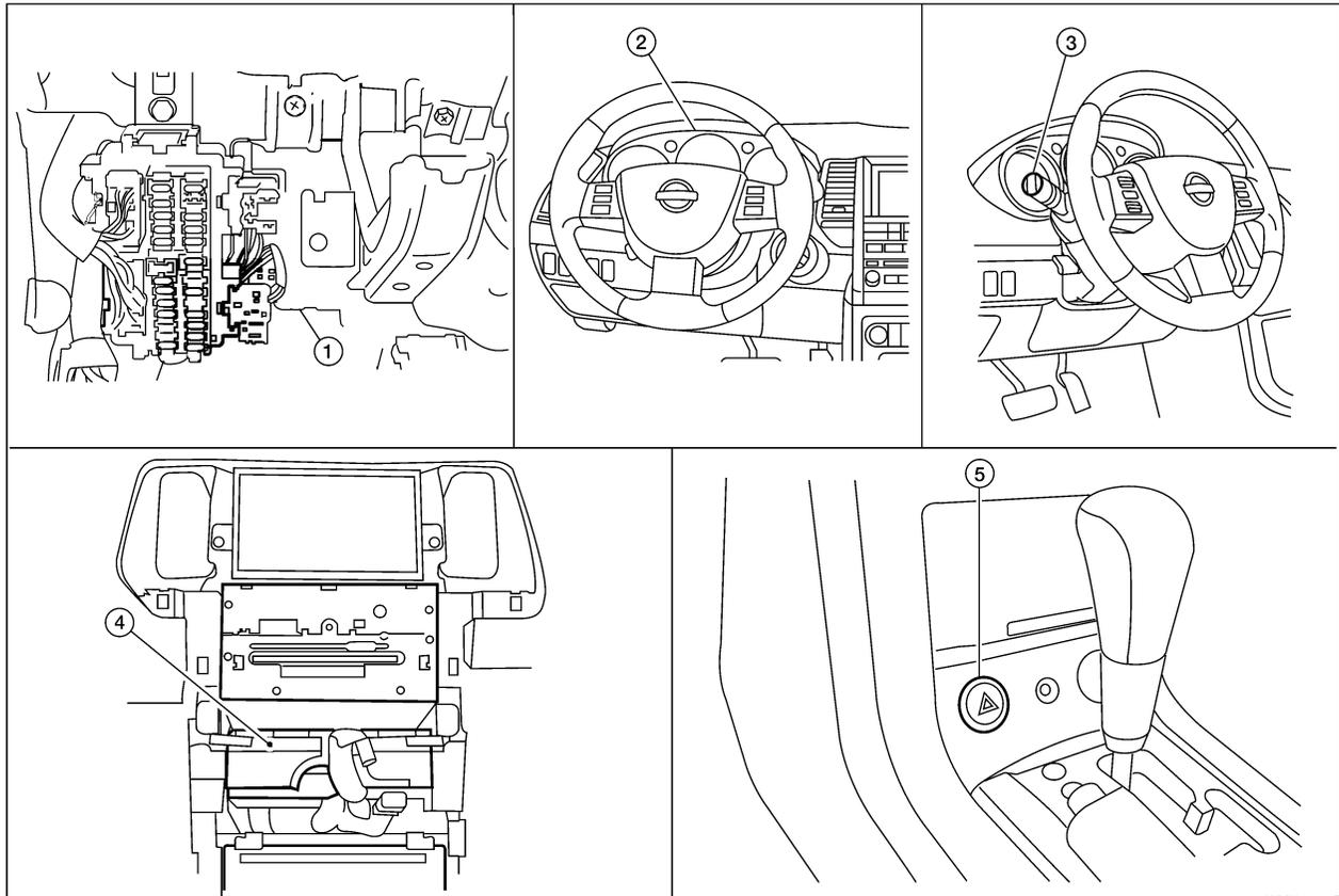
1. BCM M18 and M20 (View with instrument panel removed)
