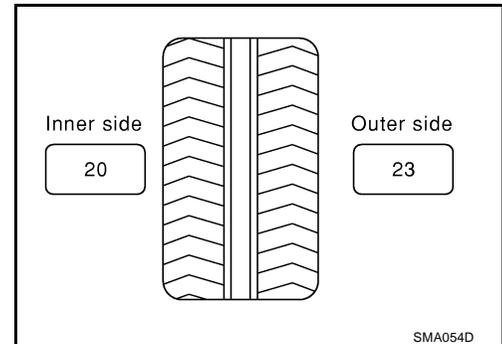
Indicated unbalance value  $\times 5/3$  = balance weight to be installed
