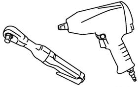
PBIC0190E <p>Removing wheel nuts</p> |
