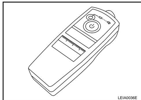
5. Register the IDs in order from FR LH, FR RH, RR RH and RR LH. When ID registration of each wheel has been completed, a buzzer sounds and the hazard warning lamps flash.
