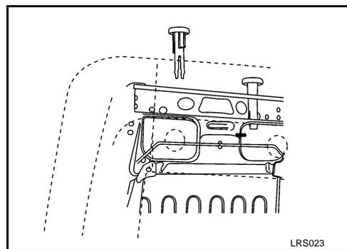
3. Pull out the harness connector for the side air bag from the seat cushion.
