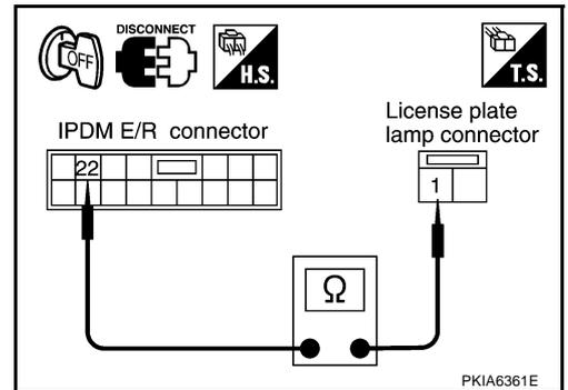
5. Check continuity between IPDM E/R harness connector and rear combination lamp harness connector.
