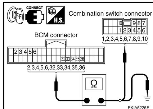
4. Check for continuity between each terminal of BCM harness connector in suspect malfunctioning system and ground.
