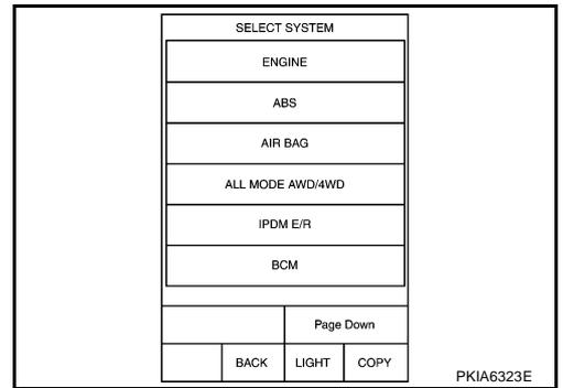
4. Select the desired part to be diagnosed on "SELECT SYSTEM" screen.
