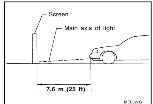
3. Adjust front fog lamps using adjusting screw so that the top edge of the high intensity zone is in the hatched area as shown in the figure.
