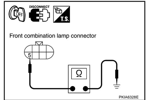
2. Check continuity between license plate lamp harness connector and ground.
