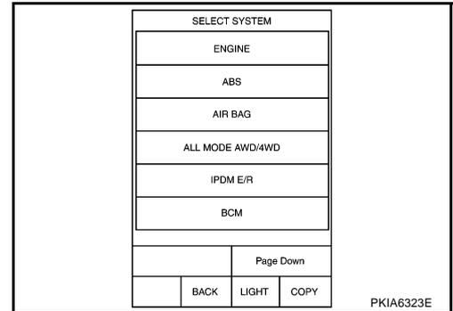
4. Select the desired part to be diagnosed on "SELECT SYSTEM" screen.
