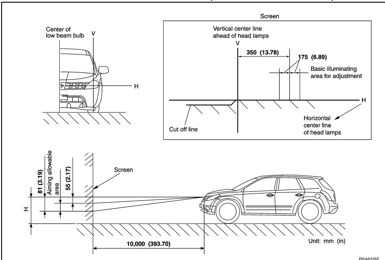
If the vehicle front body has been repaired and/or the headlamp assembly has been replaced, check aiming. Use the aiming chart shown in the figure.
