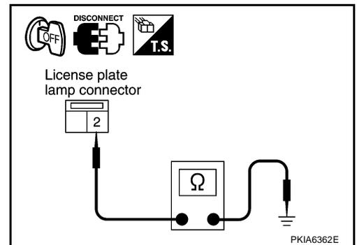
3. Check continuity between rear combination lamp harness connector and ground.
