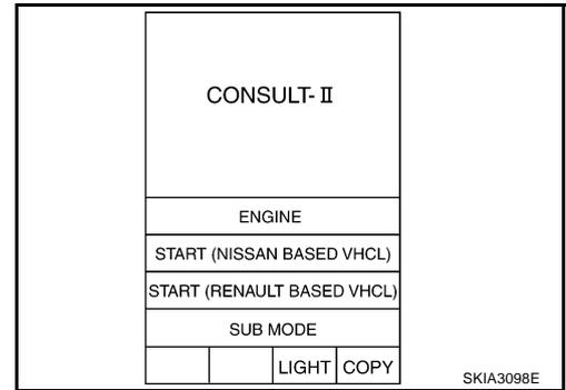
3. Touch "IPDM E/R" on "SELECT SYSTEM" screen. If "IPDM E/R" is not displayed, print "SELECT SYSTEM" screen, then refer to [GI-39, "CONSULT-II Data Link Connector \(DLC\) Circuit"](#).
