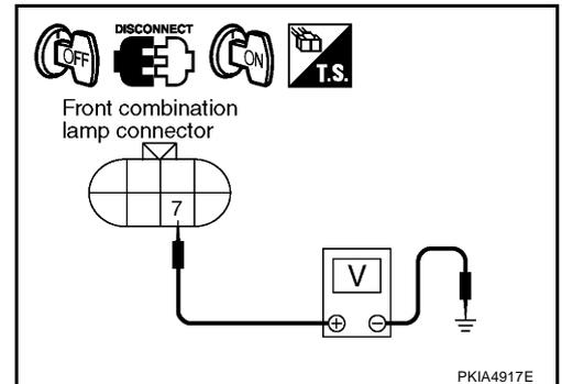
5. Check voltage between license plate lamp connector and ground.
