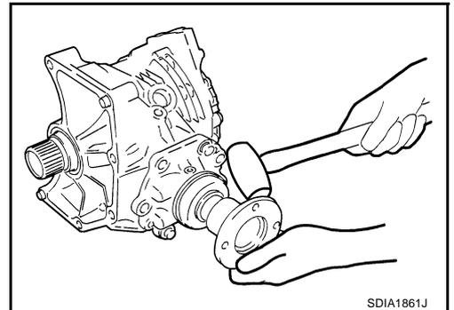
5. Using a drift, remove drive pinion assembly from pinion sleeve with a press.
