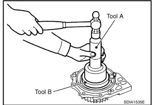
4. Using a drift, drive the adapter case oil seal until it becomes flush with the case end.
