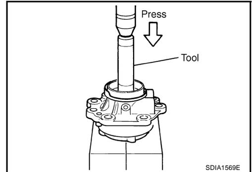
4. Using a drift, install the pinion front bearing outer race.
