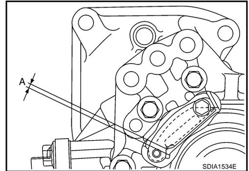
4. Using a drift, drive the transfer case oil seal until it becomes flush with the case end.
