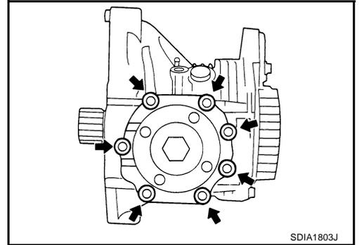
2. Using a plastic hammer, tap companion flange to remove pinion sleeve assembly.
