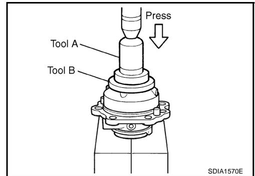
5. Apply gear oil to pinion front bearing inner race and mating position on the drive pinion. Using a drift, install pinion front bearing inner race to the drive pinion.
