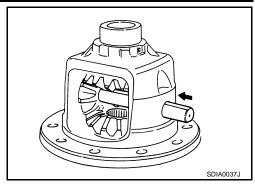
Measure side gear end play following the procedure below, and select the appropriate side gear thrust washers.
