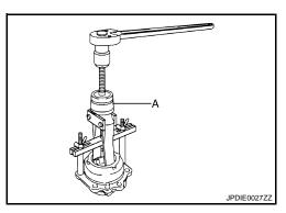
14. Using the replacer (A) (commercial service tool), press the pinion front bearing inner race out of the drive pinion.
