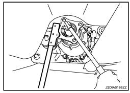
8. Remove coupling cover with electric controlled coupling from final drive assembly.
