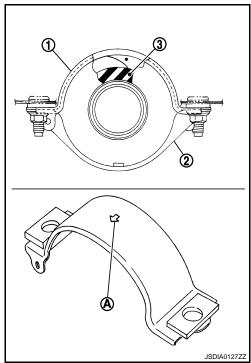
After tightening the bolts and nuts to the specified torque, check that the bolts (3) on the flange side is tightened as shown in the figure.
