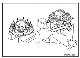
7. Remove side bearing inner races, using pullers and the drift [SST: ST33052000 ( — )].
