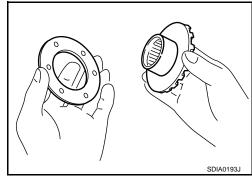
3. Align 2 pinion mate gears in diagonally opposite positions, then rotate and install them into differential case after installing pinion mate thrust washers to pinion mate gears.
