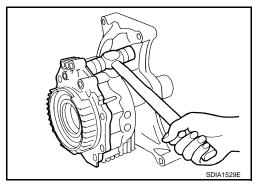
4. Remove adapter case oil seal with a suitable tool.
