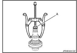
7. Lightly tap adapter case with a plastic hammer to remove drive gear from the gear ring.
