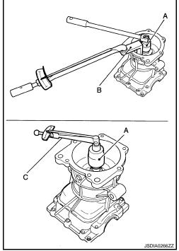
e. Apply gear oil to side bearings, and install new side bearing adjusting shims with the same thickness or re-install the old ones to the same mounting position they were in prior to disassembly. Set the drifts [SST: KV40100610 (J-26089)] to the right and left. Install differential case assembly to gear carrier.
