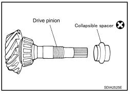
Apply gear oil to pinion front bearing, and assemble pinion front bearing inner race to drive pinion. Using the drifts and stand, press pinion front bearing inner race to drive pinion as far as drive pinion nut can be tightened.
