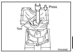
2. Press pinion front bearing outer race into gear carrier, using the drift [SST: 33230000 (J-25805-01)].
