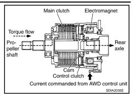
Transmission torque to the rear wheels is determined according to command current.
