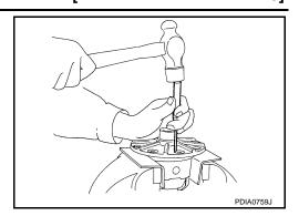
Remove pinion mate shaft, pinion mate gears, pinion mate thrust washers, side gears, side gear thrust washers from differential case.
