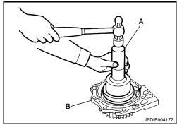
4. Using the drift (A) [SST: KV38101700 ( — )], drive the adapter case oil seal until it becomes flush with the case end.
