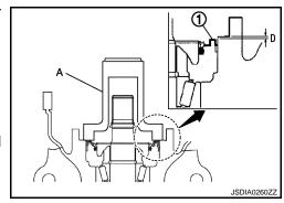
Connect AWD solenoid harness to electric controlled coupling.
