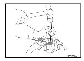
7. Press side bearing inner races to differential case, using the drift [SST: KV40105020 ( — )].
