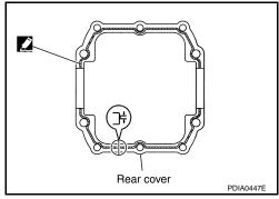
15. Set the drifts [SST: KV40100610 (J-26089)] to the right and left side bearing adjusting shims individually. Compress differential case assembly and side bearing to install rear cover.
