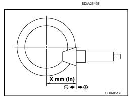
• If the tooth contact is near the face (face contact), or near the heel (heel contact), thicken drive pinion gear adjusting shim to move drive pinion closer to drive gear.
