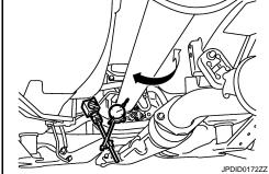
Check runout again. If runout still exceeds specifications, replace propeller shaft assembly.
