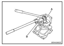
Press drive pinion assembly out of gear carrier.
