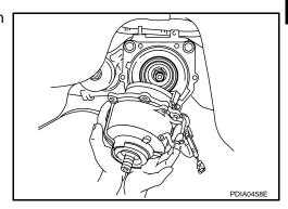
11. Remove front oil seal from coupling cover, using a suitable tool.
