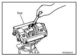
4. Rotate drive gear back and forth several times, check drive pinion gear to drive gear tooth contact.
