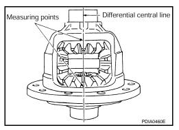
b. Using thickness gauges, measure the clearance between side gear back and differential case at 3 different positions, while rotating side gear. Average the 3 readings, and then decide the clearance. (Measure the clearance of the other side as well.)
