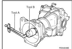
If measured value is out of the specification, disassemble it to check and adjust each part. Adjust the pinion bearing preload and side bearing preload.
