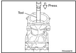
Press pinion rear bearing inner race to drive pinion, using the drift [SST: ST23860000 ( — )].
