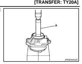
4. Install the pinion front bearing outer race with the drifts.
