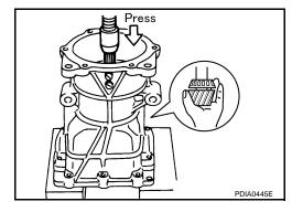
7. Remove pinion rear bearing inner race from drive pinion, using puller and bearing puller.
