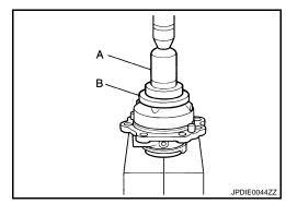
5. Install the pinion front bearing inner race to drive pinion with the drift (A) [SST: ST30901000 (J-26010-01)].
