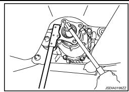
Remove front oil seal from coupling cover, using a suitable tool.
