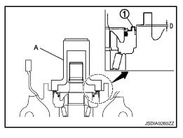
Connect AWD solenoid harness to electric controlled coupling.
