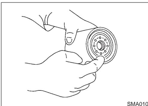
2. Clean oil filter mounting surface on cylinder block. Coat rubber seal of new oil filter with engine oil.
