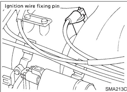
When installing spark plugs to No. 2 and 4 cylinders, securely fit each ignition wire mounting hole onto the ignition wire fixing pin.
