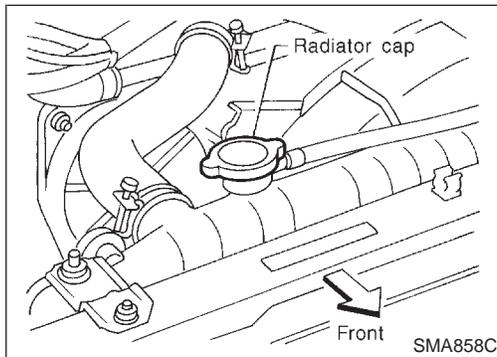
3. Remove radiator filler cap. Remove reservoir tank, drain coolant, then clean reservoir tank. Install it temporarily.
