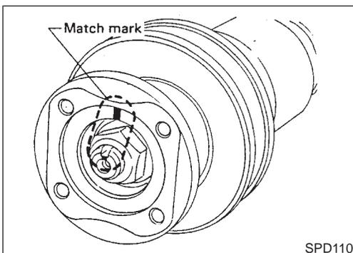
2. Put match marks on the flange and shaft. NAPD0007S01
