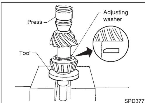
2. Select drive pinion height adjusting washer and pinion bearing adjusting washer. Refer to "PINION GEAR HEIGHT AND PINION BEARING PRELOAD", PD-26.
