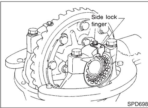
14. Tighten side bearing cap bolts.
