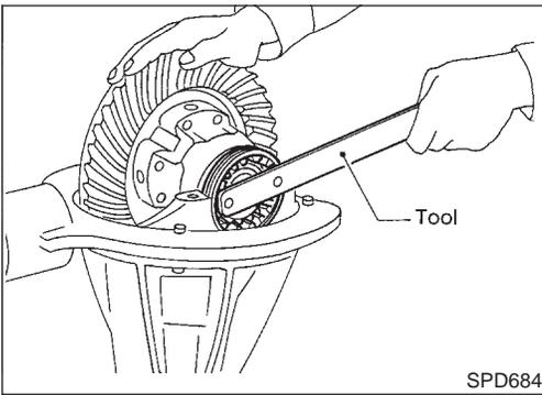
4. Remove side bearing adjuster with Tool.
