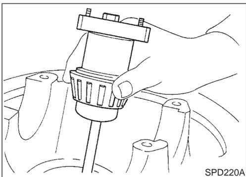
13. Remove the J34309 pinion preload shim selector tool from the final drive housing and disassemble to retrieve the pinion bearings.
