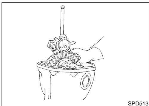
16. Measure ring gear to drive pinion backlash with a dial indicator.
