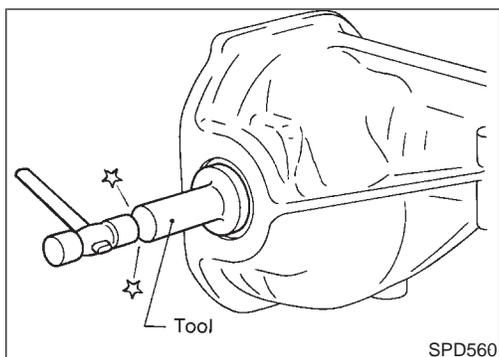
15. Apply multi-purpose grease to cavity at sealing lips of oil seal. Install side oil seal.
