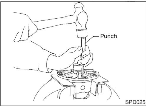
4. Drive out pinion mate shaft lock pin, with punch from ring gear side.
