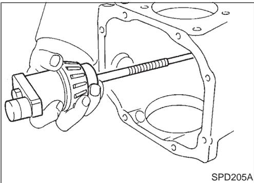
16. Remove the J34309 pinion preload shim selector tool from the final drive housing and disassemble to retrieve the pinion bearings.
