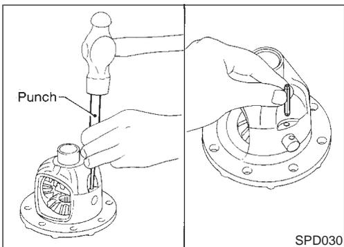
4. Install pinion mate shaft lock pin with a punch. **Make sure lock pin is flush with case.**
