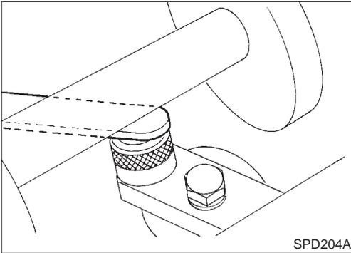
13. Select the correct standard pinion height adjusting washer thickness by using a standard gauge of 3.0 mm (0.118 in) and your J34309-101 feeler gauge. Measure the gap between the J34309-11 "R200A" pinion height adapter and the arbor.
