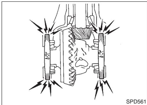
18. Recheck ring gear to drive pinion backlash because increase or decrease in thickness of shims will cause change of ring gear-to-pinion backlash.
