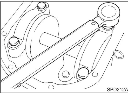
12. Install the side bearing caps and tighten the cap bolts.
