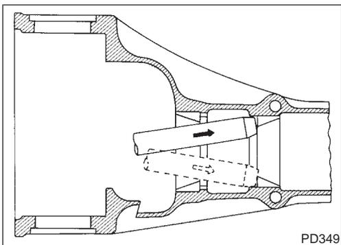
11. Remove pinion bearing outer races with a brass drift.
