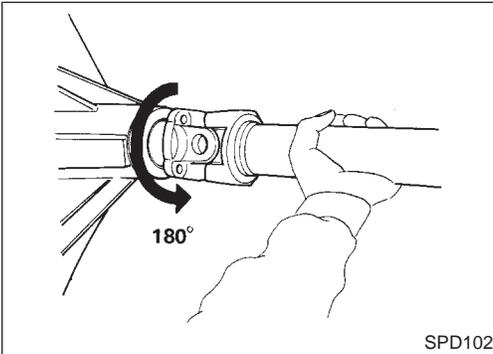
3. If runout exceeds specifications, disconnect propeller shaft at final drive companion flange; then rotate companion flange 180 degrees and reconnect propeller shaft.
