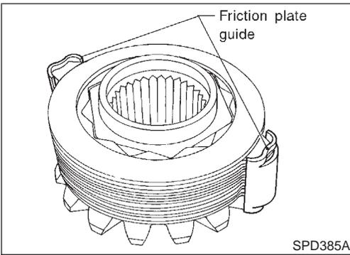
3. Install friction plate guides.
