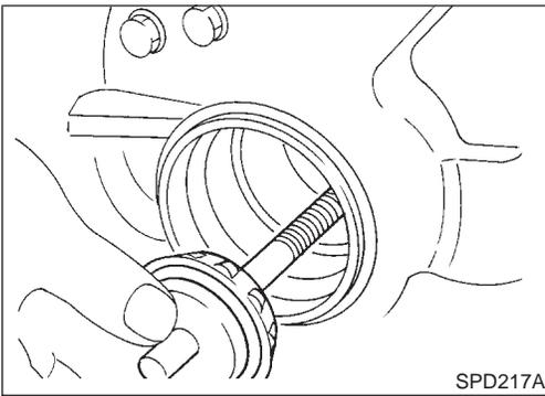
4. Install the J34309-2 gauge anvil with the front pinion bearing into the final drive housing and assemble it to the J34309-1 gauge screw. Make sure that the J34309-16 gauge plate will turn a full 360 degrees, and tighten the two sections by hand to set bearing pre-load.
