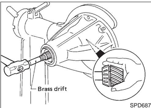
8. Take out drive pinion together with pinion rear bearing inner cone, drive pinion bearing spacer and pinion bearing adjusting shim.
