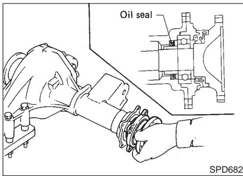
22. Install differential side shaft assembly.
