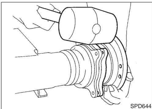
2. Remove differential side shaft assembly.
