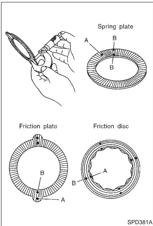
4. Measure frictional surfaces and projected portions of friction disc, friction plate, spring plate, and determine each part's differences to see if the specified wear limit has been exceeded. If any part has worn beyond the wear limit, and deformed or fatigued, replace it with a new one that is the same thickness as the projected portion.
