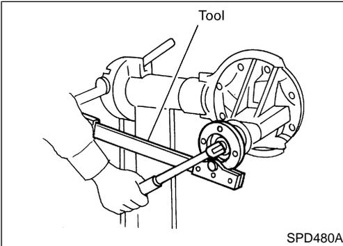
6. Remove drive pinion nut with Tool.
