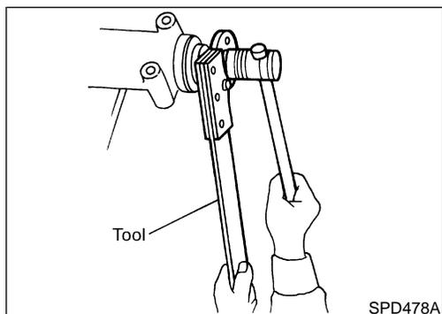
8. Tighten pinion nut to the specified torque. **The threaded portion of drive pinion and pinion nut should be free from oil or grease.**
