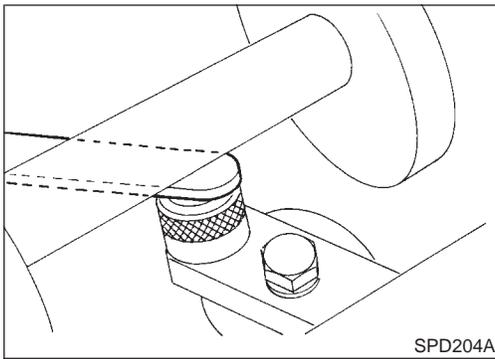
10. Select the correct standard pinion height adjusting washer thickness using a standard gauge of 2.5, 3.0, or 3.5 mm (0.098, 0.118, or 0.138 in) and your J34309-101 feeler gauge. Measure the distance between the J34309-12 "H233B" pinion height adapter and the arbor.
