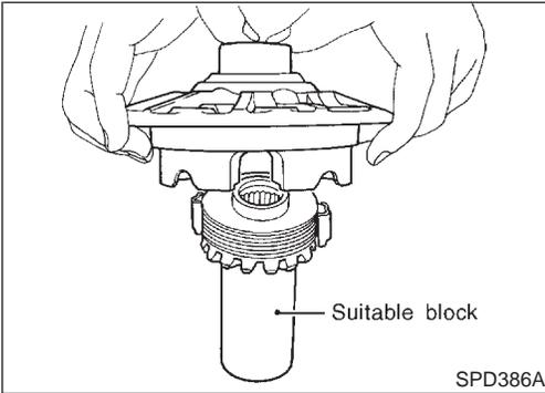
4. Install differential case B over side gear, discs, plates and friction plate guide assembly.
