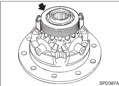
6. Install side gear to pinion mate gears.
