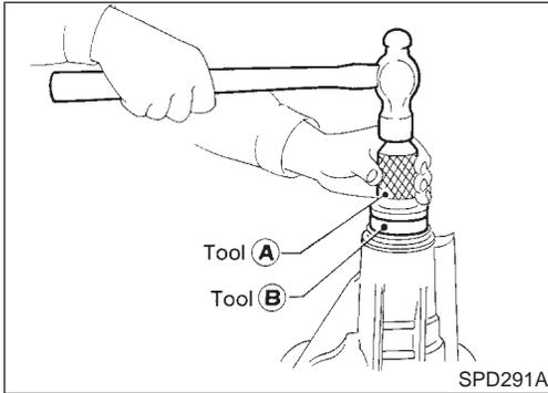
5. Apply multi-purpose grease to cavity at sealing lips of oil seal. Install front oil seal.
