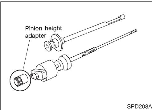
7. Place the J34309-12 "H233B" pinion height adapter onto the gauge plate and tighten it by hand.
