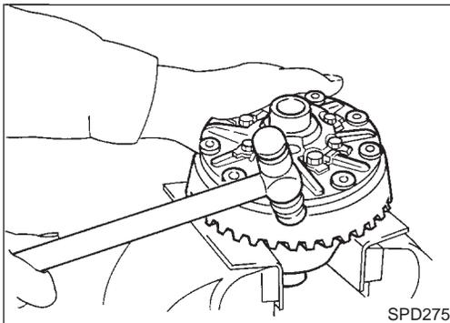
1. Remove side bearing inner cone with Tool.
