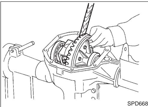
10. Remove the carrier from the final drive housing, saving the selected preload washers for later use during the assembly of the final drive unit.
