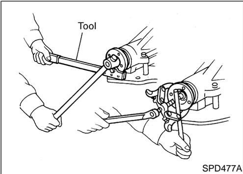
7. Loosen drive pinion nut.
