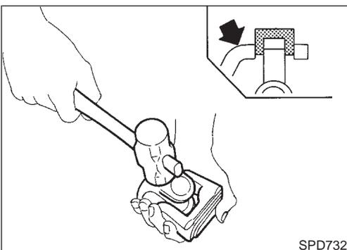
3. Remove pushed out journal bearing by lightly tapping yoke with a hammer, taking care not to damage journal and yoke hole.
