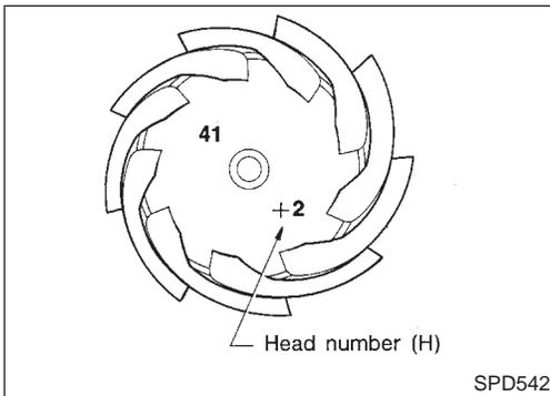
12. Correct the pinion height washer size by referring to the "pinion head height number".
