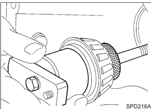
3. Place the pinion preload shim selector tool gauge screw assembly, J34309-1, with the pinion rear bearing inner cone installed, into the final drive housing.
