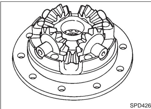
5. Install pinion mate gears and pinion mate thrust washers on pinion mate shaft, then install pinion mate shaft in differential case B.
