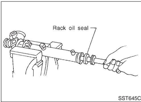
4. Install rack oil seal and rack bushing with rack assembly.
