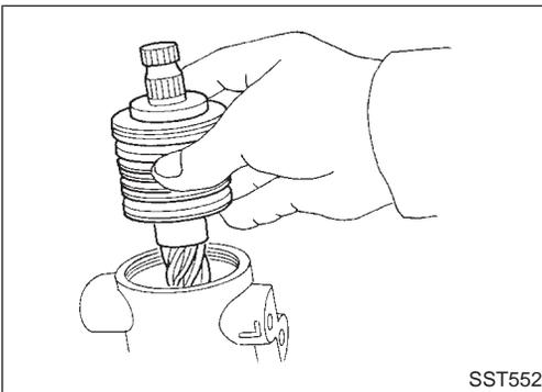
12. Install pinion assembly to rear housing.
