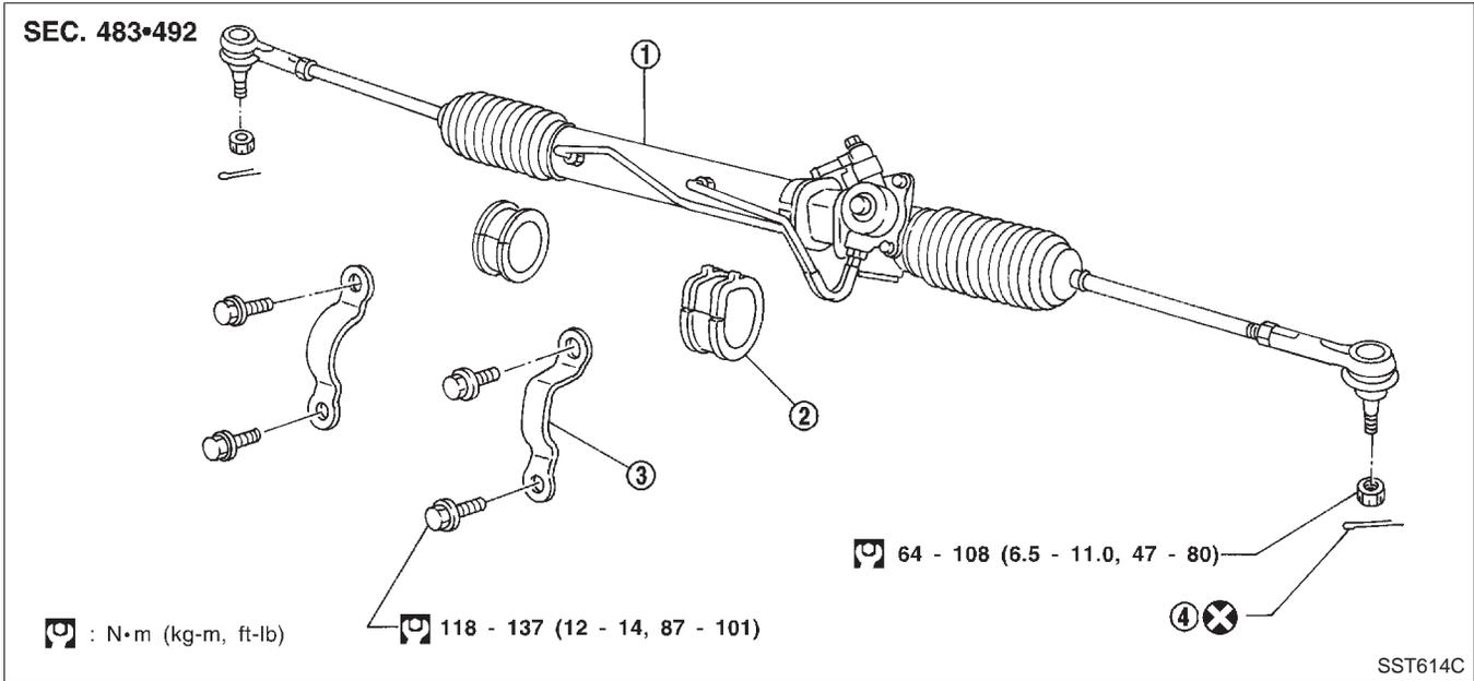
1. Gear and linkage assembly
