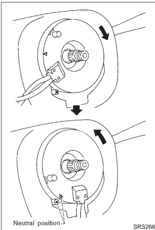
2. Align spiral cable correctly when installing steering wheel.
