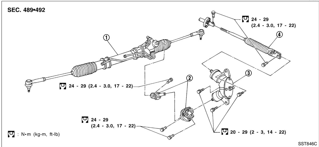
1. Power steering gear assembly
