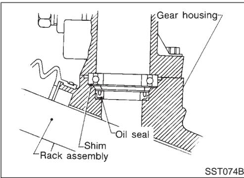
9. Install pinion bearing adjusting shim(s).
