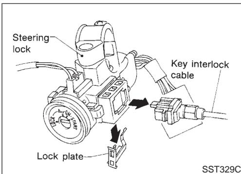
4. Remove key interlock cable (A/T models).
