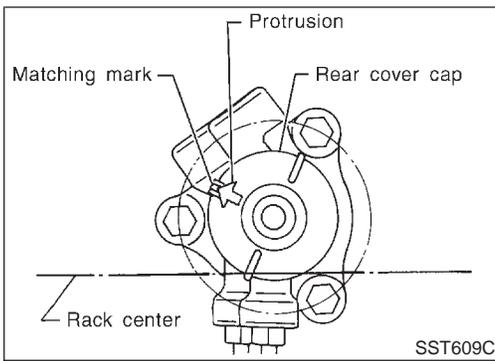
14. Ensure that the rack is centered. Install rear cover cap so that its protrusion is positioned as shown in figure.
