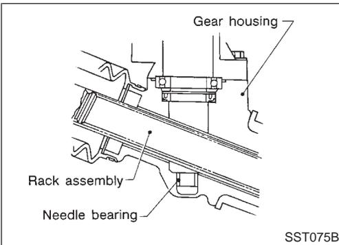
11. Apply a coat of multi-purpose grease to needle bearing roller and oil seal lip.
