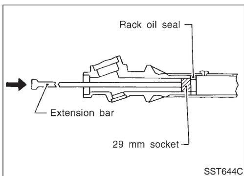
11. Remove rack bushing and rack oil seal using tape wrapped socket and extension bar.
