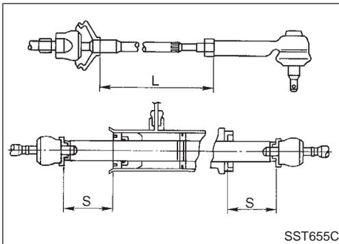
17. Tighten outer socket lock nut.
