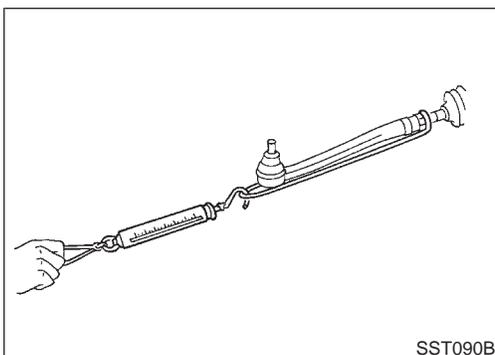
12. Check rack sliding force on vehicle as follows:
