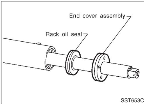
5. Insert rack oil seal and end cover assembly to rack. Then tighten end cover assembly.
