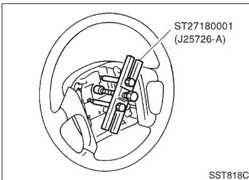
3. Remove steering wheel with Tool.
