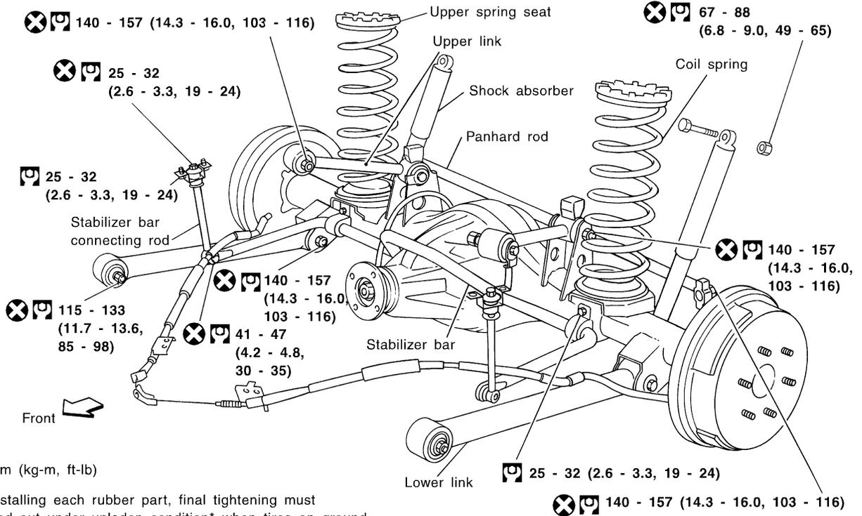
When installing each rubber part, final tightening must be carried out under unladen condition\* when tires on ground.
