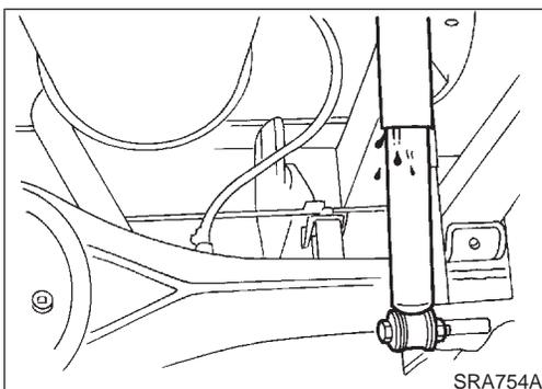
3. Check shock absorber for oil leakage and other damage.
