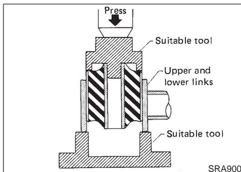
**When installing bushing, apply a coat of 1% soapy water to outer wall of bushing.**
