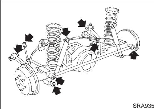
Final tightening for rubber parts requires to be carried out under unladen condition with tires on ground.
