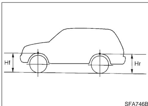
6. Check spring height from top of wheelarch to ground using the following procedure.
