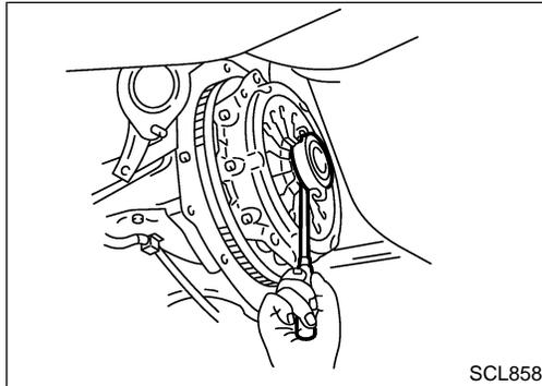
4. Using a flat-head screwdriver or the like, remove release bearing from clutch cover.
