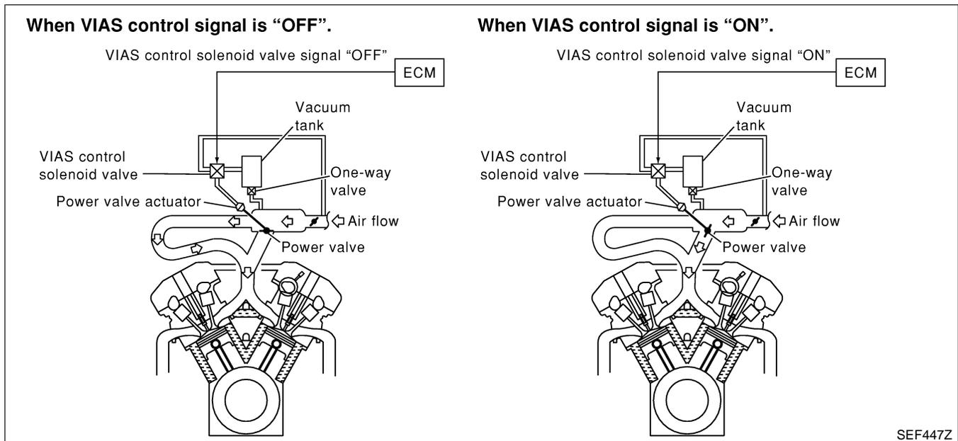
When the engine is running at low or medium speed, the power valve is fully closed. Under this condition, the effective suction port length is equivalent to the total length of the intake manifold collector's suction port including the intake valve. This long suction port provides increased air intake which results in improved suction efficiency and higher torque generation.
