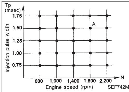
The ignition timing is controlled by the ECM to maintain the best air-fuel ratio for every running condition of the engine. The ignition timing data is stored in the ECM. This data forms the map shown.
