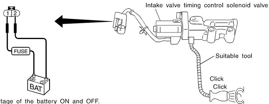
Turn the voltage of the battery ON and OFF.
