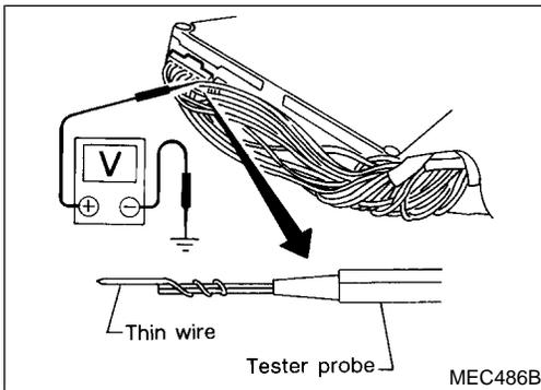
3. Perform all voltage measurements with the connector connected. Extend tester probe as shown to perform tests easily.
