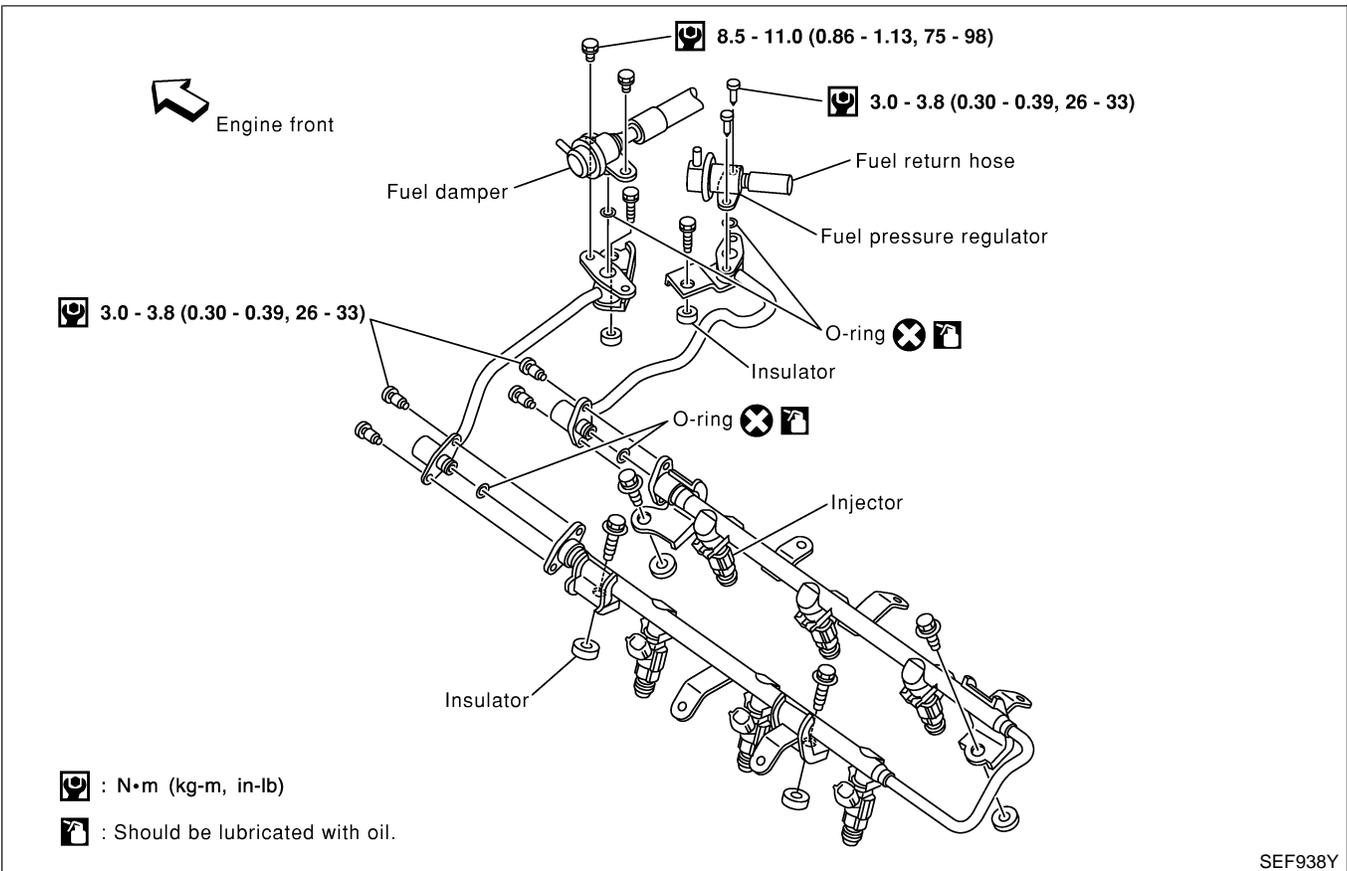
8. Align protrusions of fuel tubes with those of fuel injectors. Insert fuel injectors straight into fuel tubes.
