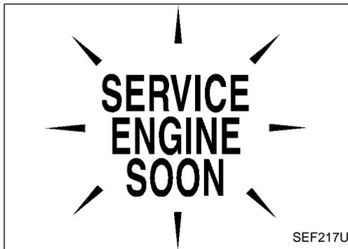
The MIL is located on the instrument panel.
