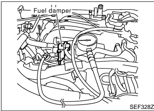
3. Install pressure gauge to the fuel pressure check adapter as shown in the figure.
