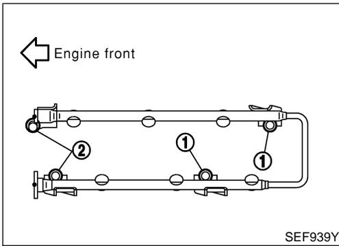
10. Tighten fuel tube assembly mounting nuts in numerical sequence (indicated in the figure at left) and in two stages.
