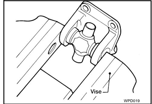
2. Select new snap rings that will provide the specified play in an axial direction of the journal, and install them. Refer to [PR-15, "Snap Ring"](#).
