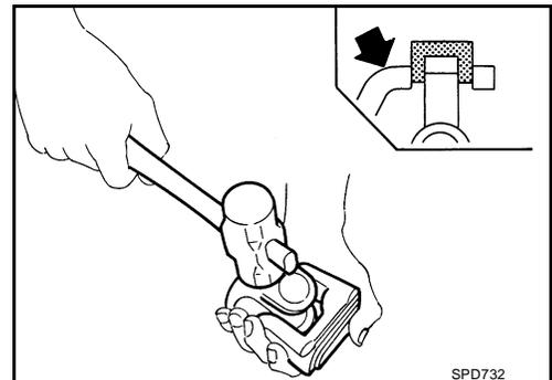
4. Push out and remove the remaining journal bearings at the opposite side by lightly tapping the flange yoke with a hammer, taking care not to damage the journal or flange yoke hole.
