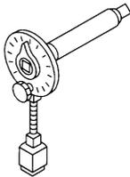
Tightening bolts for bearing cap, cylinder head, etc. in angle                                            |
