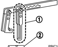
Disassembling valve mechanism<br>Part (1) is a component of KV10116200 (J-26336-A), but part (2) is not.                                                                                               | A<br>EM<br>C |
