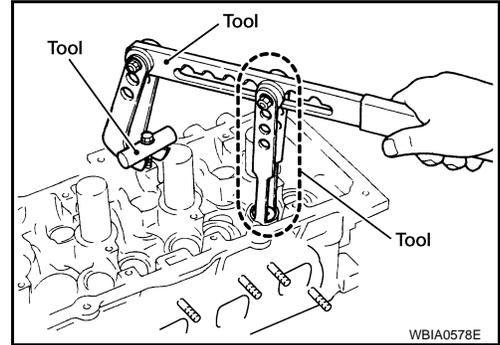
5. Remove valve oil seal using Tool.
