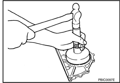
9. Install rear oil seal retainer.
