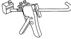
Pressing the tube of liquid gasket                                                                                 |
