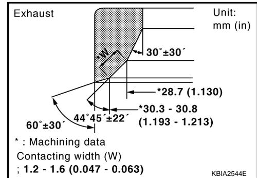
7. Check again for normal contact. Follow the "VALVE SEAT CONTACT" procedure.
