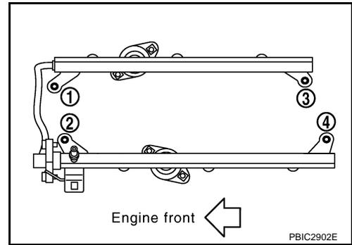
6. Tighten bolts which connects fuel tube (RH) and fuel tube (LH) with the specified torque.
