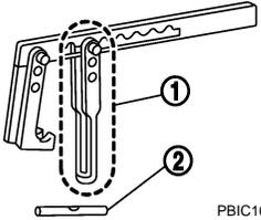
Disassembling valve mechanism<br>Part (1) is a component of KV10116200 (J-26336-A), but Part (2) is not so. |
