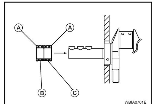
4. Install the timing chains and associated parts.
