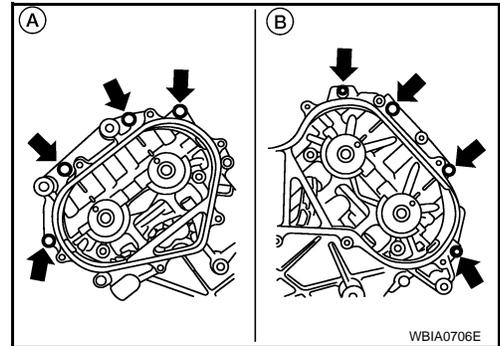
10. Remove RH (A) camshaft bracket bolts and LH (C) camshaft bracket bolts in the reverse of order shown to remove camshaft brackets.
