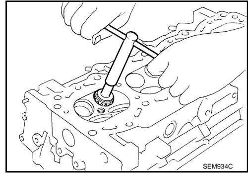
6. Grind to obtain the dimensions indicated as shown.
