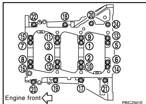
18. Remove lower cylinder block.
