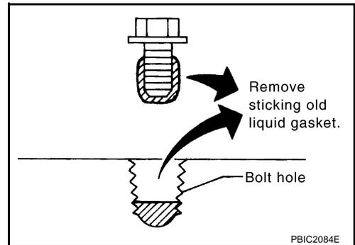
24. Use a scraper to remove all traces of old liquid gasket from water pump cover, chain tensioner cover and intake valve timing control covers.
