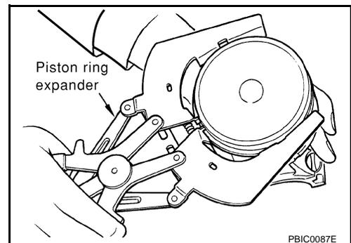
16. Remove piston from connecting rod as follows:
