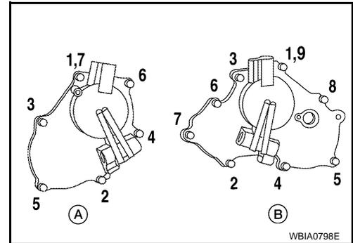
4. Paint alignment marks on the RH bank (A) timing chain links (C) and LH bank (B) timing chain links (D) and align with the camshaft sprocket alignment marks (E) and (F).
