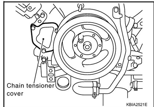
7. Remove the RH bank timing chain tensioner using the following steps.
