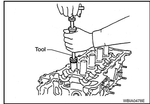
8. Replace the valve seat if necessary. Refer to [EM-212, "Inspection After Disassembly"](#).
