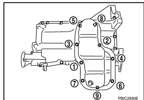
2. Install oil pan drain plug. Refer to [EM-36. "Removal and Installation"](#).
