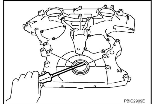
22. Use a scraper to remove all traces of old liquid gasket from front and rear timing chain cases and oil pan (upper), and liquid gasket mating surfaces.
