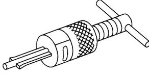
Removing crankshaft pilot bushing                                                                                                                                                                    | N<br>O       |
