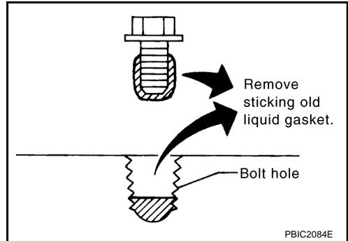
34. Use scraper to remove all traces of liquid gasket from water pump cover, chain tensioner cover and intake valve timing control covers.
