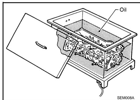
4. Provide valve seats cooled well with dry ice. Force fit valve seat into cylinder head.
