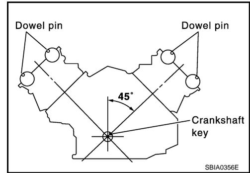
2. Install the camshaft sprockets.
