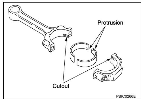
13. Install the piston and connecting rod assembly to the crankshaft using Tool.
