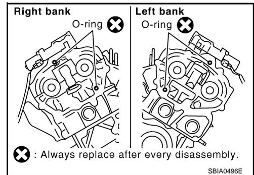
31. Remove O-rings from cylinder block.
