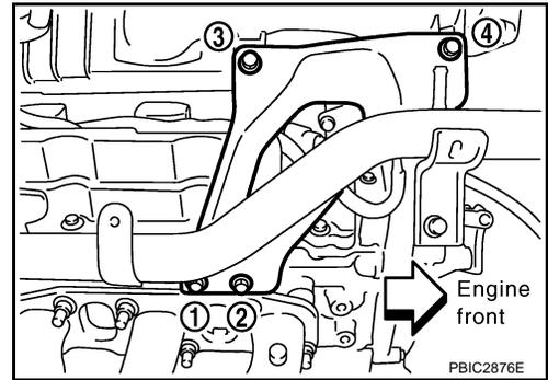
6. Disconnect EVAP hoses and harness connector from EVAP canister purge volume control solenoid valve.
