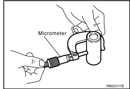
Connecting Rod Bushing Oil Clearance (Small End)
