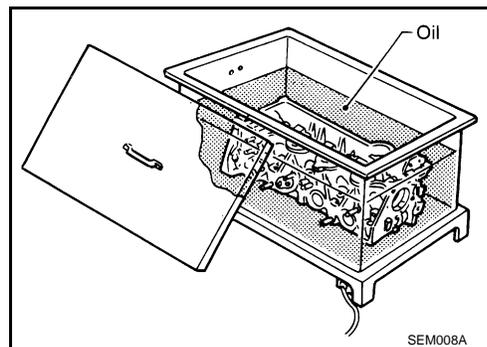
4. Cool the valve seats well with dry ice. Force fit the valve seat into the cylinder head.
