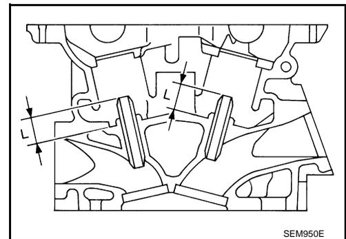
6. Apply reamer finish to valve guide using suitable reamer.
