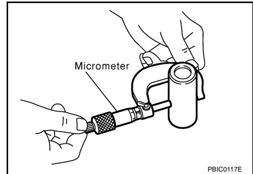
Piston to Piston Pin Oil Clearance
