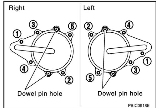
7. Install crankshaft pulley as follows:
