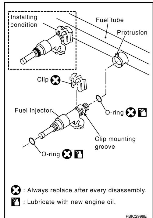
8. Disconnect fuel tube (RH) from fuel tube (LH).
