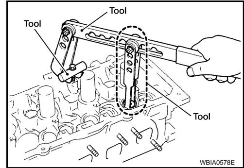
9. Install the valve lifters.
