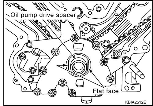
9. Remove the oil pump. Refer to [LU-30. "Removal and Installation"](#).
