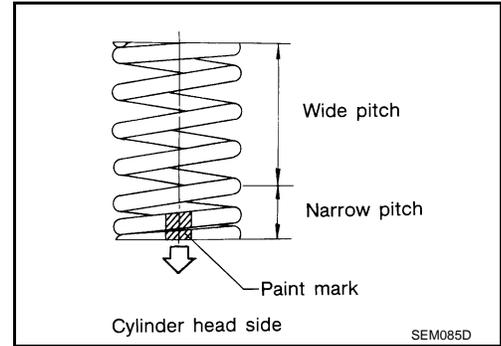
7. Install valve spring retainer.
