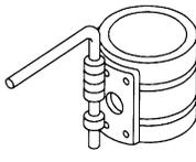
Installing piston assembly into cylinder bore                                                             |
