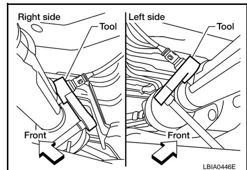
4. Remove center exhaust tube, main muffler and left front exhaust tube. Refer to [EX-5. "Removal and Installation"](#).
