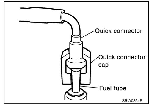
b. With the sleeve side of Tool facing quick connector, install Tool onto fuel tube.
