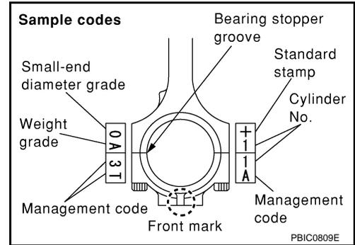
**Factory installed parts grading:**
