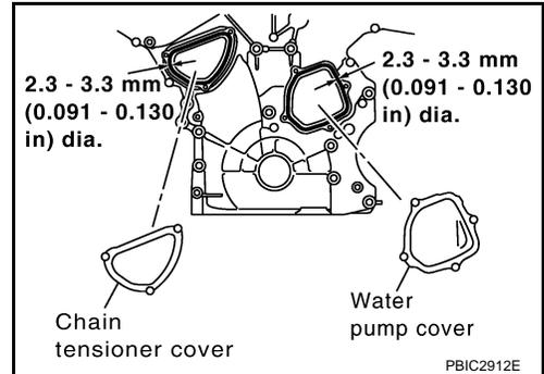
13. Install front timing chain case as follows:
