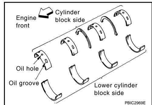
5. Install crankshaft to cylinder block.
