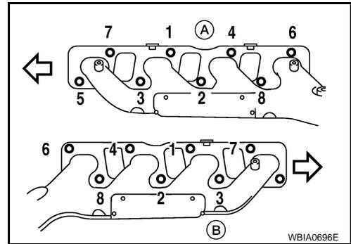
11. Remove the exhaust manifold (RH) (B) following the steps below.
