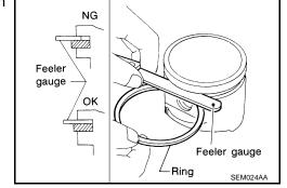
• If the measured value exceeds the limit, replace piston ring, and measure again. If it still exceeds the limit, replace piston also.
