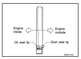
Press-fit until the front oil seal is level with the front cover using suitable tool.
