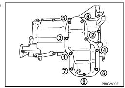
Insert Tool between the oil pan (lower) and the oil pan (upper).
