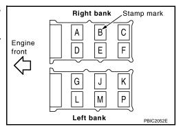
Apply liquid gasket to mating surface of camshaft bracket (No. 1) as shown on right and left banks.
