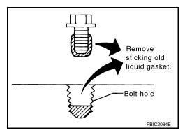
34. Use scraper to remove all traces of liquid gasket from water pump cover, chain tensioner cover and intake valve timing control covers.
