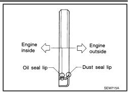
Press-fit the rear oil seal using suitable tool.
