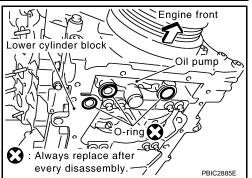
Apply a continuous bead of liquid gasket using Tool to the lower cylinder block mating surfaces of oil pan (upper) as shown.
