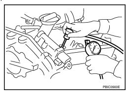
Use compression gauge whose pick up end inserted to spark plug hole is smaller than 20 mm (0.79 in) in diameter. Otherwise, it may be caught by cylinder head during removal.
