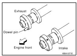
Follow your identification marks made during removal, or follow the identification marks that are present on new camshafts for proper placement and direction.
