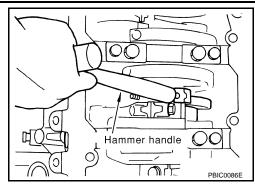
8. Remove connecting rod bearings.
