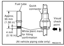
• Insert fuel tube into quick connector until top spool is completely inside quick connector, and 2nd level spool exposes right below quick connector on engine side.
