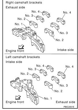
Install camshaft brackets (No. 2 to 4) aligning the stamp marks as shown.
