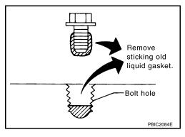
23. Use a scraper to remove all traces of old liquid gasket from water pump cover, chain tensioner cover and intake valve timing control covers.
