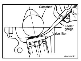
8. Turn the crankshaft pulley clockwise 270° from the position of No. 1 cylinder compression TDC to obtain No. 3 cylinder compression TDC.
