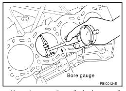
• If measured value exceeds the repair limit, or if there are scratches and/or seizure on the cylinder inner wall, hone or bore the inner wall.
