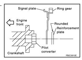
• Tighten the drive plate bolts in a diagonal pattern in two steps. Refer to <u>EM-108</u>, "<u>Disassembly and Assembly</u>".
