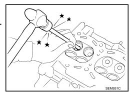
3. Ream the cylinder head valve guide hole using suitable tool.
