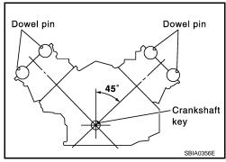
Install the camshaft sprockets.
