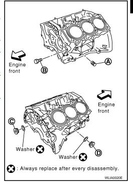
Tighten each plug as specified below.
