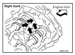
Use feeler gauge, measure the clearance between valve lifter and camshaft.
