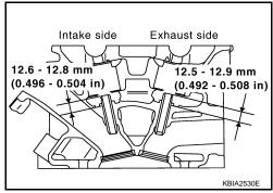
6. Ream the cylinder head valve guide using suitable tool.
