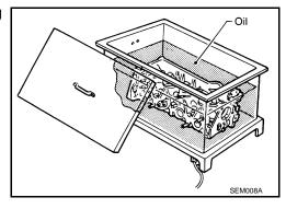
4. Provide valve seats cooled well with dry ice. Force fit valve seat into cylinder head.
