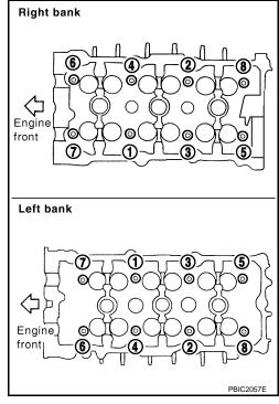
Measure the tightening angle using Tool.
