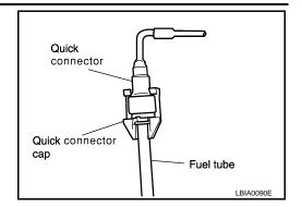
b. With the sleeve side of Tool facing quick connector, install Tool onto fuel tube.
