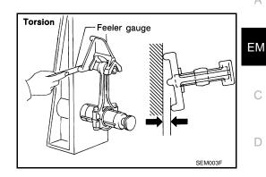
If measurement exceeds the limit, replace connecting rod assembly.
