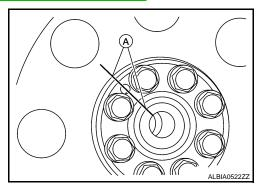
3. Lock the drive plate using Tool (A).
