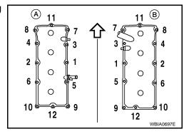
Apply liquid gasket to the joint part of the cylinder head and camshaft bracket following the steps below.
