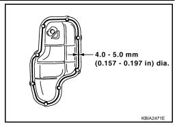
b. Tighten the oil pan (lower) bolts in numerical order as shown.
