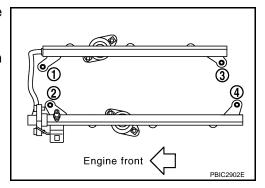
Remove bolts which connects fuel tube (RH) and fuel tube (LH).
