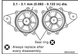
c. Install new collared O-rings in front timing chain case oil hole (left and right sides).
