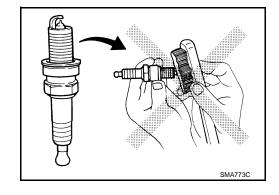
• If the spark plug tip is covered with carbon, a spark plug cleaner may be used.
