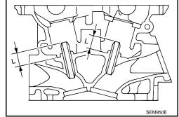
Apply reamer finish to valve guide using suitable tool.
