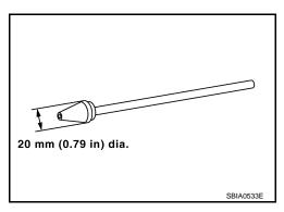
8. Turn ignition switch to "START" for cranking. When the gauge pointer stabilizes, read the compression pressure and engine rpm. Perform these steps to check each cylinder.
