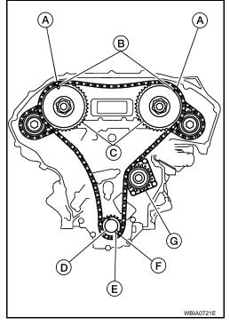
8. Install internal chain guide, slack guide and timing chain tensioner (primary).
