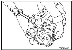
14. Remove connecting rod bearings from connecting rod and connecting rod bearing cap. **CAUTION:**
