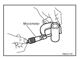
Connecting Rod Bushing Oil Clearance (Small End)
