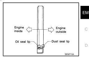
• Install new rear oil seal using Tool.
