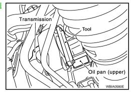
b. Loosen crankshaft pulley bolt and locate bolt seating surface as 10 mm (0.39 in) from its original position.
