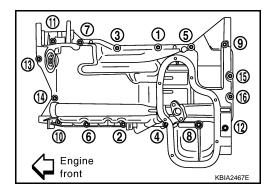
b. Remove the oil pan (upper) from the cylinder block by prying it at the points shown, using suitable tool.
