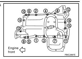
Insert Tool between oil pan (upper) and lower cylinder block.
