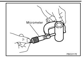
Connecting Rod Bushing Oil Clearance (Small End) (Connecting rod small end oil clearance) = (Inside diameter of connecting rod small end) – (Piston pin diameter)
