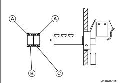
Install the timing chains and associated parts.
