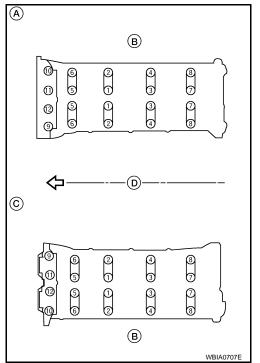
a. Tighten the RH (A) and LH (B) front cover bolts (4 for each bank) as shown to the specified torque.
