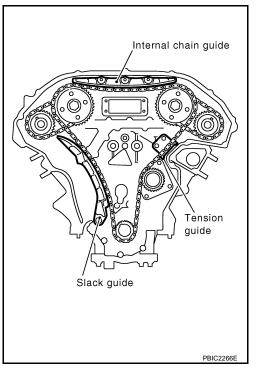
Remove timing chain (primary) and crankshaft sprocket.
