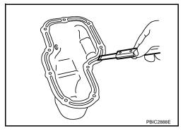
b. Apply a continuous bead of liquid gasket using Tool to the oil pan (lower) as shown.
