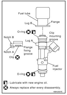
4. Install the fuel tube and fuel injector assembly to the intake manifold.
