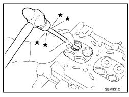
3. Ream cylinder head valve guide hole using suitable tool.
