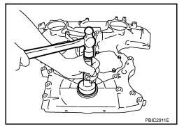
B. Install water pump cover and chain tensioner cover to front timing chain case, if removed.
