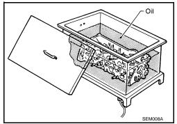
2. Remove the valve guide using suitable tool.
