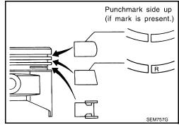
Position each ring with the gap as shown referring to the piston front mark.
