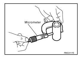
Piston to Piston Pin Oil Clearance
