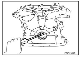
22. Use a scraper to remove all traces of old liquid gasket from front and rear timing chain cases and oil pan (upper), and liquid gasket mating surfaces.
