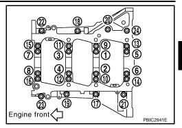
ii. Turn M10 bolts 90° clockwise in numerical order from No. 1 to 16 using Tool.
