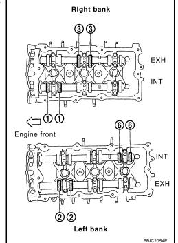
Rotate crankshaft by 240° clockwise (when viewed from engine front) to align No. 3 cylinder at TDC of its compression stroke.
