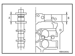
Camshaft Sprocket Runout
