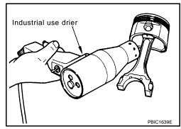
c. Push out piston pin with stick of outer diameter approximately 20 mm (0.79 in).
