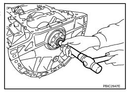
Press-fit pilot converter with its chamfer facing crankshaft as shown.
