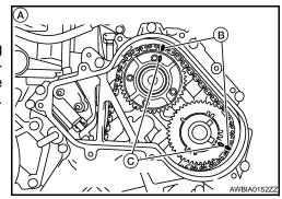
Install the intake VTC (A) and exhaust (B) side camshaft sprockets by selectively using the groove of the dowel pin according to the bank for the exhaust (B) side camshaft sprockets. (Common part used for both exhaust banks.)
