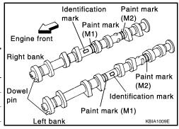
Install camshaft so that dowel pin hole and dowel pin on front end face are positioned as shown. (No. 1 cylinder TDC on its compression stroke)
