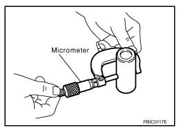
Piston to Piston Pin Clearance
