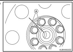
b. Lock the drive plate using Tool (A).
