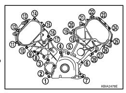
11. Install the Intake valve control solenoid valve cover (RH) (A) and Intake valve control solenoid valve cover (LH) (B) as follows:
