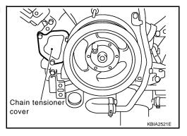
7. Remove the chain tensioner (RH) using the following steps.
