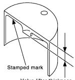
Valve lifter thickness SE
