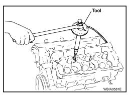
After installing cylinder head, measure distance between front end faces of cylinder block and cylinder head (left and right banks).
