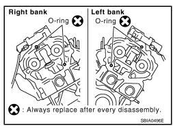
31. Remove O-rings from cylinder block.
