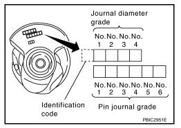
Select main bearing grade at the point where selected row and column meet in "Main Bearing Selection Table".
