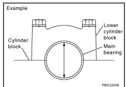
If the calculated value exceeds the limit, select proper main bearing according to main bearing inner diameter and crankshaft main journal diameter to obtain specified bearing oil clearance. Refer to EM-129, "How to Select Piston and Bearing".
