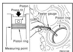
• If the measured value exceeds the limit, replace piston ring, and measure again.
