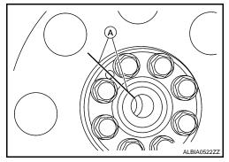
• Install the drive plate and the reinforcement plate in the direction as shown.
