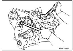
d. Pull stopper pins out from timing chain tensioners (secondary).
