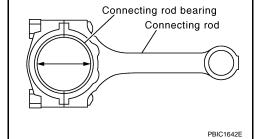
If the calculated value exceeds the limit, select proper connecting rod bearing according to connecting rod big end diameter and crankshaft pin journal diameter to obtain the specified bearing oil clearance. Refer to EM-129, "How to Select Piston and Bearing".
