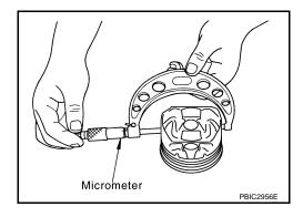
Piston to Cylinder Bore Clearance
