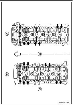
Measure valve clearance using suitable tool. Refer to <u>EM-250</u>, <u>"Standard and Limit"</u>.
