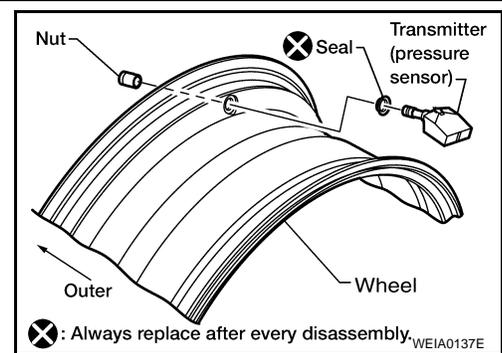
4. Place wheel on turntable of tire machine. Ensure that transmitter is 270 degrees from mounting/dismounting head.
