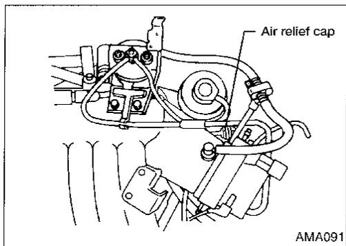
17. Remove heater pipe air relief cap.
