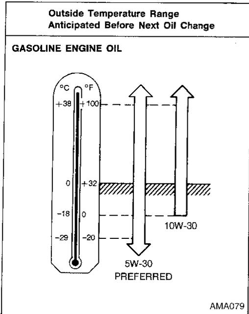
SAE 5W-30 viscosity oil is preferred for all temperatures. SAE 10W-30 viscosity may be used if the ambient temperature is above -18°C (0°F).
