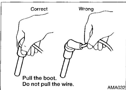
1. Disconnect ignition wires from spark plugs at boot. Do not pull on the wire.
