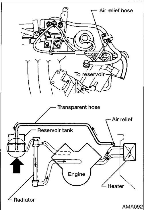
18. Install 1 meter (40") of 6 mm (0.24 in) I.D. heat resistant hose (clear if available, minimum temperature rating 105°C/ 220°F) to heater pipe air relief.
