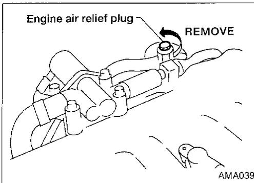
15. Remove engine air relief plug.
