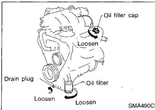
2. Remove drain plug and oil filler cap.
