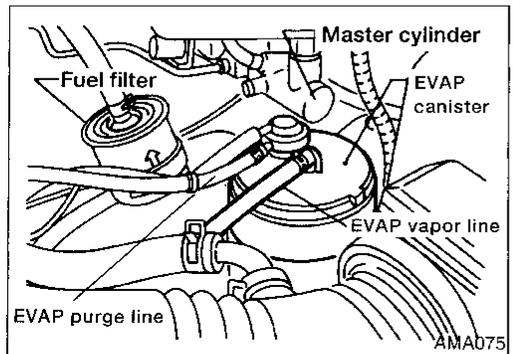
1. Visually inspect EVAP vapor purge lines for improper attachment, cracks, damage, loose connections, chafing and deterioration.
