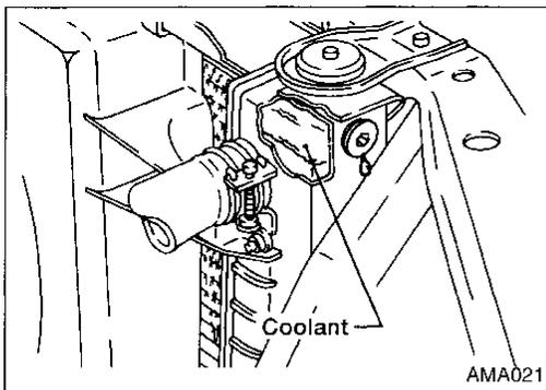
20. Slowly pour proper mixture of coolant into the radiator filler neck. Allow several minutes for air to escape.
